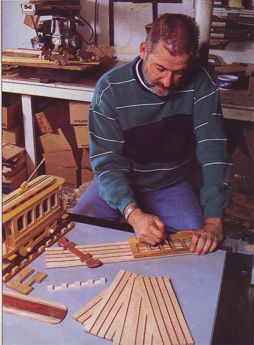
Hank uses templates to help him lay out the parts for a trolley car. With track, his trolley will bring $125.
