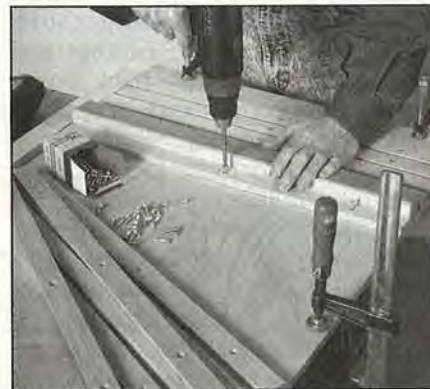
Glue and screw the maple mounting strips to the plywood back, using the spacing jig for consistent gaps.
