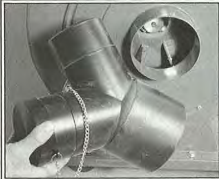
The Grizzly, Jet, Penn State DC2, and Woodmaster units have no physical barrier to the impeller-housing inlet.
