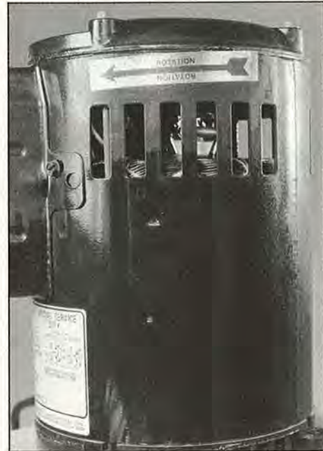
Totally enclosed, fan-cooled motors have a fan on the end of the motor and beneath a protective housing.
