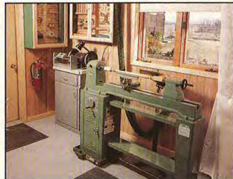
Below. The lathe parallels an end wall of the shop. Its mobile base allows you to swing it out for special turning tasks. Note the portable dust pickup behind the lathe and the turning-tool storage nearby.
