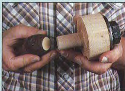
A dowel and an auxiliary faceplate provide a simple, effective way to mount tagua nuts for turning.
