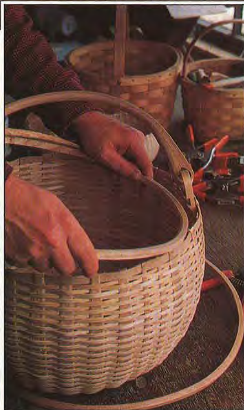
Above photos. Stephen seats the solid ash inner rim, and then adds an outer rim to protect the top. Next, with stout, flexible splints, he tightly lashes the rims together and to the weavers.
