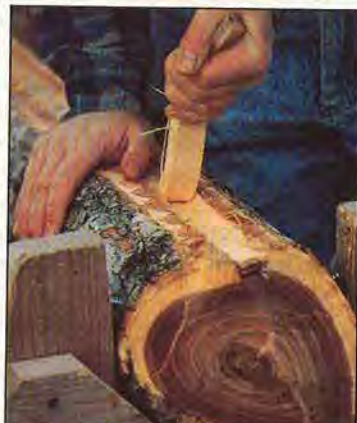
Before stripping off splints, the basketmaker marks their width at about 2" with incisions.
