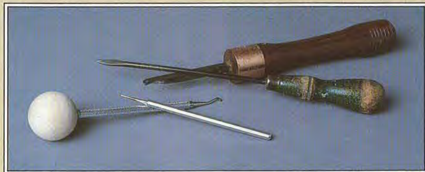
A practical assortment of tools for turning tagua nuts includes dental tools (note the ball-end handle added to one to give firm grip), an old screwdriver ground into a scraper, and a shop-made scraper.
