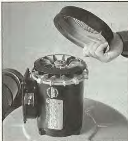
Totally enclosed, fan-cooled motors have a fan on the end of the motor and beneath a protective housing.
