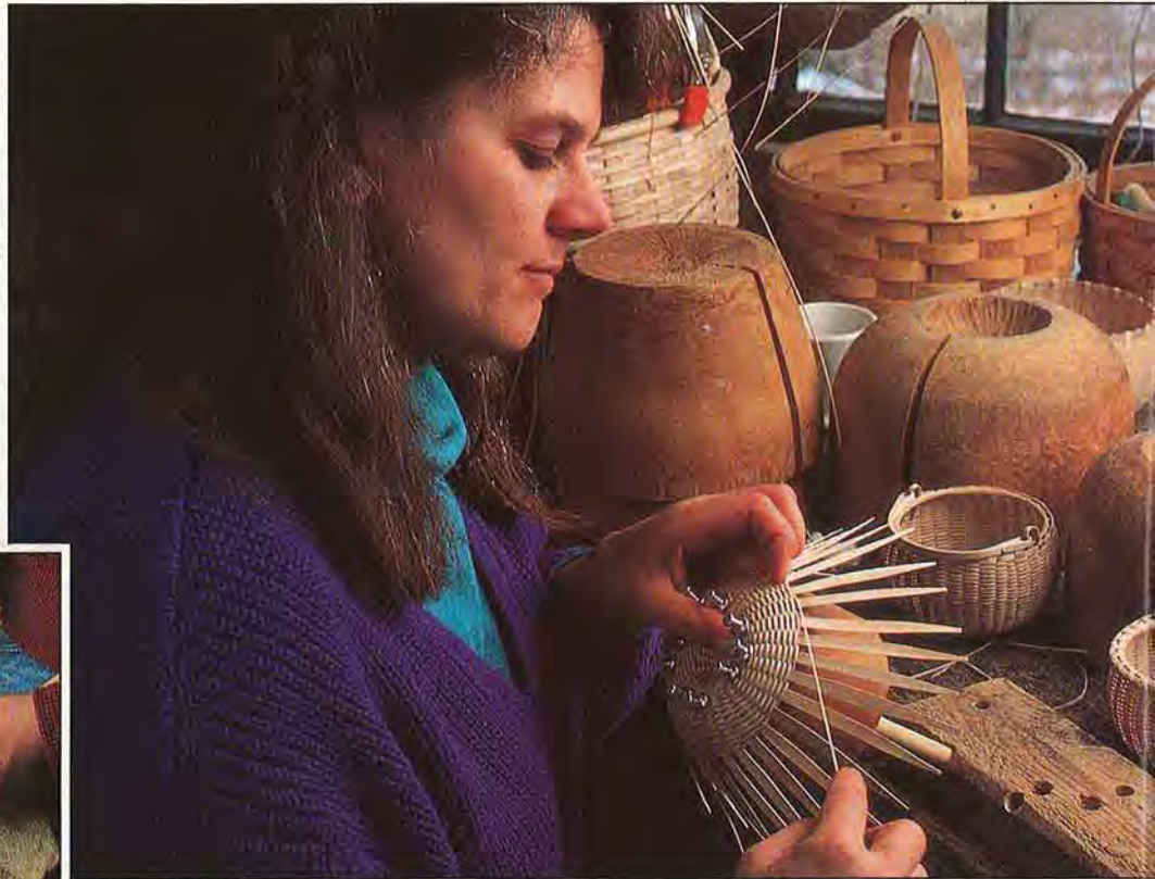
Left. Stephen scrapes ash splints clean so they'll weave more easily, but the process adds luster, too. Above. With the uprights in place on the mold, Tammy weaves a small basket. Each round Zeh basket begins with a kick-up bottom to distribute the load.
