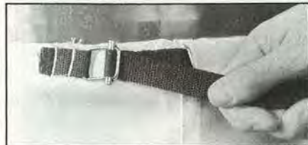
The nylon straps on the Grizzly G1029 work conveniently, but need to be snugged up from time to time.
