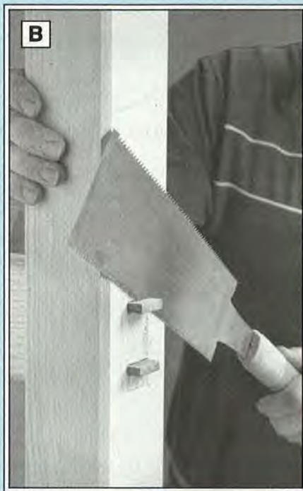
B Tap the hardwood wedges into the notches. After the glue dries, trim the wedges flush with the legs.
