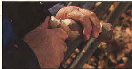
3. Use the paring cut for smoothing the surface or whittling details. Let the workpiece shield your thumb.
