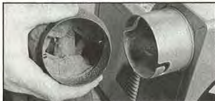
Two locking pins hold the single bag of the Makita 410 securely in place, and help make for quick disconnects.
