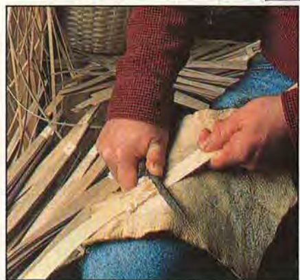
Left. Stephen scrapes ash splints clean so they'll weave more easily, but the process adds luster, too. Above. With the uprights in place on the mold, Tammy weaves a small basket. Each round Zeh basket begins with a kick-up bottom to distribute the load.
