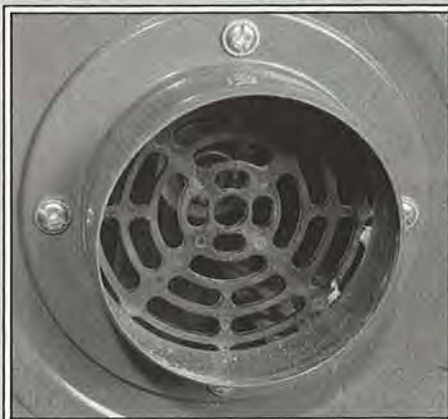
The Penn State DC3 has a grate covering the impeller-housing inlet, but it clogs when handling debris larger than fine sanding dust. You can easily remove the grate, but doing so leaves no protection over the opening.
