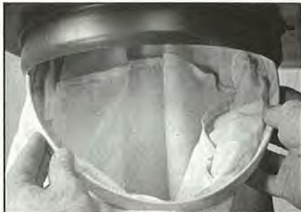
A sewn-in hoop on the Sears 29978 waste bag forms a good seal and helps you quickly change the bag.
