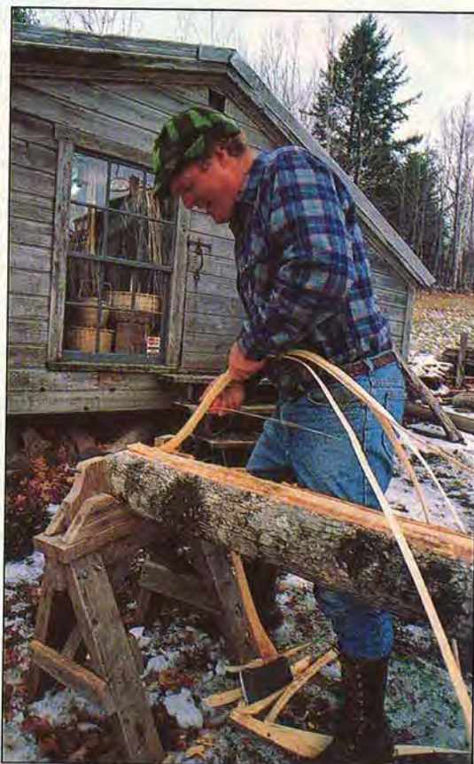
The growth rings peel off 5–6 at a time as separate splints about 1/8" to 1/32" thick. Stephen will use both sapwood and heartwood.
