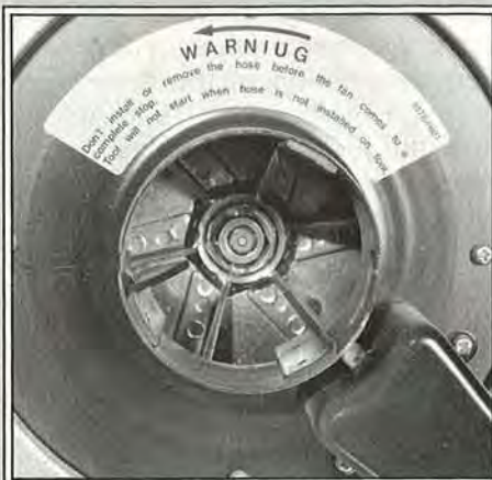
The Makita 410 has a safety switch which turns the machine off when you disconnect the pickup hose.
