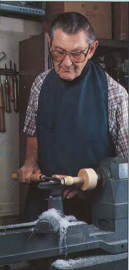
Chuck Luebbers shapes a vegetable ivory vessel. He runs the lathe at 2,000 rpm when turning tagua nuts.
