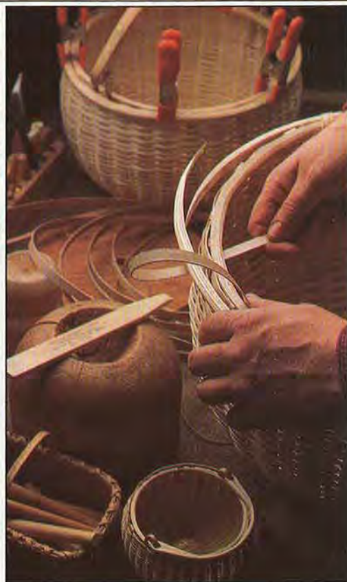
Above photos. Stephen seats the solid ash inner rim, and then adds an outer rim to protect the top. Next, with stout, flexible splints, he tightly lashes the rims together and to the weavers.
