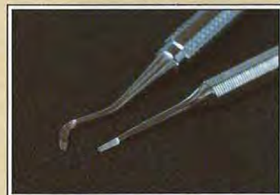
Reground dental scalers are just the ticket for reaching inside tagua turnings. Single-ended ones are best.
