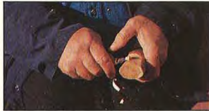
1. Pare away wood quickly for roughing with this basic whittling stroke.
