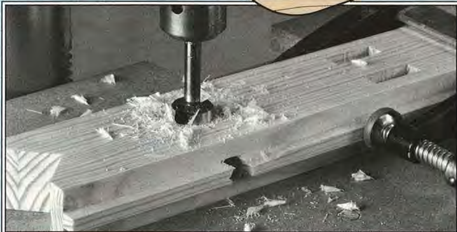
With the stool legs clamped together and the adjustment-dowel holes aligned, bore a 1" hole through both legs to form the finger recesses.
