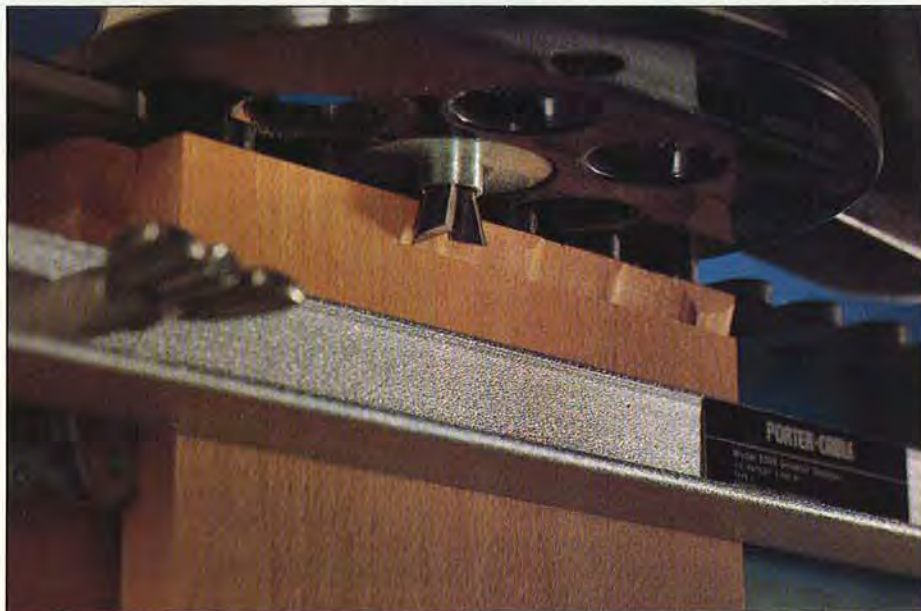
Before cutting the dovetails, make a skimming cut to help prevent grain tearout. Make light cuts, but hold the router firmly to maintain control.
