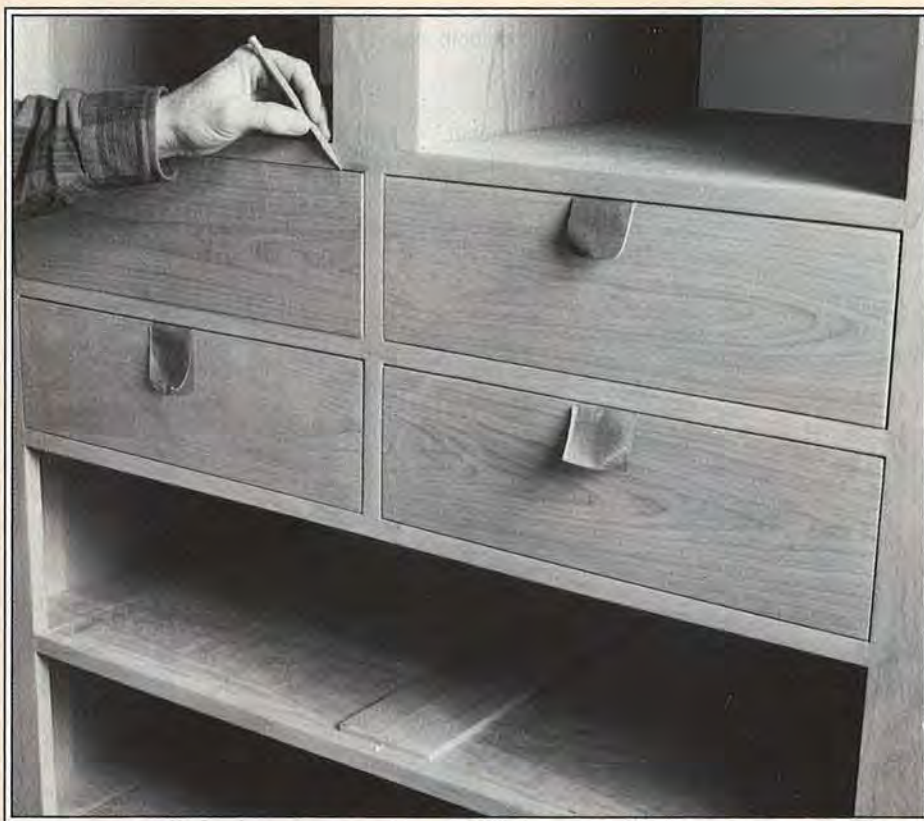
If the front of a drawer protrudes beyond the face frame, mark the protrusion. Then, plane and sand it flush with the face frame.
