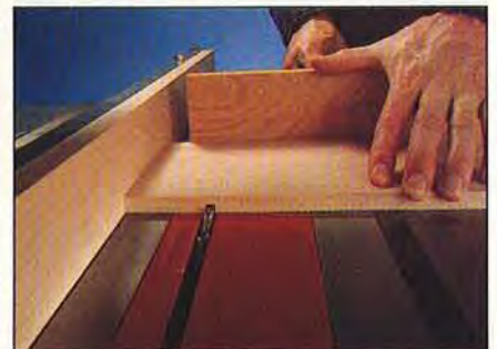
Use your tablesaw's fence as a stop when cutting dados into the drawer sides for holding the drawer back.
