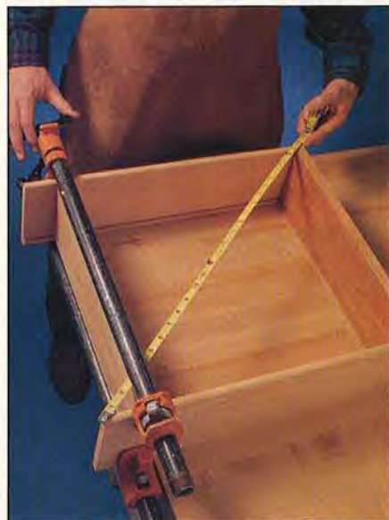
Reposition your clamps slightly to make the drawer square.
