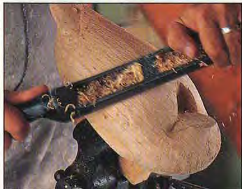
The notched platform on the decoy body will accept a resting head, one of many head types Grayson uses in a rig.
