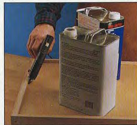
A few beads of hotmelt glue will hold the bottom in place and prevent it from rattling around in its groove.
