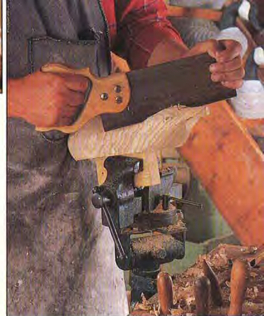
The sharp definition of gathered wing feathers on the decoy's back requires a cut with a backsaw.
