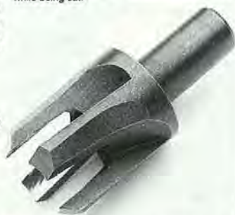
TAPERED Sides are smooth since they are shaved to size while being cut. STANDARD Sides are rough because of fiber tearing while being cut.
