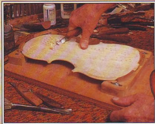
Spruce tops can be hand-carved to thickness, such as Bill is doing here, but hard maple requires machine tools.
