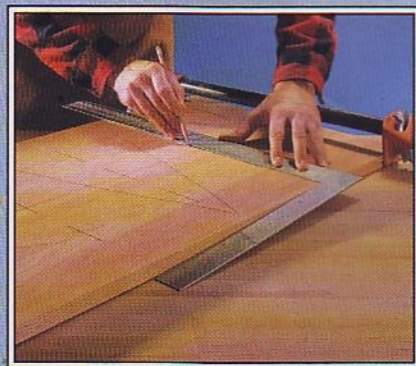
A framing square helps you accurately mark the biscuit positions along the joint lines of a dry-clamped panel.
