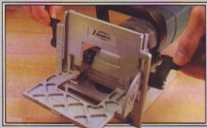
You can change the height and angle of the fence on the Virutex AB-11 in seconds by flipping two levers.
