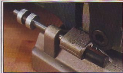
Most biscuit joiners have a three-stop depth setting similar to this one on the Freud JS100.
