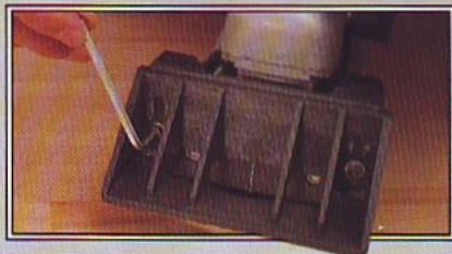
To reposition the fence on the Skil 1605:02 you have to loosen two screws with an allen wrench.
