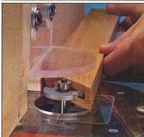
A freehand guard helps you rout curved workpieces.
