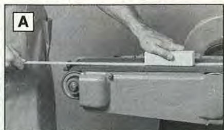
Using a block for uniform pressure, sand the faces of the uprights and weavers to remove saw and burn marks.
