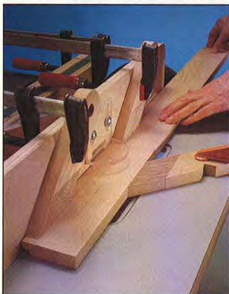
Feather boards ensure safe, consistent cuts on long workpieces.
