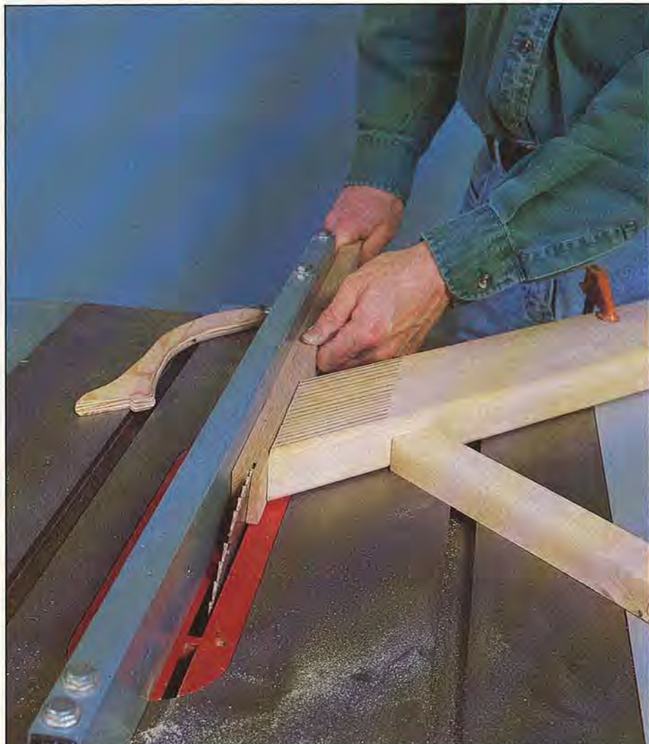
Use a feather board and feather-board support clamped to the saw table to support the stock when bevel-ripping the oak trim pieces.
