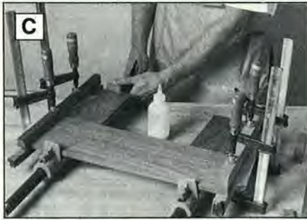
C Glue, spline, and clamp the lid together in two steps to help ensure a flat lid.
