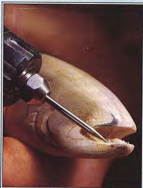
Carve a groove around the lower inside jaw with a small spherical cutter. Undercut the tongue on the front and sides so that it looks like it's flicking when you view the fish from the side.
