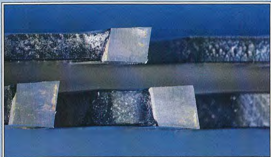
In this top-view photo, the narrow teeth of a thin-kerf blade (top) distinguish it from a full-kerf blade (bottom).
