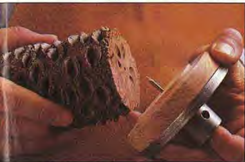
A nail through a hole in the center of the auxiliary faceplate acts as temporary index for mounting the pod.
