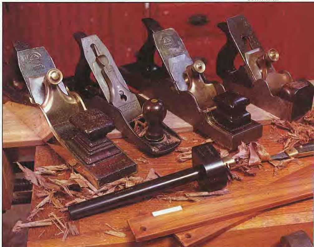
Each bench plane has a purpose and is used in order when straightening a board. Left to right: scrub plane, try plane, fore plane, and smoothing plane.
