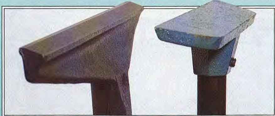
We prefer tool rests like the Sears version ( left ) that has a long, flat, smoothly ground top edge and a finger groove just below this edge for guiding the tool. The Reliant tool rest ( right ) lacks these qualities.
