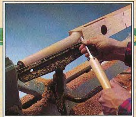
Use a gouge to turn the cove where the leg taper meets the unturned portion.
