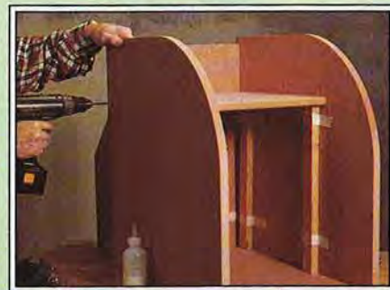
Tape four supports in place to hold the shelf in position when screwing it in place in the box.
