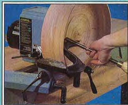
Pivoting headstocks make outboard turning a snap. Above is the Delta 46-700 with an optional tool-rest base extension and a curved tool rest.
