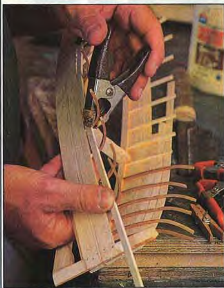
Top. To shape poplar into ribs, Steve tacks them to a master form. The strips were first soaked in ammonia for a week. Above. The outward-flaring ribs push against the secured planks, holding them in place until the glue dries.
