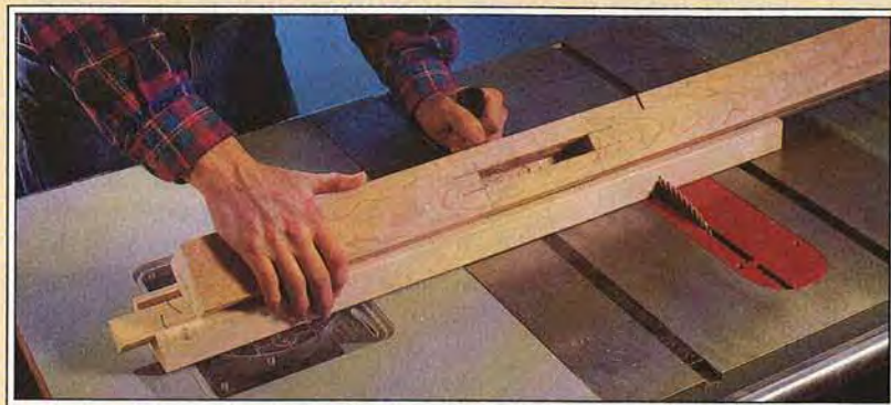
Cut kerfs to act as reference marks and minimize chipping when turning.
