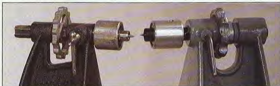
Extra dollars buy you a better fit and finish on similar-looking tailstocks from AMT ( left ) and Williams & Hussey.
