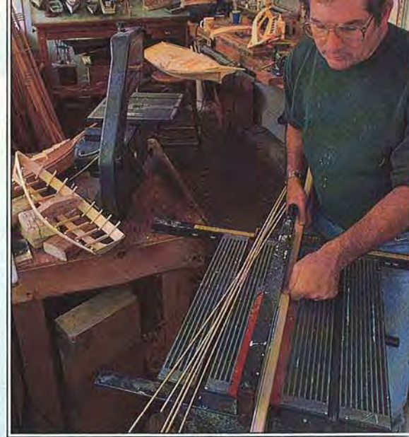
In his sunlit shop on an enclosed porch, Steve rips 3/32"-thick pieces of Idaho white pine for planking. His benchtop saw is sized for the work.
