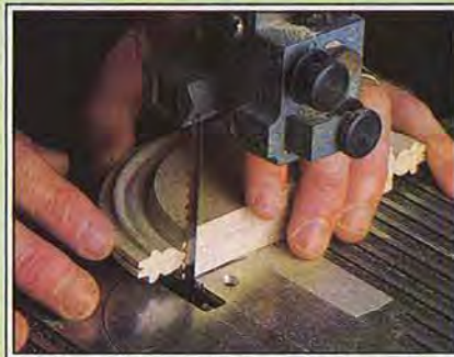
Turning a "hoop," Glenn's tiny gouge cuts the profile of a gingerbread cookie in yellow poplar. At the bandsaw, he saws off the profiled hoop and slices 550 tiny gingerbread-man shapes from it.
