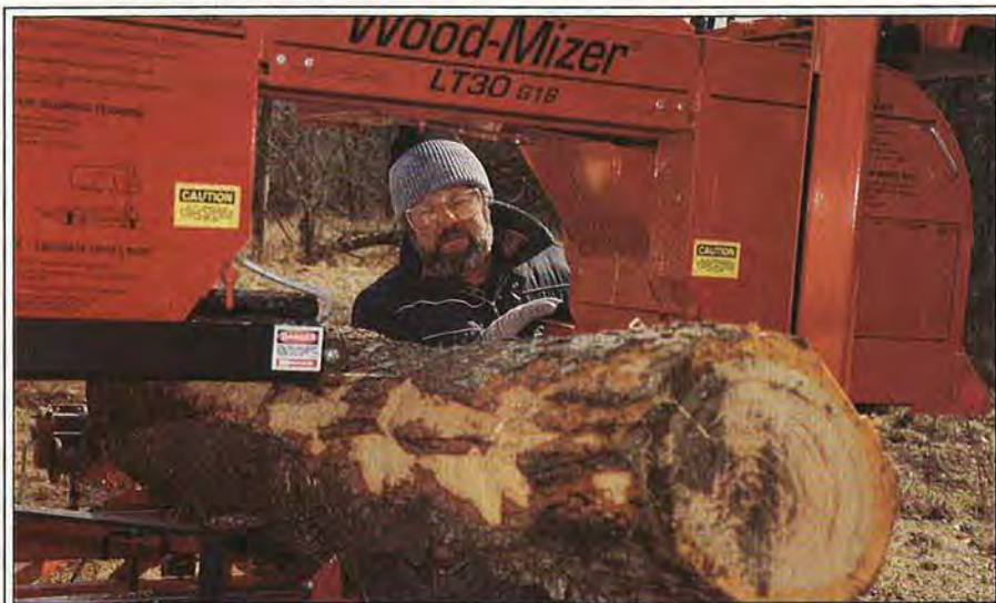
With four saw passes, Jim Downing will shape this log into a square cant. Then, he can start sawing for grade from the best, defect-free side.
