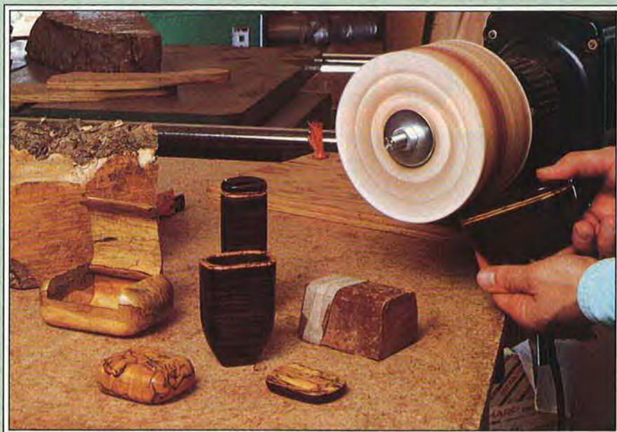
▲ The six-ply cotton buffing wheel on Jerry's bench grinder required a long custom spindle. For a high gloss on the finish, he charges the wheel with tripoli, a polishing compound, then follows with carnuaba wax.
