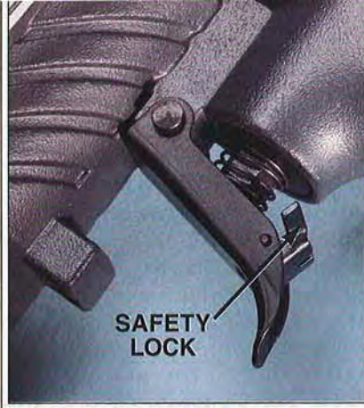
▲ The Sears 18300 air-powered stapler has a safety lock that works like the trigger lock on a firearm.
