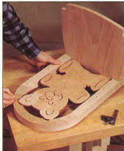
Position the bear cutout on the assembled backrest, and mark the slot locations as shown.
