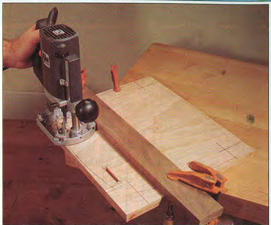
Rout a pair of \frac{1}{4} " slots \frac{1}{2} " deep in the seat blank to house the bottom of the bear's feet. For photo clarity we moved the model's right hand away from the router.
