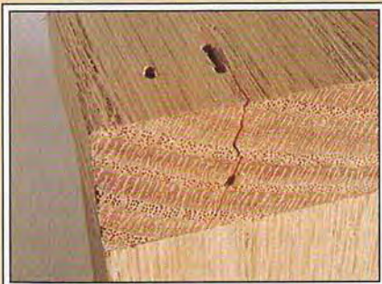
Staples have greater holding power, but leave larger holes, and tend to split hardwoods more so than brads.
