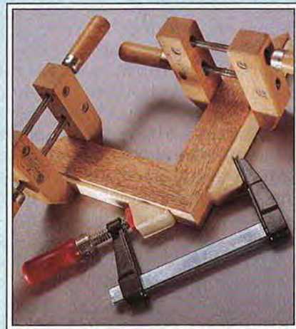
Corner clamp blocks like those illustrated on the next page help your clamps snugly hold miters together.
