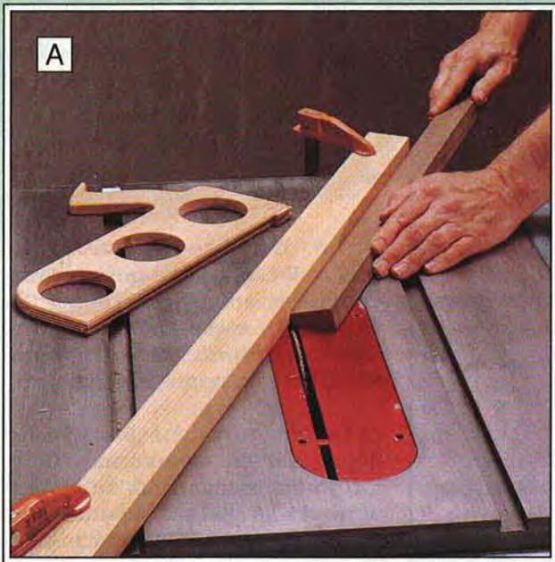
A Clamp a straightedge in place, raise the blade \frac{1}{16} " above the saw surface, and cut a cove in the frame stock.
