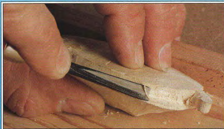
Carve the overhanging edge of the shell with a V-tool.
