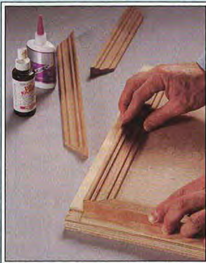
With instant glue, accelerator, and a right-angle gluing jig, you can join mitered frames in seconds.
