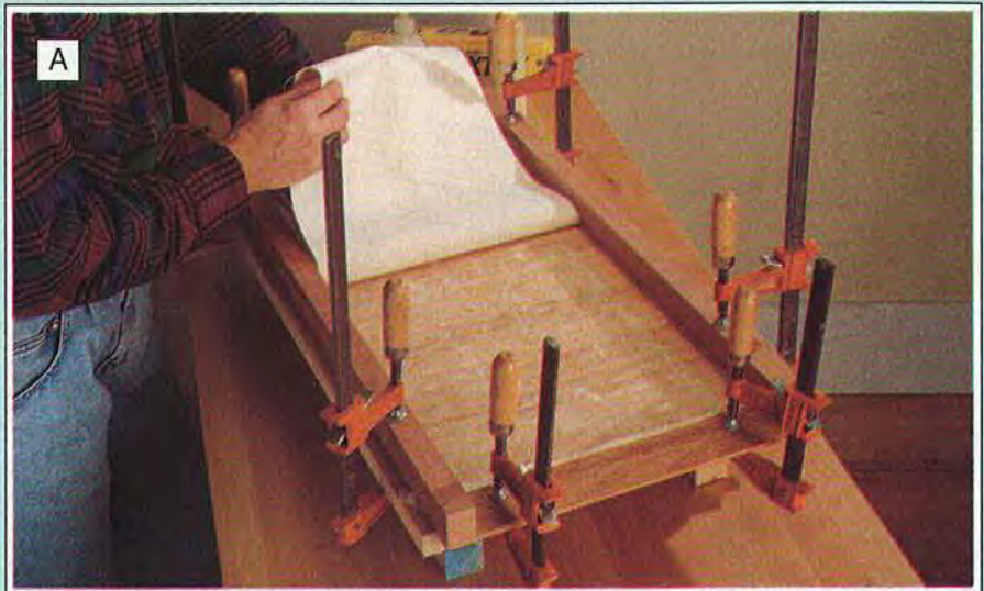
Clamp the oak strips to the clamping jig good face down. Spread glue between the clamping blocks, and adhere a piece of lightweight canvas to the strips.
