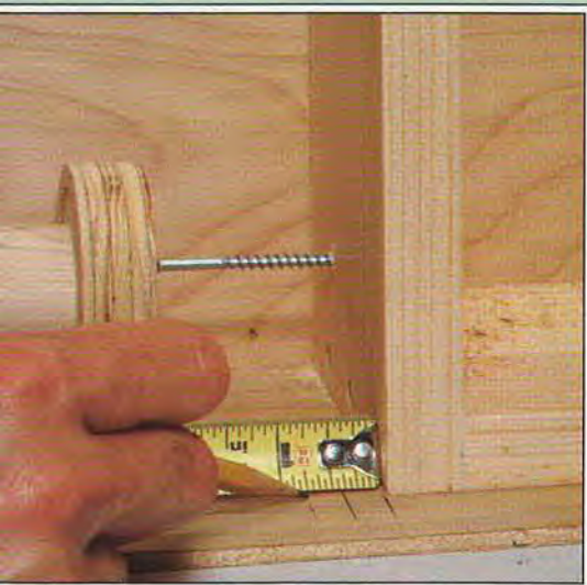
Mark the bead spacing on the base of the router-turning fence.
