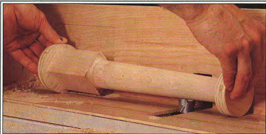
With discs of different sizes you can create tapered workpieces.
