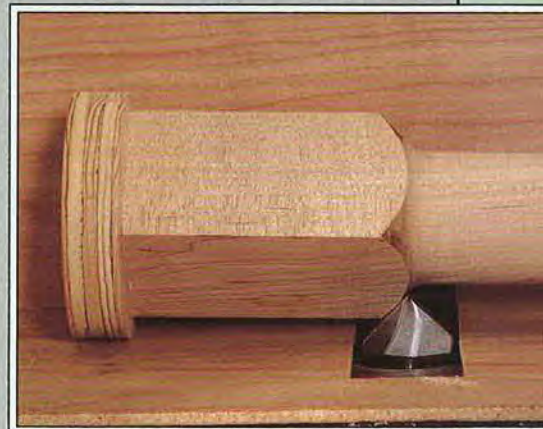
V-grooving bits cut a smooth transition from the shank to the shoulder
