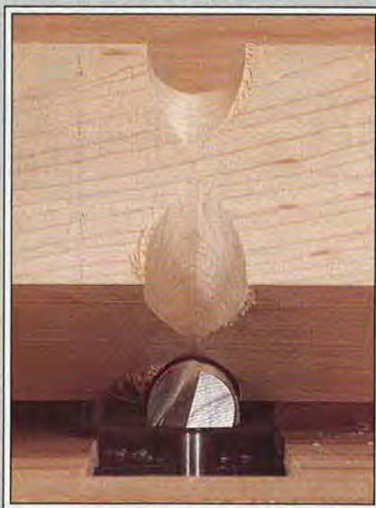
A round-nose bit cuts the shoulder that separates the shank from the tapered portion. Make the cut in several light passes to prevent splintering.
