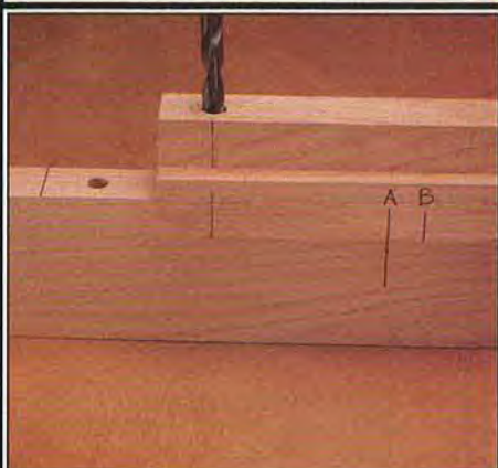
5. Top : Bore the center dowel hole on the edge of the lock rail.
