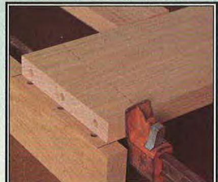
7. Use the marks on the stiles to keep the first glue-up square.
