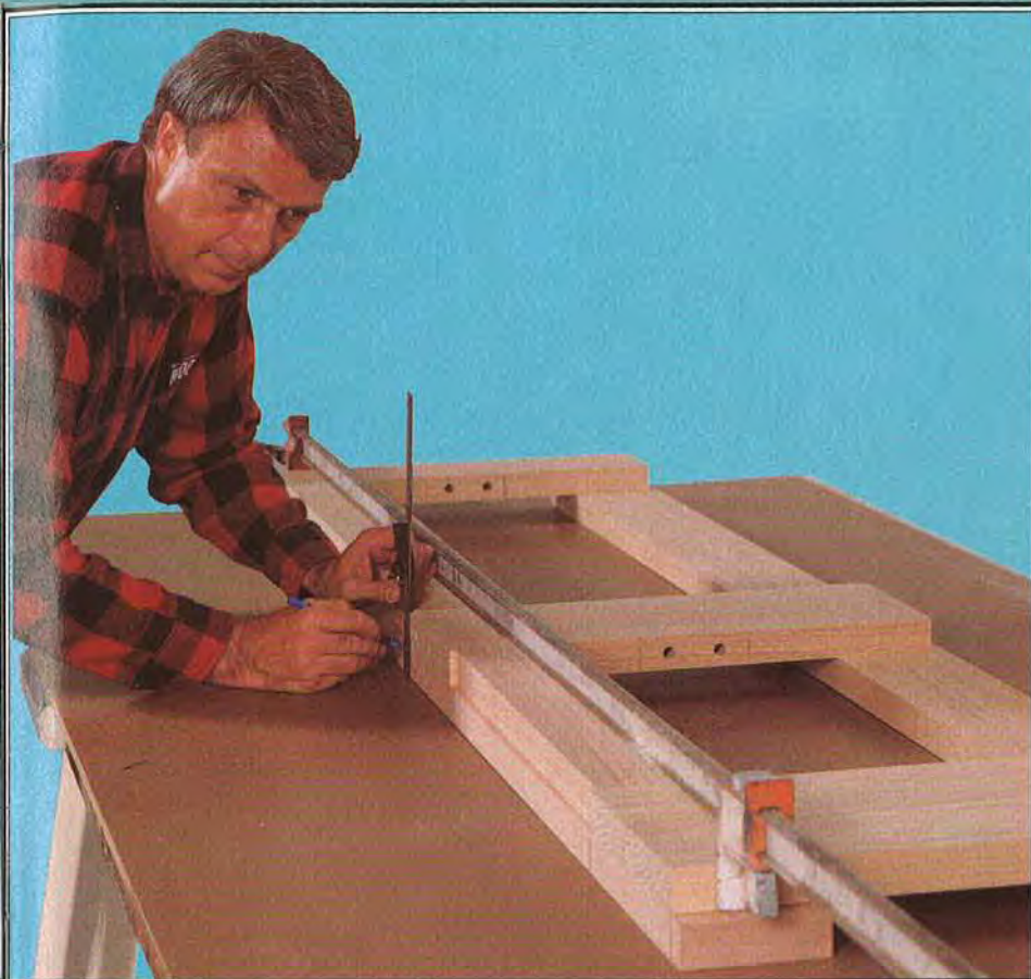
4. Mark the position of the rails on the stiles
