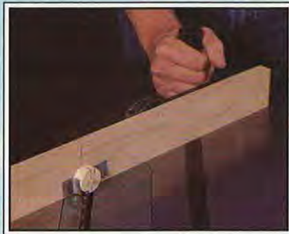
Attach a wood extension to your miter gauge, and cut a pair of angled notches in the propeller hub.
