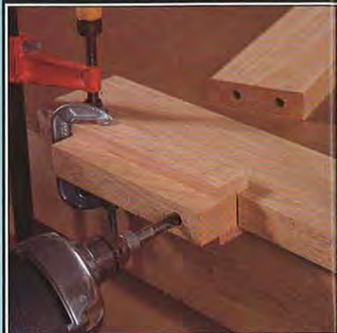
2. Top: Bore dowel holes in the end grain of the mullions.
