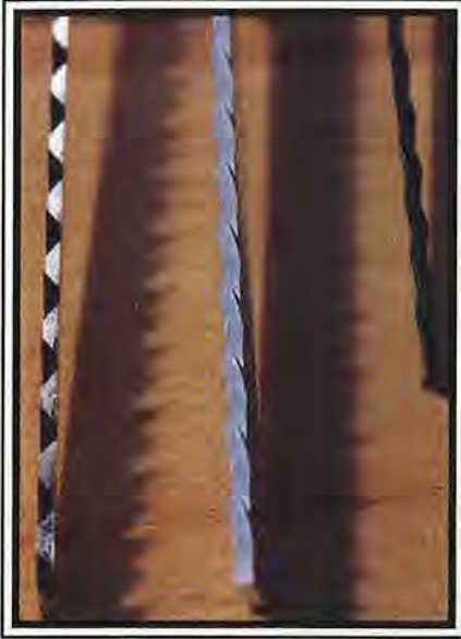
Tooth set affects the quality and speed of your cut. Flat-set blades (left) cut smoothly. Side-set blades (middle) are best used for rough cuts or speed work. Wavy-set blades (right) work well on metal, plastics, and ceramics
