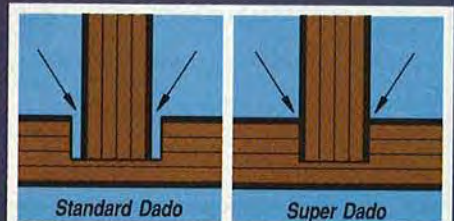
Exclusive 3/32" Chipper lets you perfectly adjust the width of the cut for today's undersized plywood.
