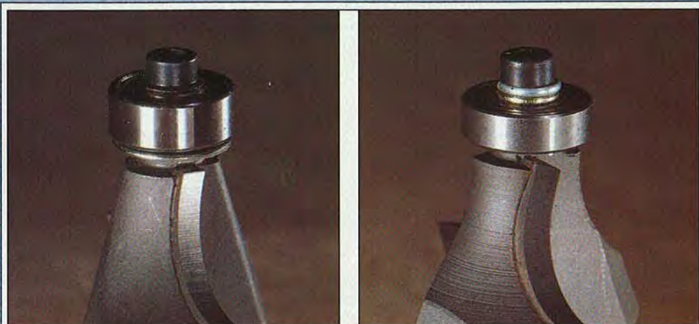
The Bosch bit, left, offers a dust shield and a relief grind under the bearing. The Grizzly bit, right, typical of the Taiwanese bits tested, keeps costs low by offering neither.
