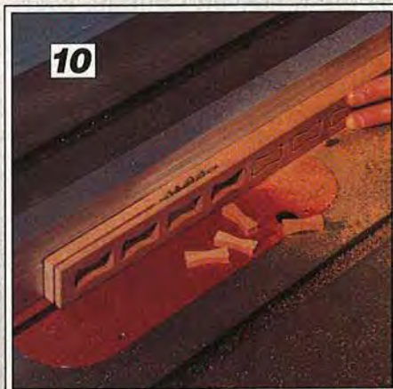
Cut the 1/4"-thick splines (bow ties) on the outboard side of your table saw blade.
