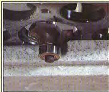
Carbide-tipped router bits cut Corian cleanly. Routed edges usually require no further finishing.
