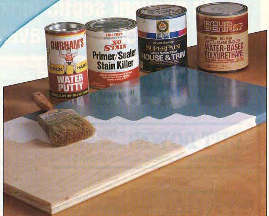
For a glass-smooth paint job on plywood, sand carefully and follow with putty, primer, paint, and a top coat of polyurethane.
