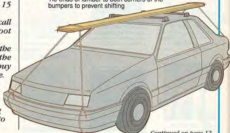
Tie ends of lumber to both corners of the bumpers to prevent shifting
