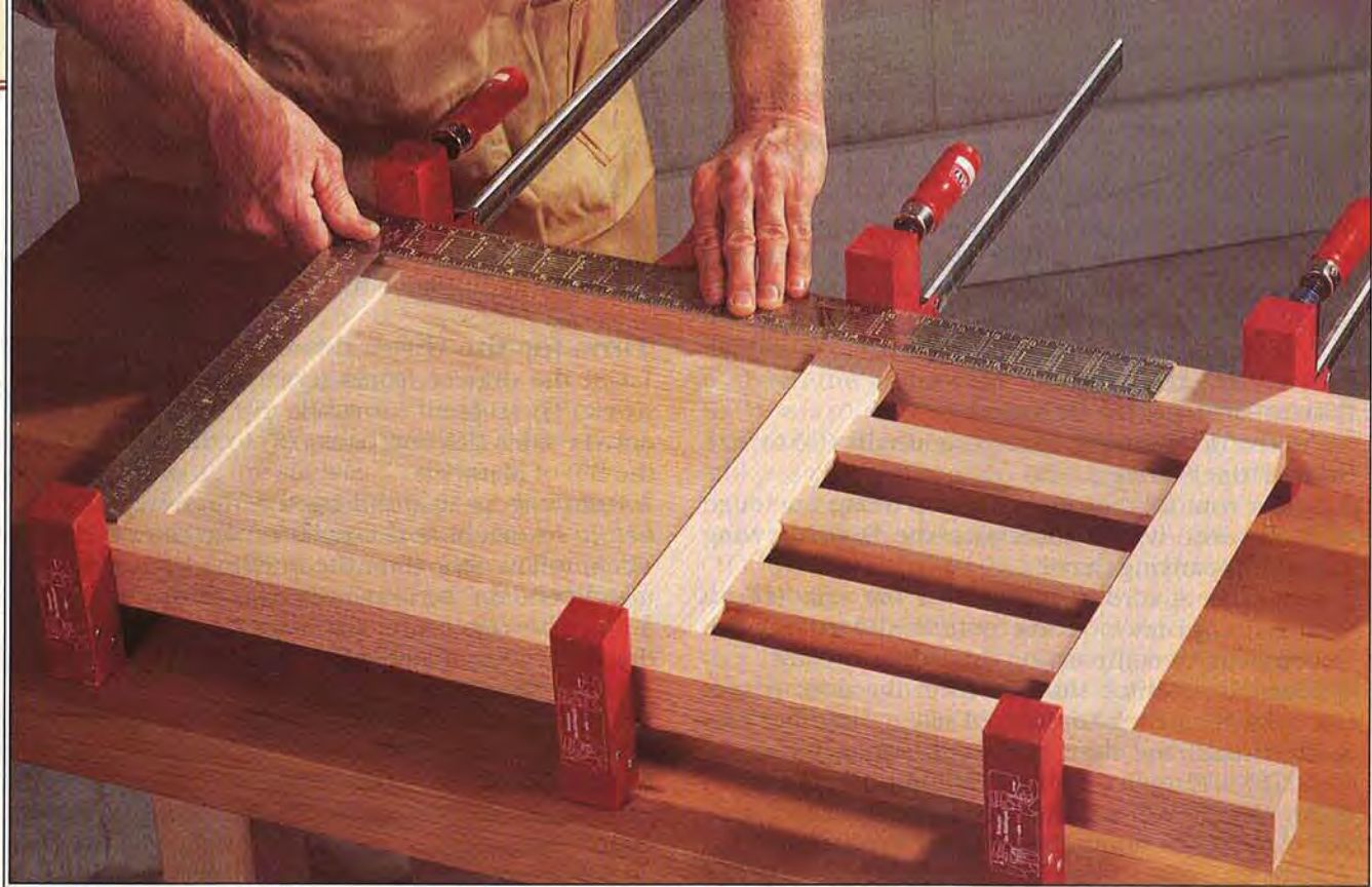
Glue and clamp each end panel, using a framing square to check for square and flatness.
