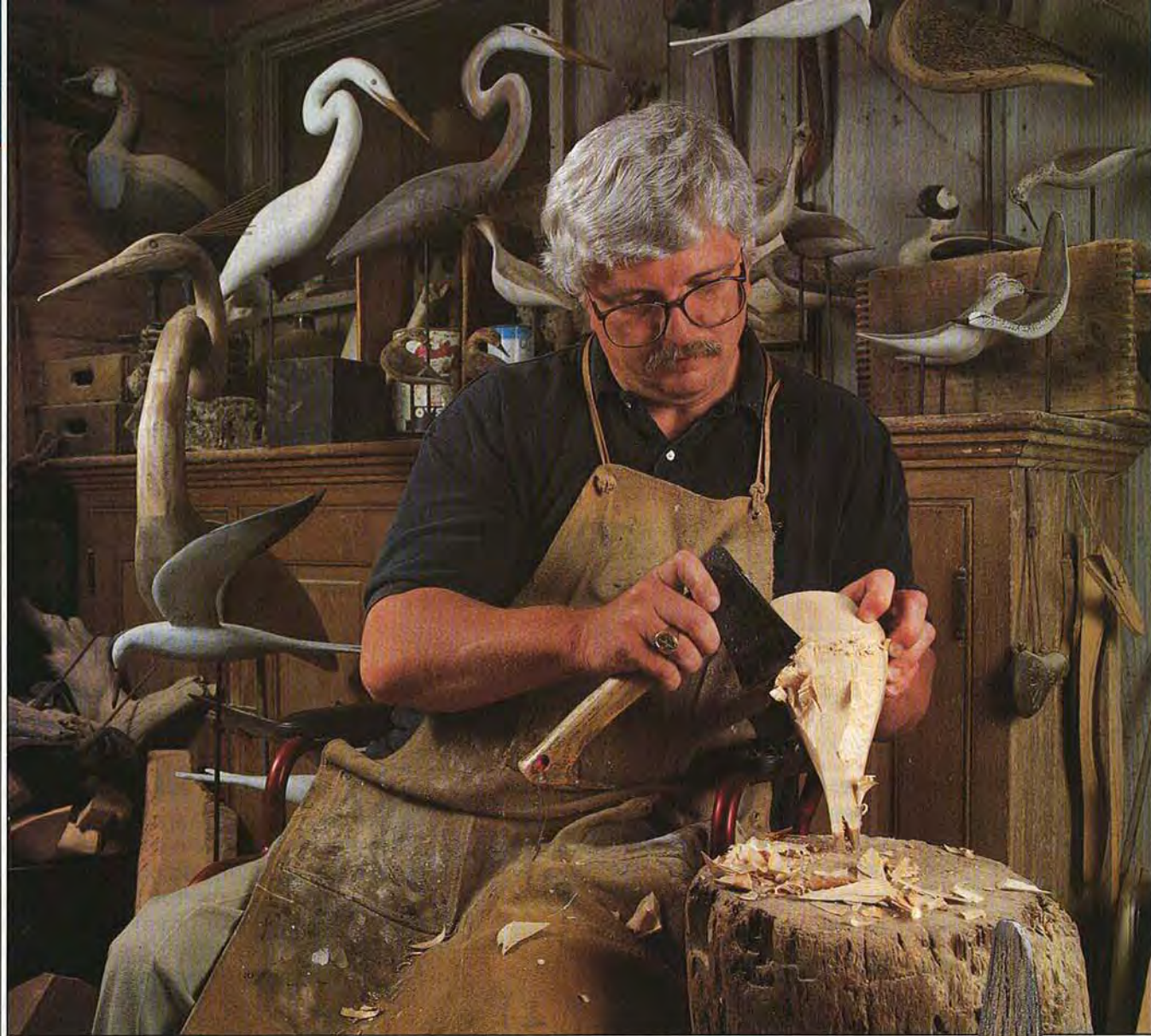
Shunning motorized tools as much as possible, the carver works the white cedar block to rough shape with a razor-edged hatchet on a chopping block made from an old stump.
