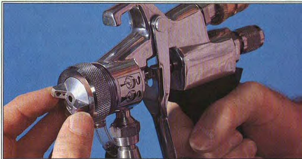
▲ Turning the air horns on the front of the spray gun enables you to change the shape of your spray pattern.
