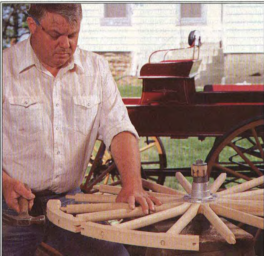
A 16-spoke wheel has eight felloes, each tapped into place on the spokes by hand, then joined and anchored to one another with wooden splines.
