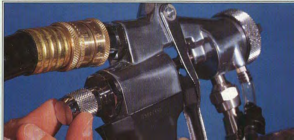
▲ Turning the air horns on the front of the spray gun enables you to change the shape of your spray pattern.
