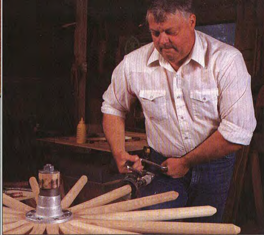
A cone plane chucked into a hand brace points the end of each spoke to act as a guide for the tenon cut.
