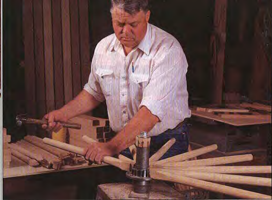
Sawed to an 11\frac{1}{4}^\circ angle at the hub end, each spoke wedges against another as Gary drives them in with a hammer around the wheel.
