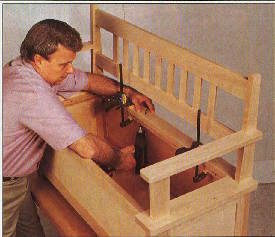
Working from inside the base, screw through the cleats to secure the seat-frame/seat-back assembly to the base.
