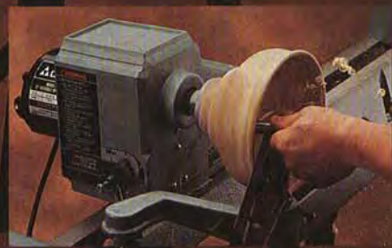
Turn stock 36" between centers, 12" over the cast iron bed or swivel the headstock 90° for outboard turning of work up to 16" diameter. Variable speed (500-2000 rpm) allows proper control for out-of-round and offset turning or roughing of green or seasoned wood through final finishing stages.
