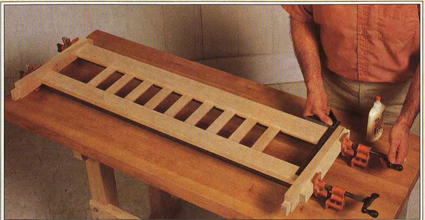
Immediately after clamping, check the seat-back assembly for square, and adjust the clamps as necessary.
