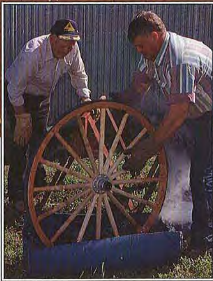
In the final cold water bath, the wooden wheel pops as all the wooden parts slip tightly into place under the force of the cooling and shrinking steel.
