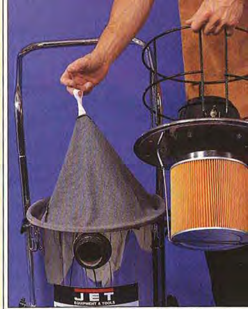
The Jet JV10 has a cloth tank liner and pleated paper filter for effective dust separation and easy debris disposal.
