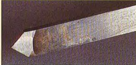
This parting tool, ground to the thickness of the inlay wire, cuts the groove.
