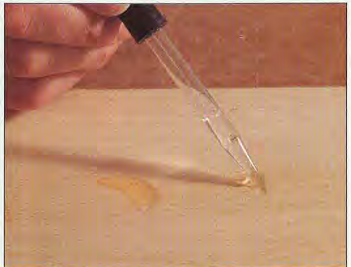
Fill the dented area with water from an eye dropper. Repeat until the dent rises up flush with the surrounding surface.
