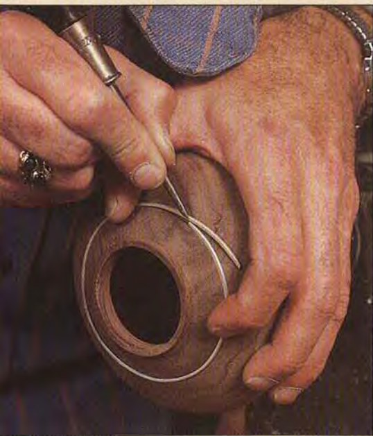
Lay the silver wire into the groove, then mark the length. Cut the end square for a close-fitting joint.
