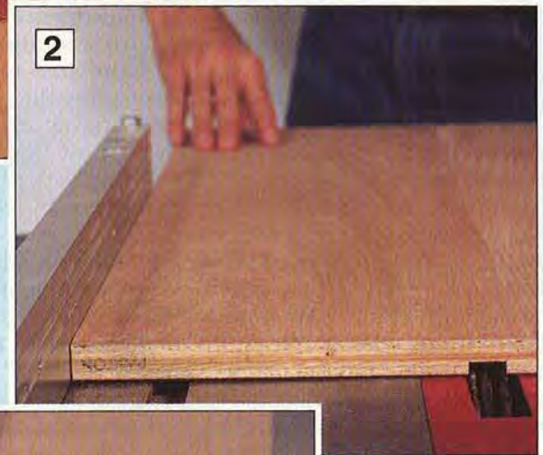
Left: From your matched piece of scrap plywood, rip a filler strip with your tablesaw blade set at 2^\circ from vertical.
