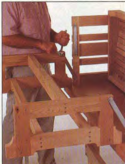
Connect the steel swing arms from the rear holes in the base to the rear holes in the seat assembly.
