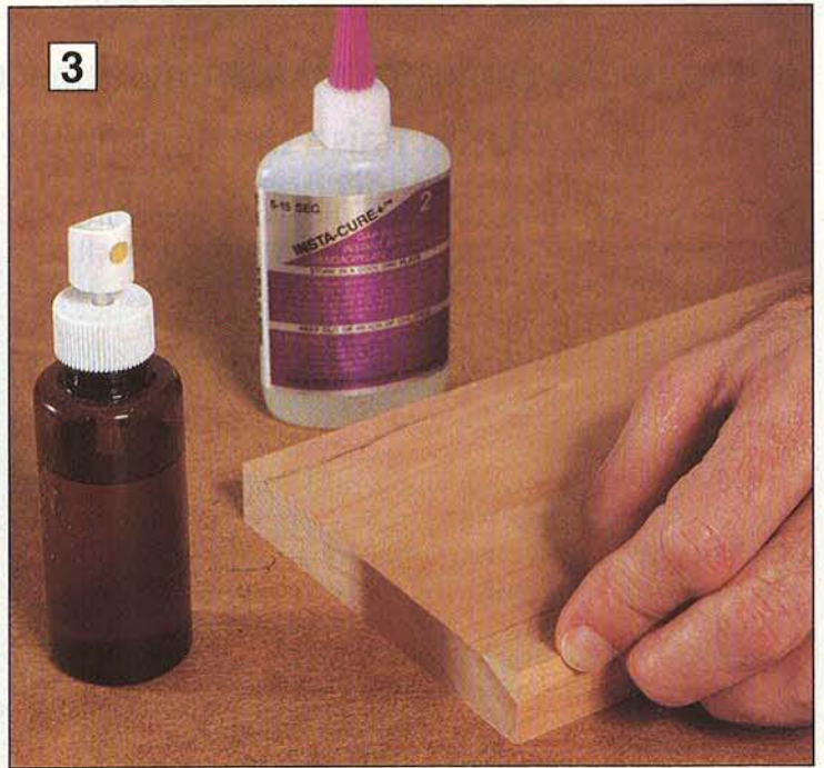
3 Use cyanoacrylate (instant) glue and accelerator to join the patch to the workpiece, and hold the patch in place until the glue dries.
