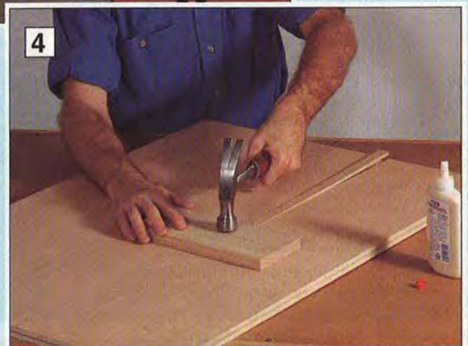
Right: Apply glue to the filler strip and groove, and tap the filler strip into place with a flat hardwood block and hammer.
