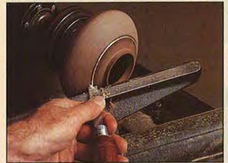
Clean up the inlay and surrounding wood with a light scraper cut. Remove as little material as possible.
