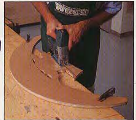
Clamp the rocker to your workbench for support when cutting the narrow cow's tail to shape.
