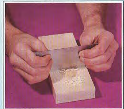
Scraping off dried polyurethane glue proves easy and won't dull or nick your cutting edges like AR glues can.
