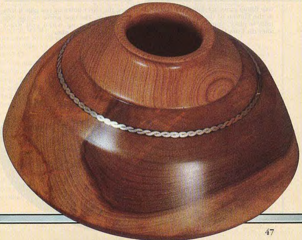
Cut the inlay groove straight into the vessel's side. A snug-fitting inlay looks best, so test-fit the wire as you work.
