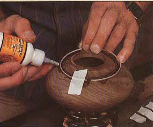
Gap-filling cyanoacrylate (CA) adhesive in the bottom of the groove holds the inlay in place. Apply CA along the sides after the inlay is in place.
