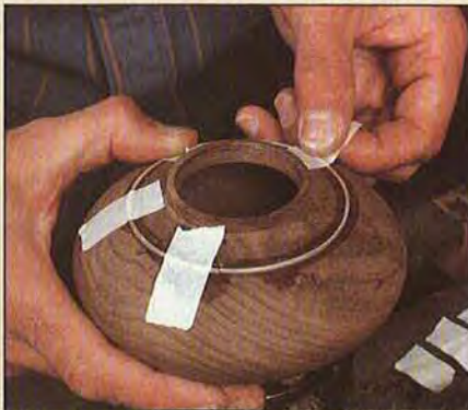
Tape the silver down as you glue it into the groove. The tape prevents one side from popping up when you press down on another.
