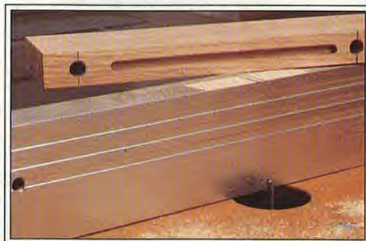
Using a fence to center the straight bit to the stock, rout a 1/4" groove 1/4" deep along the inside face of each stile (H) to house the top panel (L).
