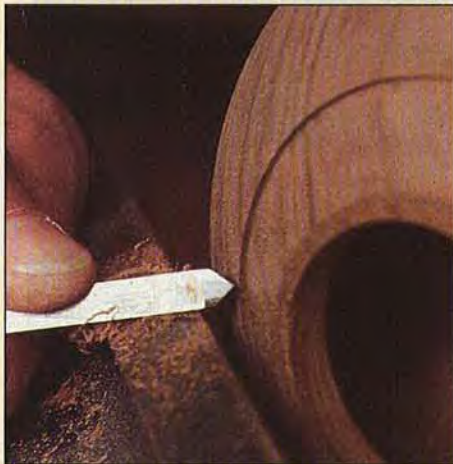
Cut the inlay groove straight into the vessel's side. A snug-fitting inlay looks best, so test-fit the wire as you work.
