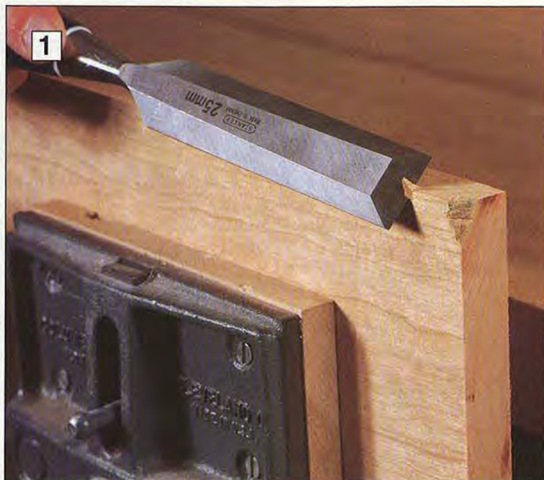
Secure the board in a woodworking vise and pare away the dented corner with the chisel positioned at 45^\circ to the edge.
