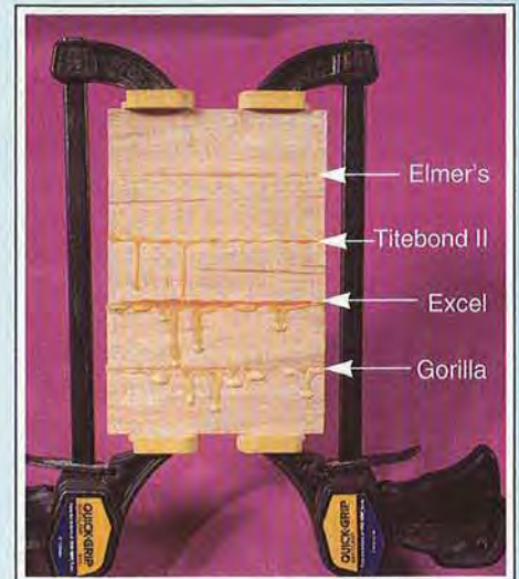
On vertical applications, glue squeeze-out can lead to a sticky situation. We purposely overloaded these joints to show how Elmer's Weather-Tite Wood Glue gel formula resists running.
