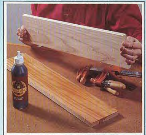
Polyurethane glues spread easily and need only be applied to one side or edge of a workpiece, making them ideal for large or complicated glue-ups.
