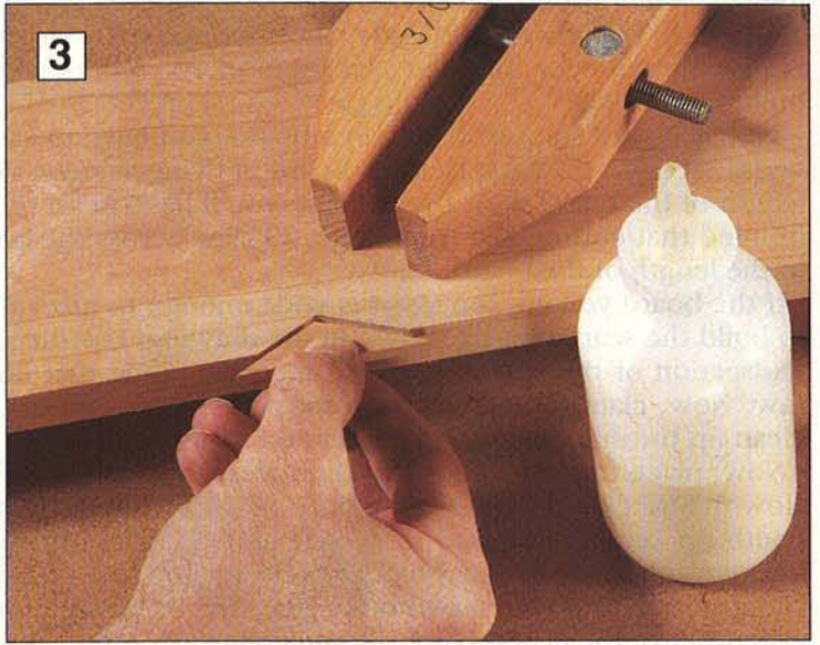
3 Adjust the patch for a tight fit by lightly sanding its inside edges, then glue and clamp the patch in place.
