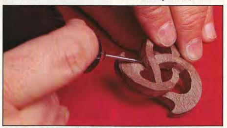
7. Undercut the strand crossings using a rotary power-carving tool with a small, spherical cutter. Don't try to cut all the way through from one side.
