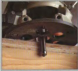
A piloted flush-trimming bit helps you quickly trim edges flush with adjoining surfaces.
