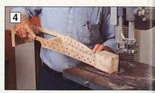
Above: Stan roughs out the shape of a carving on the bandsaw. The neck is for a baryton.
