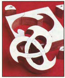
Cut out the blank with a scrollsaw or coping saw. We'll refer to the patterned side as the front of the pendant.
