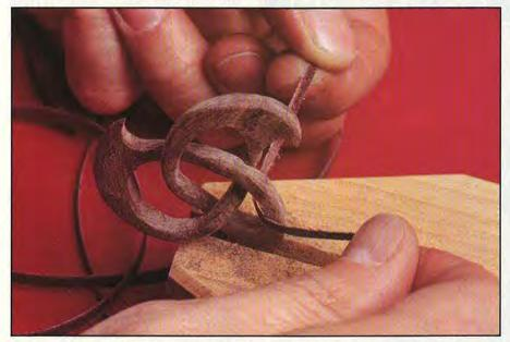
8. Clamp the pendant firmly when sanding with a strip. Work carefully, and stay close to the secured end.
