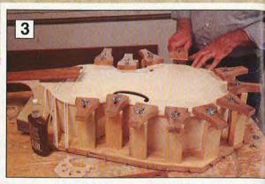
Above: This homemade clamping device ensures even pressure along the curved edges.
