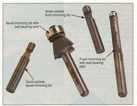
Bevel-trimming and flush-trimming bits come with or without ball-bearing pilots. Ball-bearing types are less likely to mar your plastic laminates.
