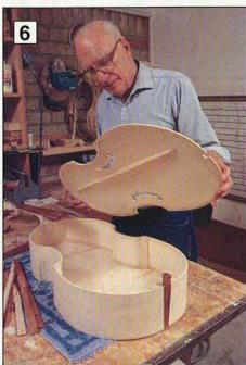
Above: With the lining in place, Stan testfits the top prior to glue-up.
