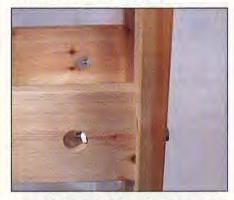
Most of the tested benches have bolts and captured nuts that join their stretchers and legs.
