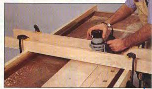
Note: These procedures work for any solid-wood top that's at least 1" thick. We recommend you flatten your benchtop if it's uneven by more than ½32". (You can check for flatness by moving a straightedge across your benchtop.) Do not try these flattening steps on laminated tops made of plywood, particleboard, hardboard, or similar materials.
