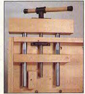
components mounted to a nearly indestructible 5"-thick edge, are the undisputed champs in this category. Among the "little things that count" that we noticed with the Ulmia vises were the square-tooth threads of their screws as shown in the drawings below. These threads cost more to manufacture because they have to be machined to exact tolerances for a tight fit. The tapered-tooth
