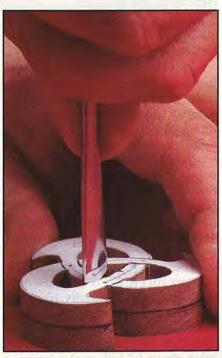
4. Keep the gouge perpendicular to the surface when stop-cutting.
