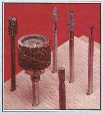
We roughed out the pendant with the five bits and small sanding drum shown. Any similar bits would work.
