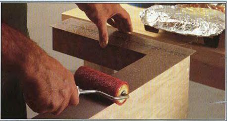
To conveniently apply adhesive with a short-nap roller to a piece of laminate, place the laminate face down on its mating substrate.
