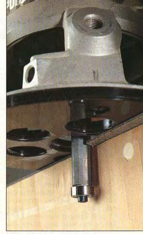
When trimming with a straight bit, set its depth so its pilot does not go into any slight indentations from countersunk screws.
