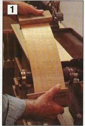
Above: After soaking a baryton side, Stan heats it on a soldering iron sheathed by a copper pipe.
