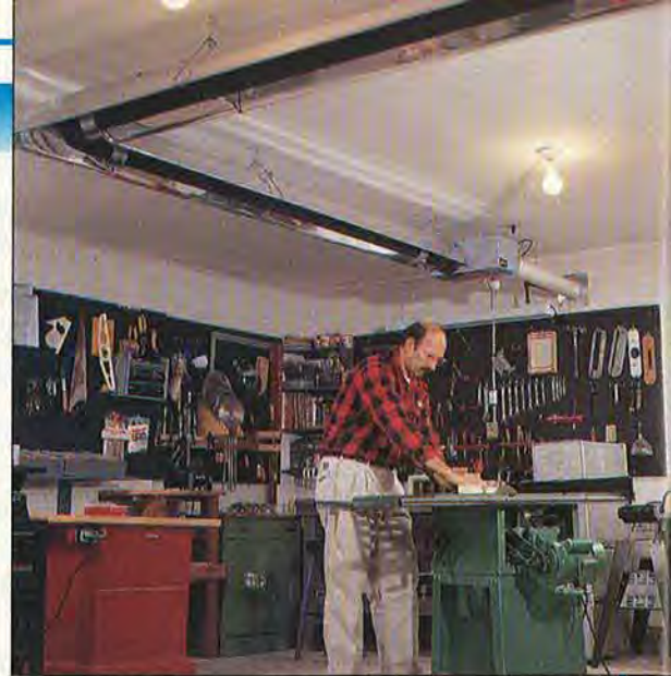
Jim Harrold, managing editor of WOOD ® magazine, enjoys a cold January day woodworking in his garage shop. An overhead radiant heater spreads warmth throughout the space.
