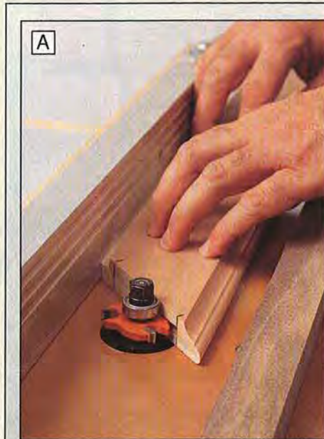
Slide the miter-cut tabletop piece along the router fence and into the spline-cutting bit.
