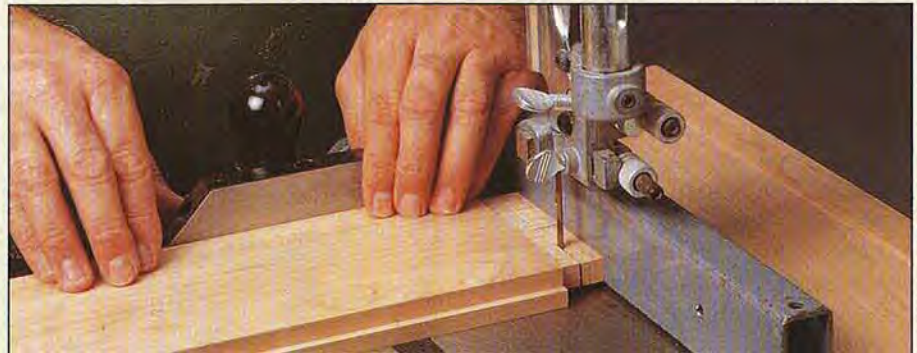
After cutting the rabbets to form the tenons on the tablesaw, mark the notches and cut them to shape on the bandsaw.
