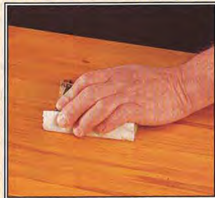
Rubbing down the final coat of shellac with 320-grit sandpaper moistened with linseed oil ensures a smooth ending.
