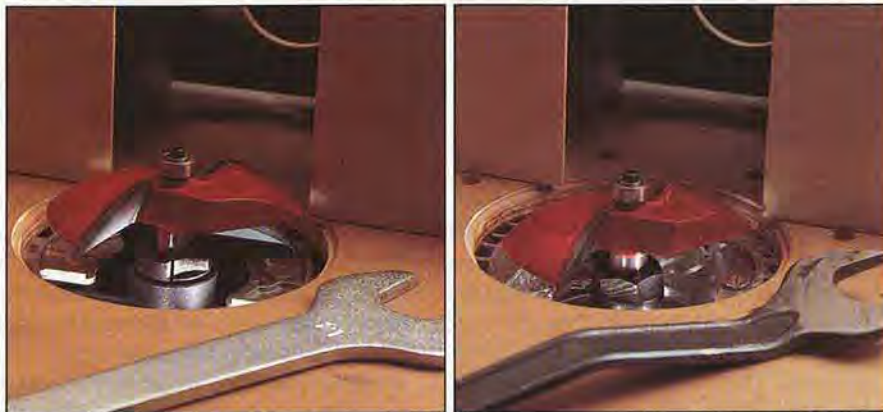
The collet nut on the Hitachi M12V (left) comes to within \frac{1}{8} " of the top of a \frac{3}{8} "-thick router-table plate, making it simple to change large-diameter router bits without removing the router from the table. To do this with the DeWalt DW625 (right), we had to bend the wrench to reach the collet that comes to within \frac{1}{2} " of the top.
