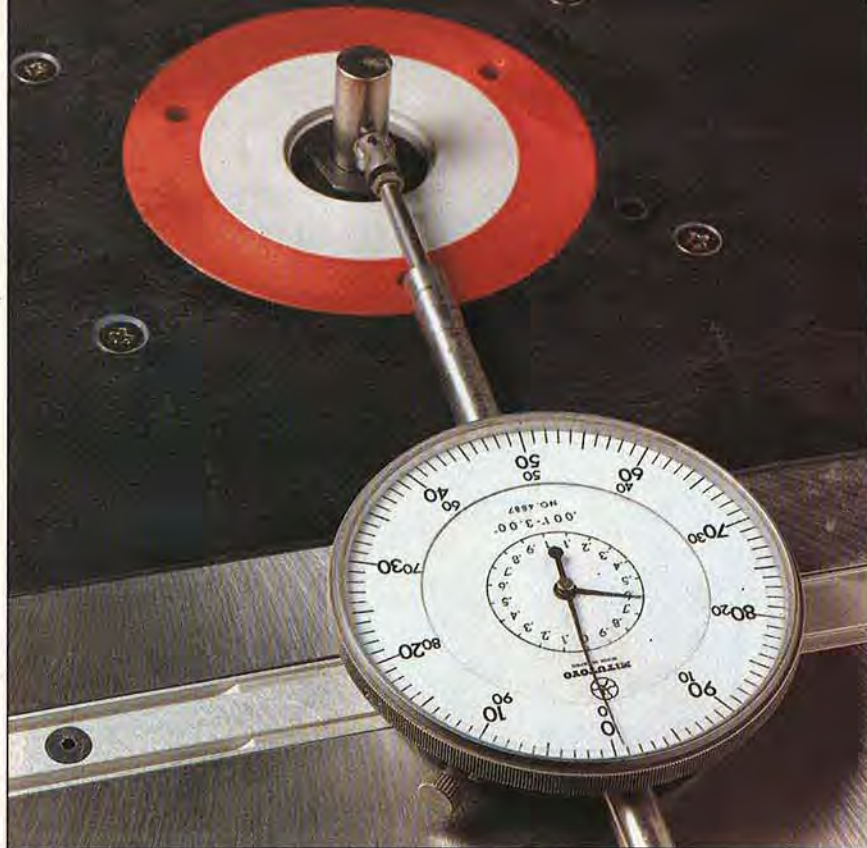
We placed a precision-machined shaft into each router's collet and measured runout with a dial indicator.
