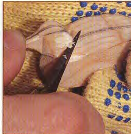
A knife is all you need to carve the letter opener. Make whittling-style shaving cuts to minimize chip-out.
