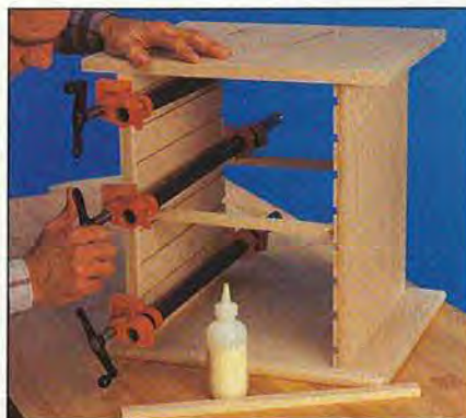
Using 12"-long spacers to hold the side-panel middles exactly 12" apart, glue the front bands to the side panels.
