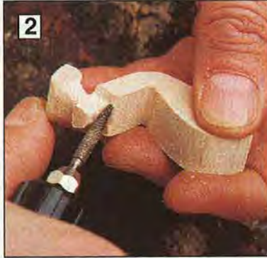
2 Form the heel and establish the cuff line at the back of the leg. Shape the insole and front of the shoe.
