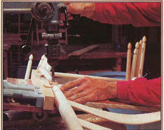
Because the back posts are bent as well as flared at the top, the 1"-deep mortises for the rungs must be precisely drilled. Charles relies on a jig to get the perfect angle.
