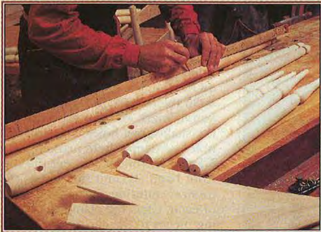
An important tool in Charles' chairmaking is the story stick—one for each model of chair. Using it as a guide, he marks the overall length of the back posts and the location of mortises.
