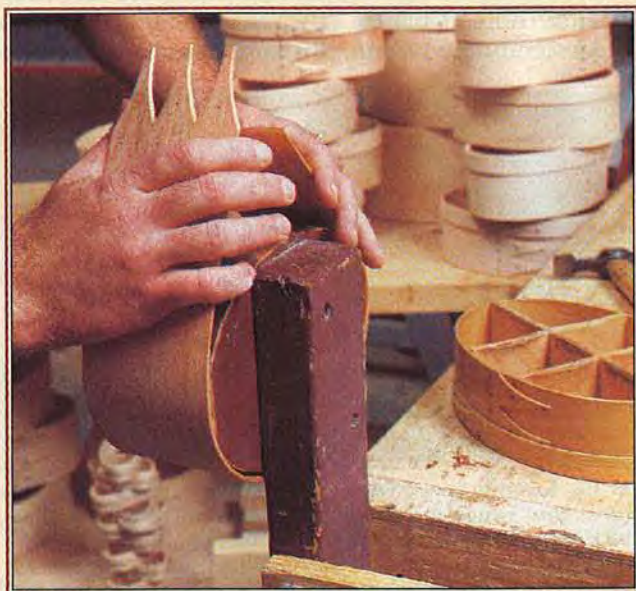
Still warm and wet from boiling, the maple band is bent around a form made from solid wood.
