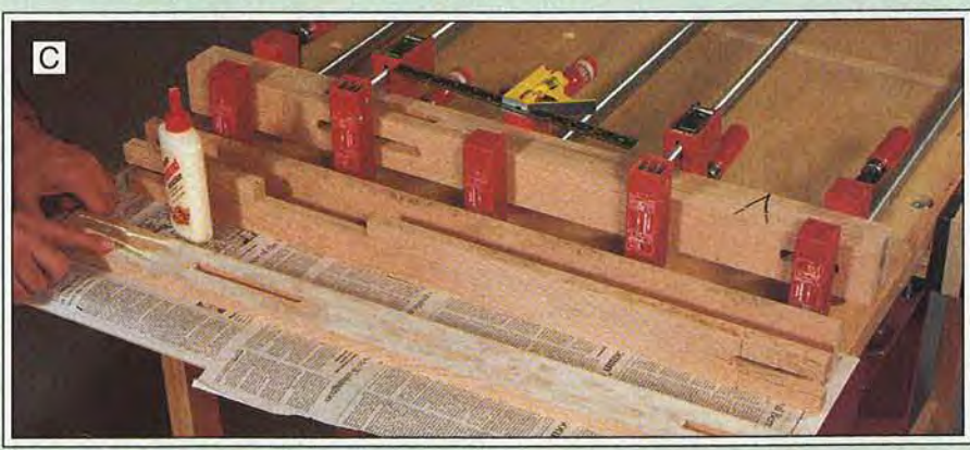
C Spread an even coat of glue on the mating surfaces, and glue the three pieces together that form each leg.
