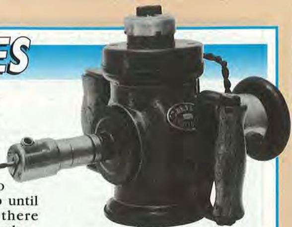
The world's first electric power tool, the Fein Electric Hand Drill, 1895.
