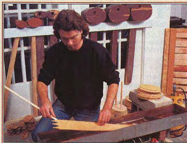
To soften the maple band for a box side, James Majcher boils it in water for about 20 minutes. A propane camp stove fires the unit.
