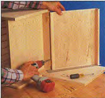
Using a piece of \frac{3}{4} " plywood and a \frac{1}{16} " spacer, center the door between the top and bottom panels. Attach the hinges.
