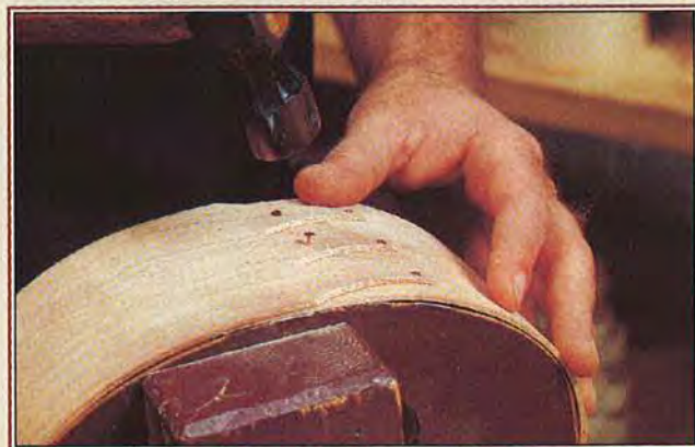
Copper tacks hold the swallowtail joint together. The Shakers commonly made their boxes with the tails of the joint pointing to the right. And the tacks lined up perfectly.
