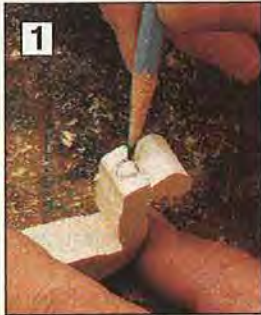
1 Center the heel outline on the bottom of the leg blank. For clownish feet, make the heel narrower than the front of the shoe.
