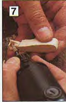
7 Form the palm of the hand by enlarging the drilled hole with a tapered carving bit.
