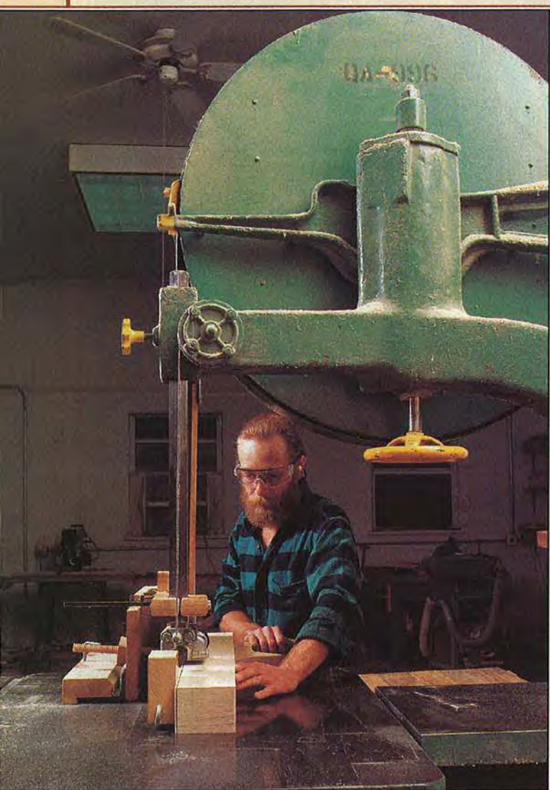
Ron Seiber resaws maple for boxes at the 1951 Moak band saw. It has a 24" throat and a blade over 19' long.
