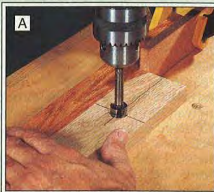
Using a Forstner bit in your drill press, drill a \frac{3}{4} " hole at the marked centerpoint on each leg centerpiece.
