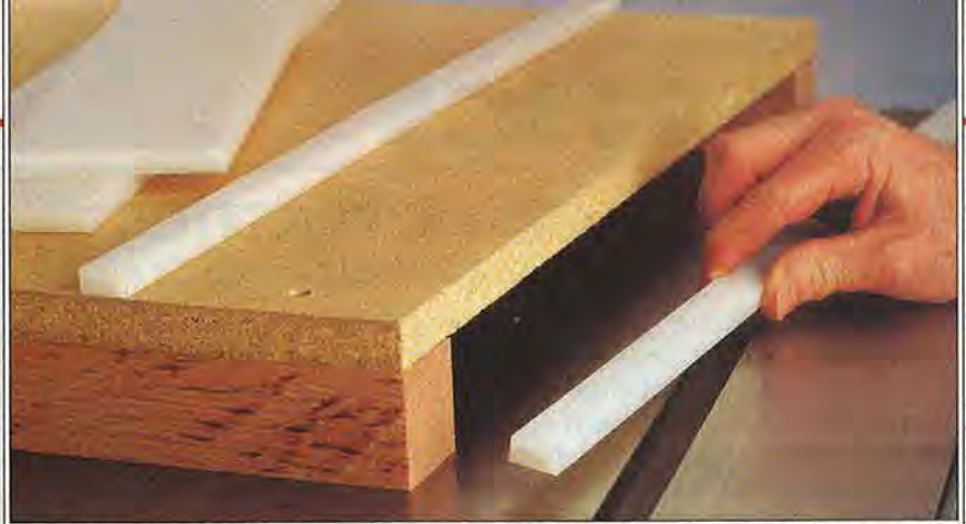
On the bottom of a tablesaw cutoff jig, UHMW polyethylene slides like silk in the miter-gauge slot.
