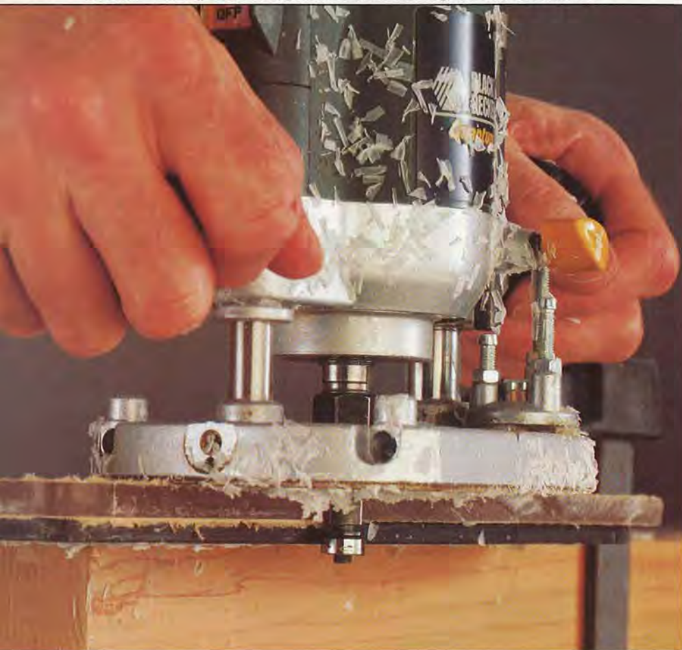
A router with a piloted straight bit cuts a clean edge around a template.
