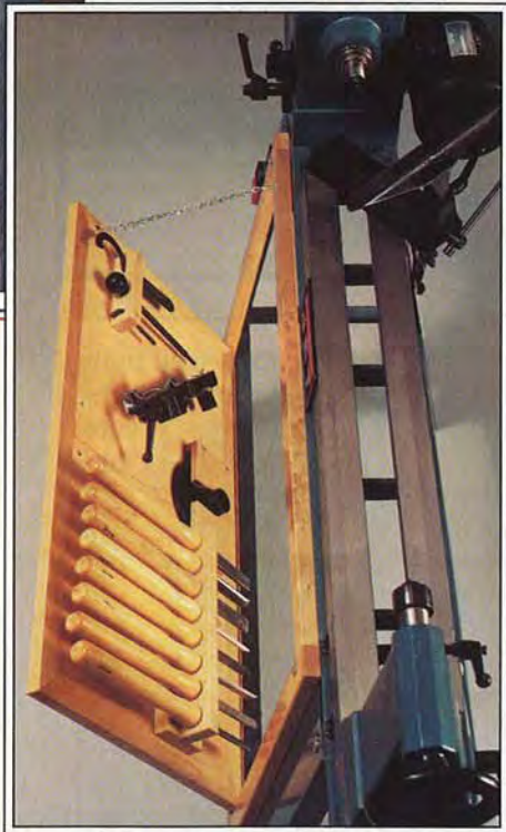
Hinged door (open), viewed from top of lathe.
