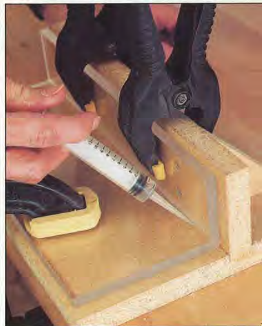
Capillary action draws the glue out of the syringe and into the joint.
