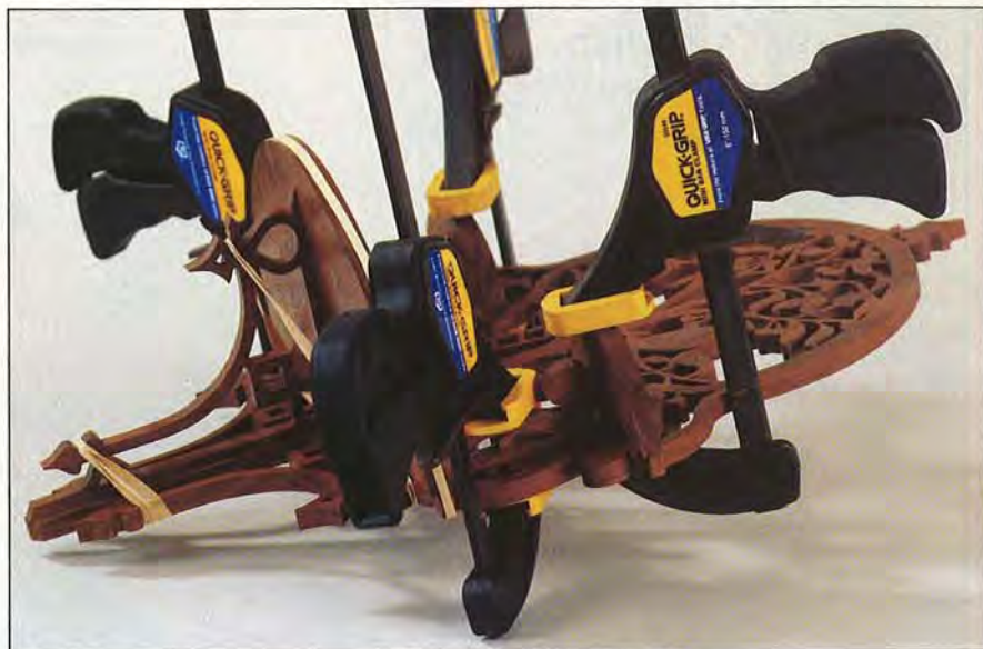
A combination of bar clamps and rubber bands will hold the shelf together securely while the glue dries.
