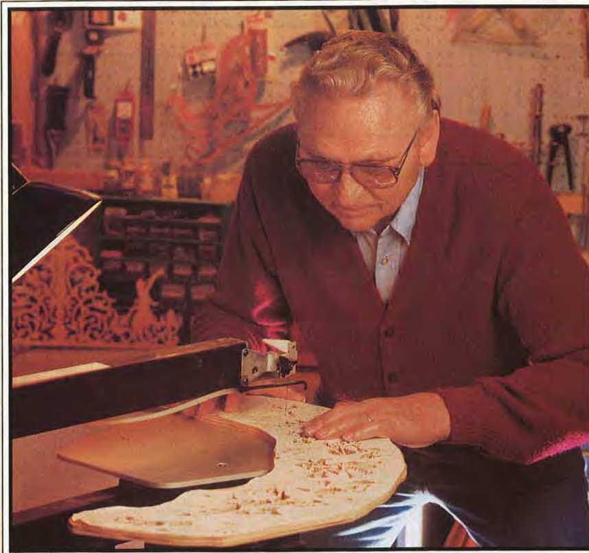
The large patterns that Carl prefers to cut out require a scrollsaw with a 30" throat.
