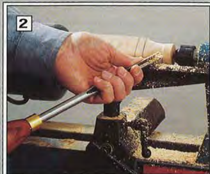
2 Turn the ends round from the outer line outward. If the turning stops too easily, increase the tailstock pressure.
