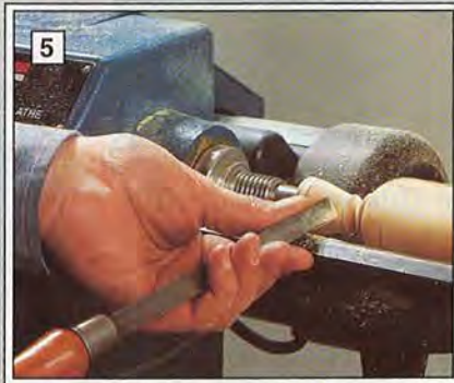
Guidelines drawn on the turning will help you position the knob features. Check the template as you work.
