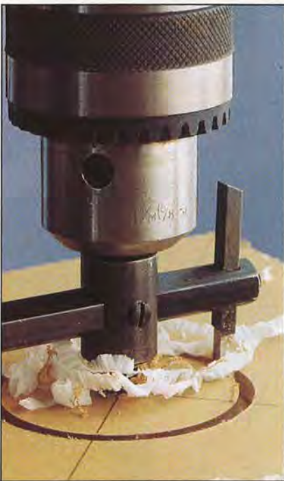
With the shaft in the hole, the cutter can scribe a smooth circle.
