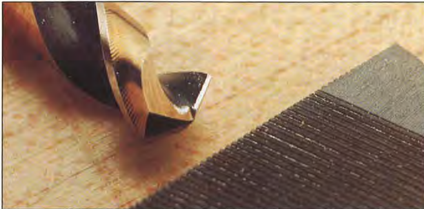
Filing a small flat on the cutting edge prevents drill bits from grabbing at the plastic.
