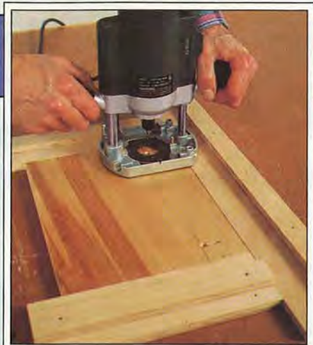
Use end and top guides to guide and stop the router when routing the keyhole slots in the plywood back.
