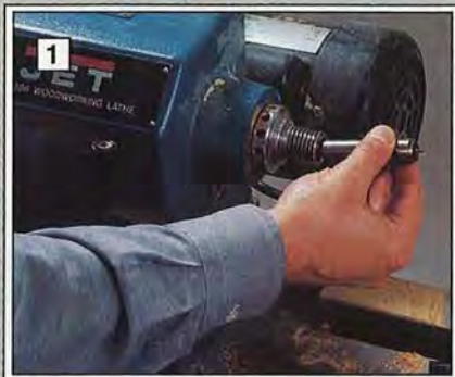
1 Install a dead (nonrotating) cup center in the headstock. This way, tool catches are less likely to damage the turning.
