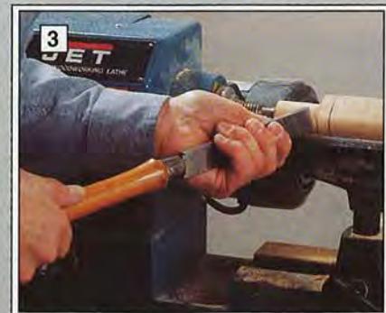
3 Square the shoulder with a skew before rough-turning the handles. Cut to the outermost line.
