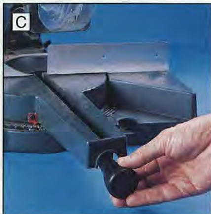
Miter-locking knobs like the one on the Sears Craftsman machine proved quick and easy to secure.
