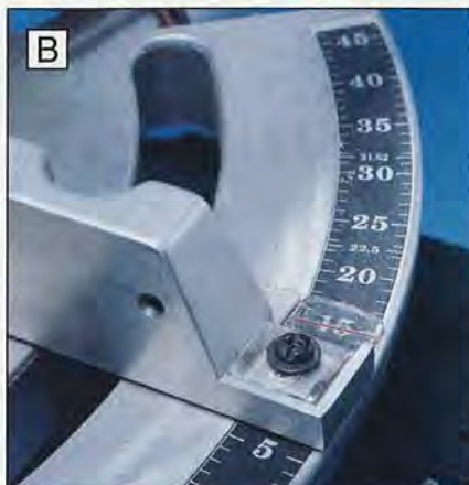
Attached sheet-metal or tape miter scales, such as the Delta Sidekick's here, are easy to read and help you make fine miter adjustments.
