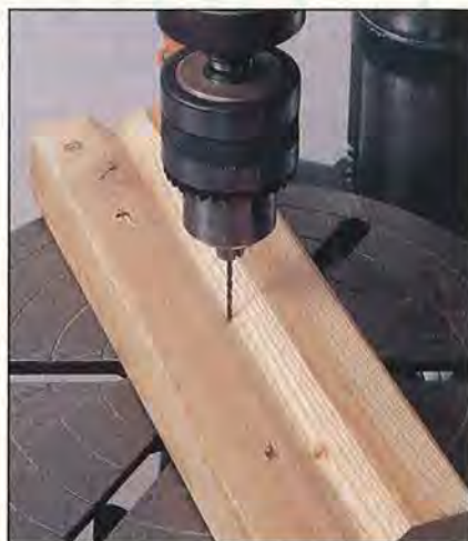
Center a V-block on the drill-press table to hold the columns and crossbar for accurate drilling.
