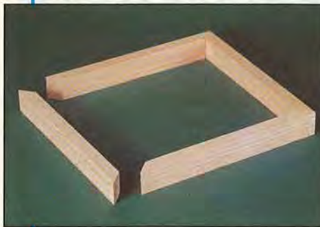
Beveled sides result when you set the miter gauge to 90° and tilt the blade to a 45° angle.
