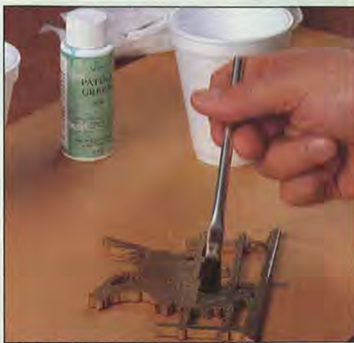
Brush on the patina solution while the second coat of metallic paint is still tacky.
