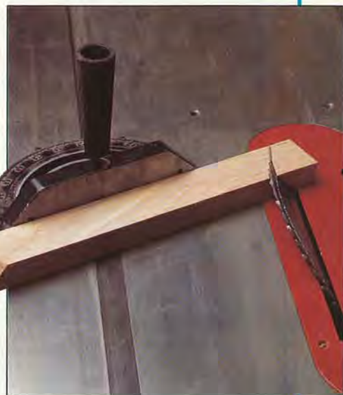
A compound miter results from sawing a miter with the blade tilted. You can find the bevel and miter settings you need by referring to the compound-miter chart on page 6 .
