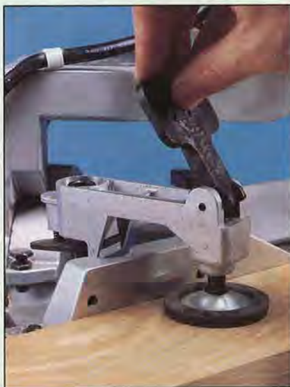
The cam-style work clamp on the Delta Sidekick proved quick to adjust.
