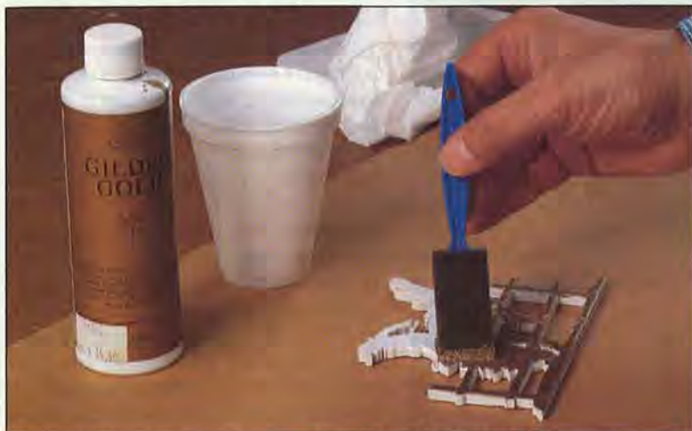
Apply the metallic coating smoothly and evenly to give the project a realistic look. Allow first coat to dry before putting on the next.
