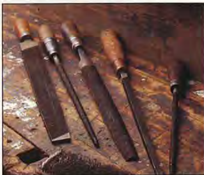
With just a few files you can "turn" brass. File shapes shown from left are mill, round, half-round, and square. At the far right is another round file. Clean the files with a file card, bottom.
