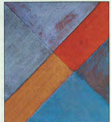
You can apply either the blue (top) or green patina solution over either the gold (left) or copper base coat.
