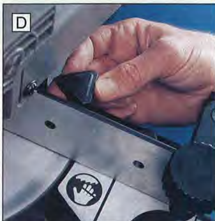
Miter-locking knobs located behind the fence were effective, but a bit of a hassle to reach and operate.
