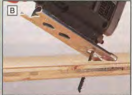
Turn on the saw, and lower the blade into the wood, causing the reciprocating blade to cut through the plywood at the marked cutline.
