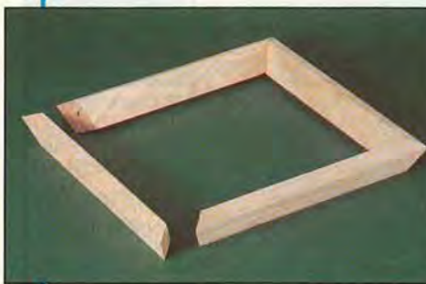
Slanted sides call for compound-miters, a combination miter-cut and bevel-cut.
