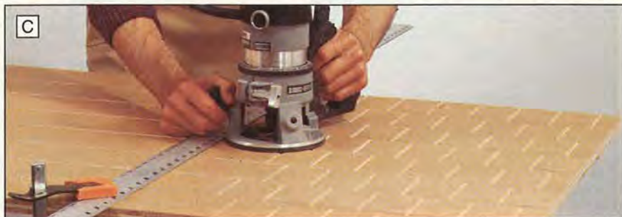
Using a straightedge to guide your router, rout the shingle facsimile lines in the roof panels. We used a \frac{1}{4} " round-nose bit for this procedure.
