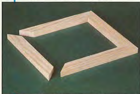
Mitered sides result when you set the miter gauge to a 45° angle and leave the blade vertical.
