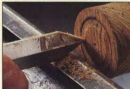
Establish the diameter for the cork recess with a parting-tool cut.
