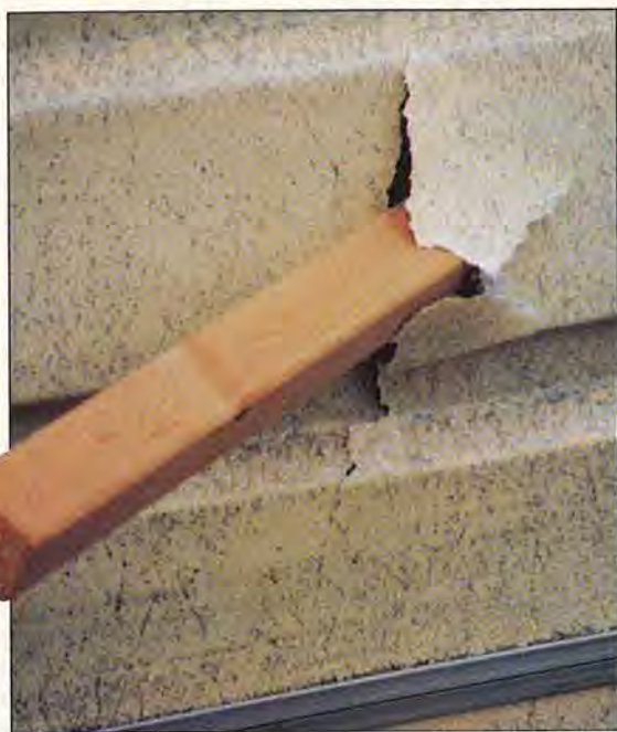
For this photograph, Victor Baker re-created what happened when his radial-arm saw kicked back a 2x2x18" piece of pine. It penetrated a fiberglass garage door and flew 15' into the driveway.
