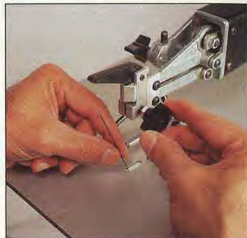
Excalibur's cam-operated tensioning lever and thumbscrew-action blade clamp help you install upper saw-blade ends quickly.
