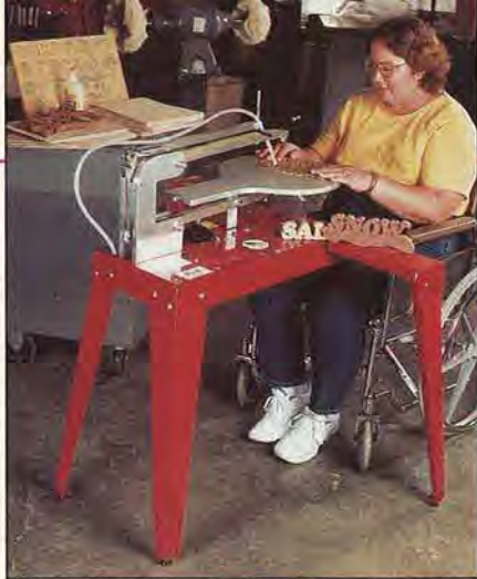
RBI offers a special wheelchair accessible leg package for its Hawk Ultra 226 scrollsaw.
