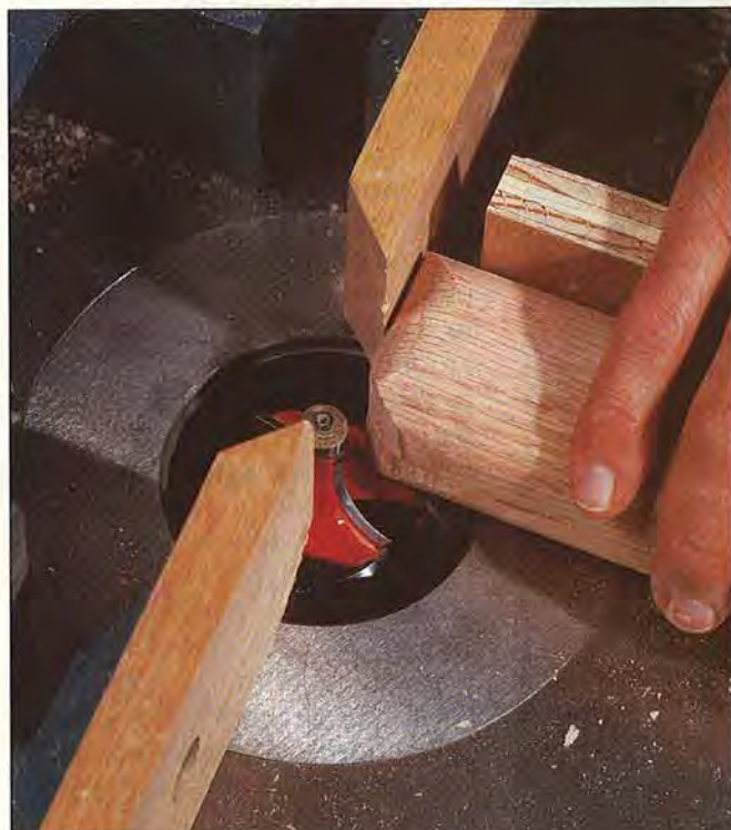
With the knob blank placed against the miter gauge and at a right angle to the router-table fence, round over the ends.
