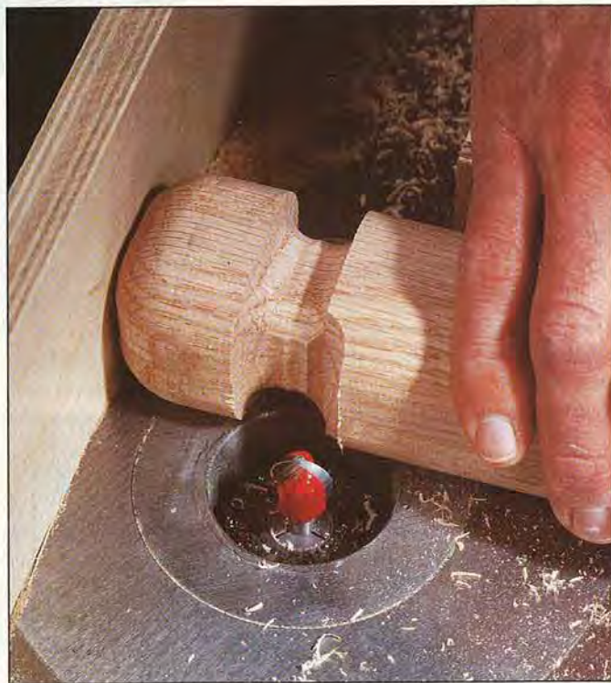
Using your miter gauge and a ¾" round-nose bit, rout the knob-to-shaft taper and the shaft with multiple passes.
