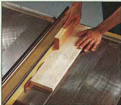
A pushblock, a zero-clearance insert, and a splitter allow you to safely cut all the thin strips.
