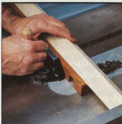
Secure a 45° V-block support to your miter gauge to cut the 3/4" notch in each leg.
