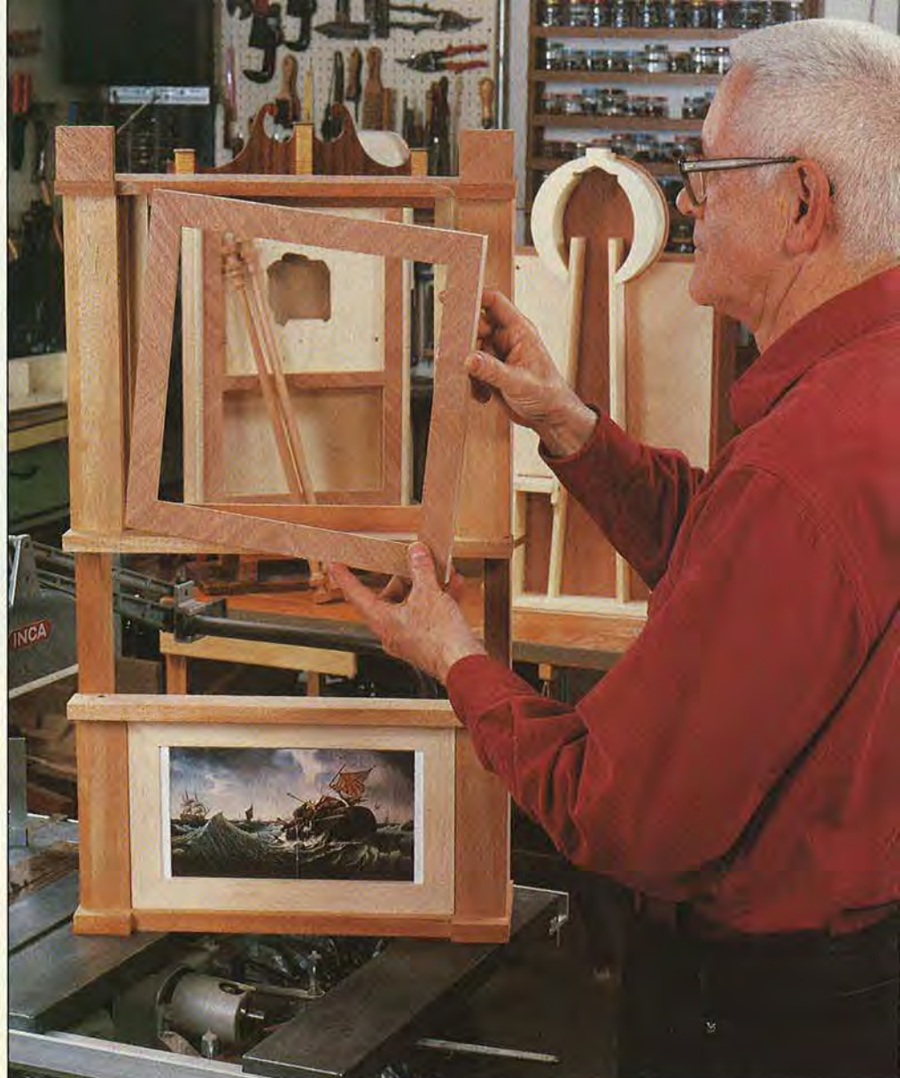
Ed builds few "triple-decker" clocks, but the one he's assembling will feature a whaling theme, popular in New England during the period. Note the "subdial" visible behind the clock he's working on. It will support the movement.
