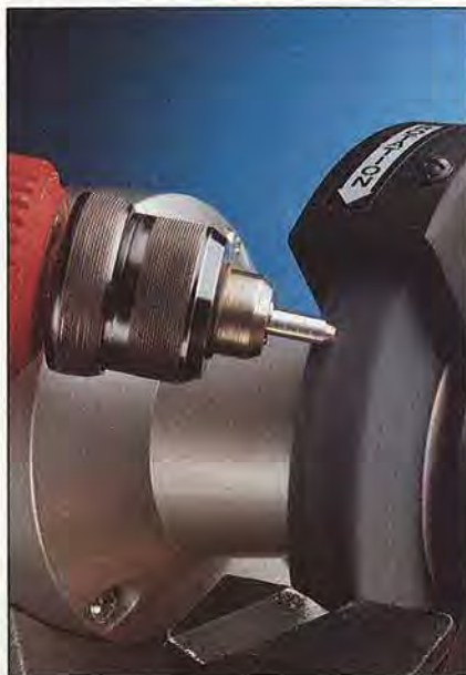
Grind the end of a \frac{1}{4} -20 \times 2" hex bolt to make the \frac{1}{8} " stylus.
