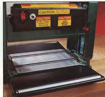
Like the similar Central Machinery and AMT planers, the Bridgewood has table rollers that we found difficult to adjust.
