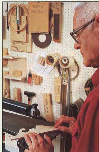
Ed makes the scrollsawn splats (top trim pieces) for coffin clocks from 1/4" curly maple or mahogany with a cross-grain inlaid plinth up the center.
