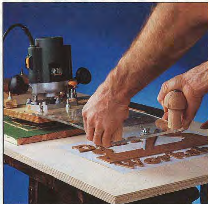
Carefully lower the router bit onto the workpiece while positioning the stylus in the waste area of your template. Arch the stylus plate to engage the stylus before the bit touches down.
