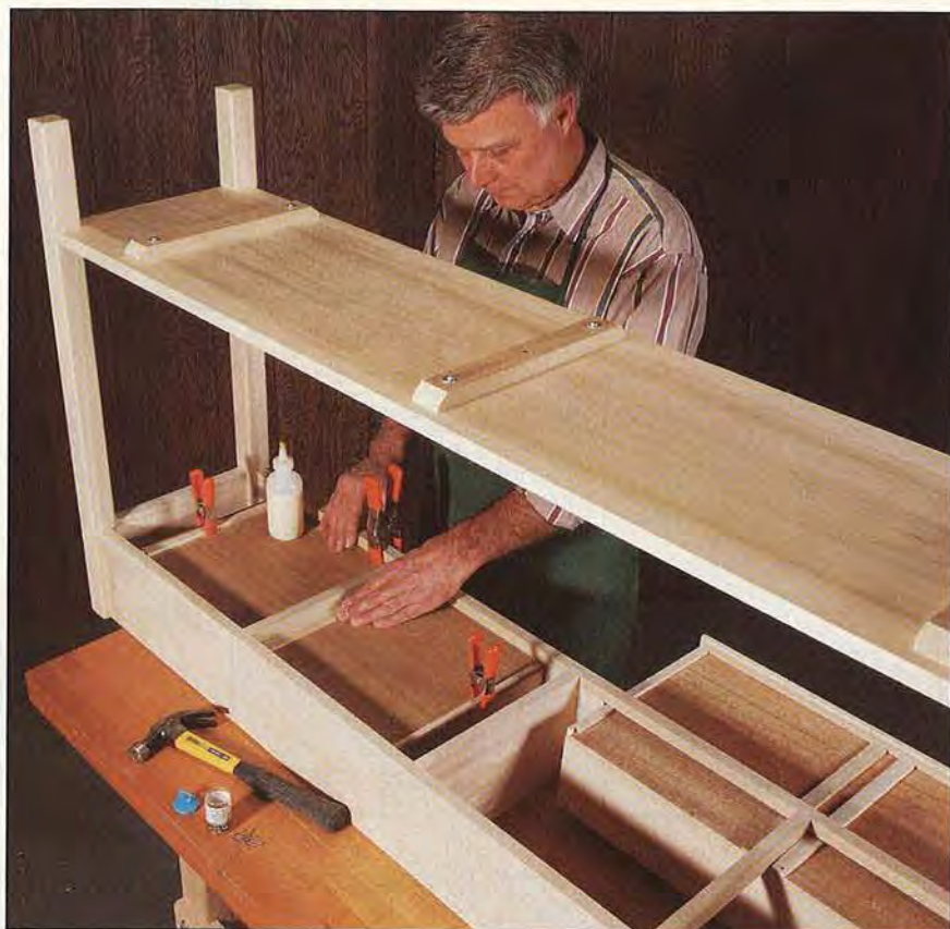
Slide the drawer bottom guides against the drawer supports, and then glue and nail the guides to the drawer bottoms.
