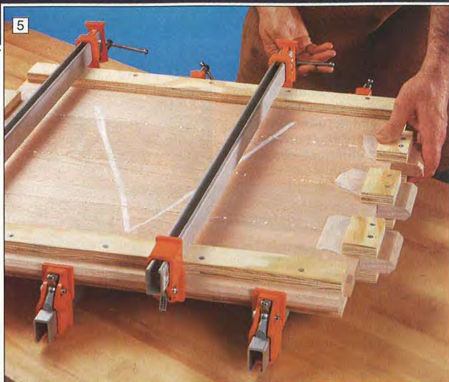
5 Draw up the clamps evenly, working outward from the center. Avoid excessive pressure; overtightening the clamps weakens the glue joint and may bow the panel.
