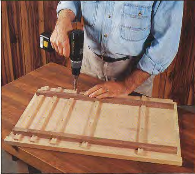
A pair of dadoed spacers allow you to accurately locate the drawer guides on the inside of the side panels.
