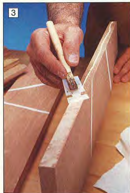
Strip the foam off a used foam brush, and you'll have a firm plastic glue spreader with a handle.
