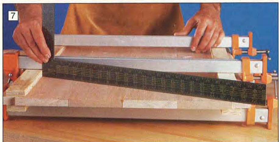
7 Use a framing square or other straightedge to check the panel for flatness.
