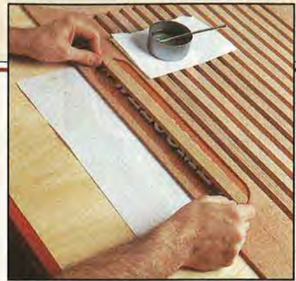
Double-faced tape holds the letters and stars on the stick for easy and accurate positioning in the epoxy-coated recess.
