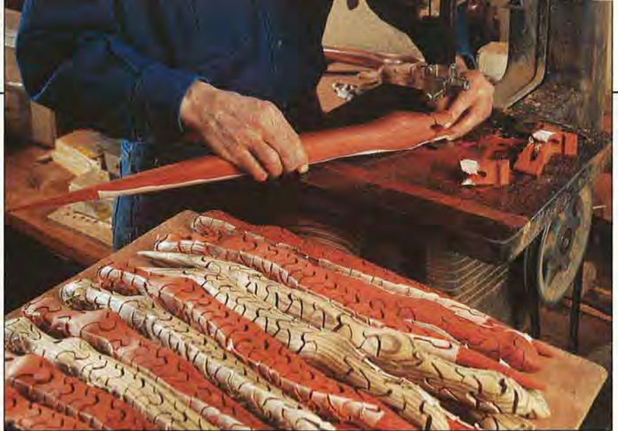
Peter bandsaws these snakes into puzzles from head to tail, turning the workpiece 90° after each cut so that the pieces cleverly interlock.
