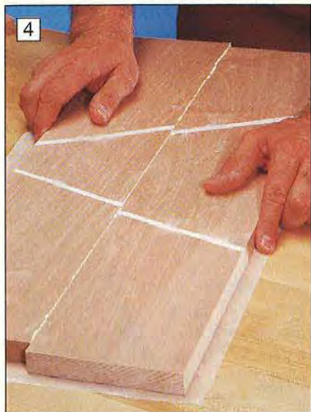
4 Rubbing the glued edges together gives the glue a chance to “grab,” making assembly easier.
