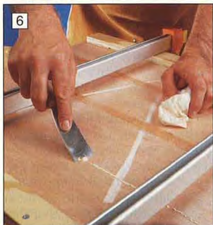
6 Scrape away glue squeeze-out with a putty knife. Then, use a wet rag to remove all traces of the glue.
