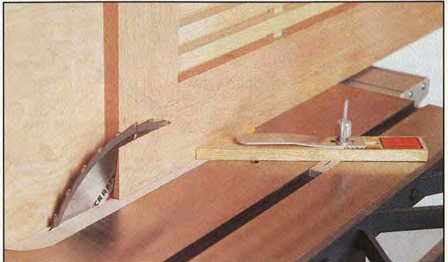
The combination of a tall auxiliary rip fence and a feather board allows you to saw the wide chamfers safely. Because the blade doesn't cut quite deeply enough, you'll need to complete the chamfers by planing or sanding.
