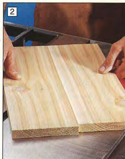
Use your saw table as a flat reference to check jointed edges. There should be no gap. Turn boards over, and repeat.
