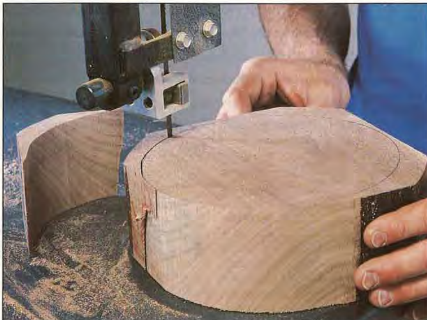
Out-of-balance stock will make the lathe vibrate excessively, so round-down rough stock for faceplate or between-centers turning before mounting it.
