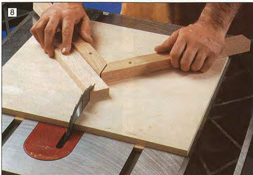
Make the first cut on each workpiece as shown. Then, clamp a stopblock to the jig to ensure that workpieces are the same length.
