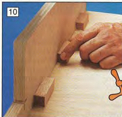
Coat the edges of a glue block with glue and rub it back and forth until the glue grabs. No clamping is necessary.
