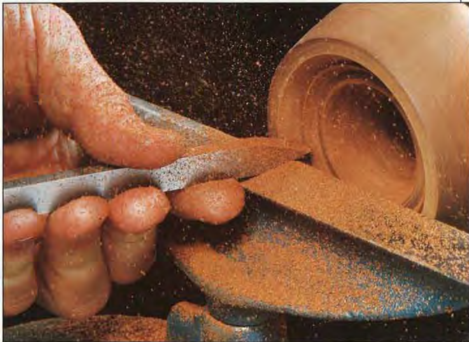
For safe turning, keep the tool rest about \frac{1}{8} " from the stock. This prevents the tool from catching and being thrown.
