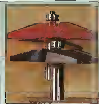
The sliver of gray on the Freud bit is all the carbide that can grab the wood should a kickback occur. The larger exposed area of carbide on the bit in front can cause a much harder kickback.
