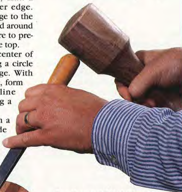
Pop the wasteblock from the base disc with a chisel and mallet. Keep the back of the chisel flat against the base disc.
