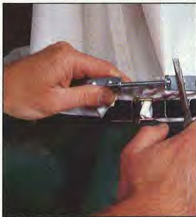
Hose-type band clamps supplement the cinch straps, as shown, on the two larger Grizzly machines. Used alone, the cinch straps can work loose, allowing the bags to blow off.
