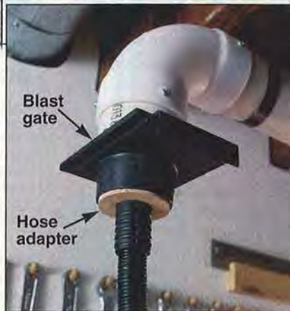
A blast gate, above , lets you shut off the flow to an unused port. Join hoses of different sizes with an empty can, right .
