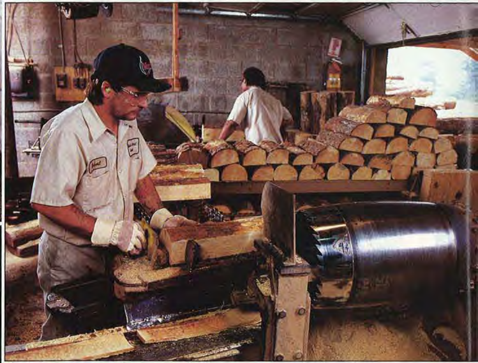
Above: Outside the cooperage, James Ennals trims raw logs to stave length. A powered carriage moves the 36"-diameter blade forward and back.
