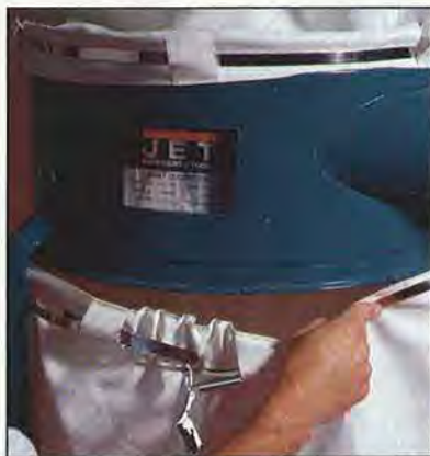
The makers of JET sew elastic into the mouth of its bags to help hold the bags in place while you flip the band clamp shut.
