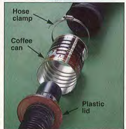
A blast gate, above , lets you shut off the flow to an unused port. Join hoses of different sizes with an empty can, right .
