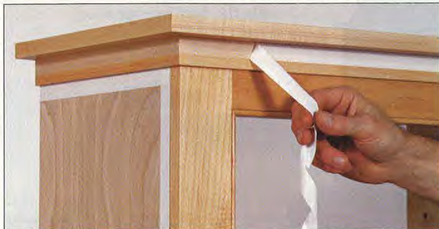
After applying the clear finish, remove the masking tape, including that where the crown molding needs to be glued.
