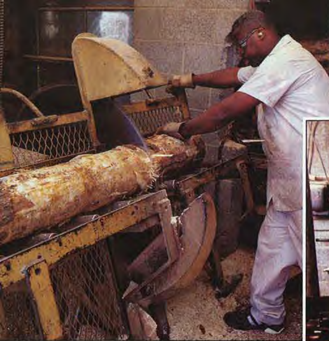
Above: Outside the cooperage, James Ennals trims raw logs to stave length. A powered carriage moves the 36"-diameter blade forward and back.
