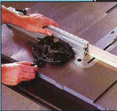
We do not recommend operating without the saw blade guard, as is shown here. US Patent #5,038,486
