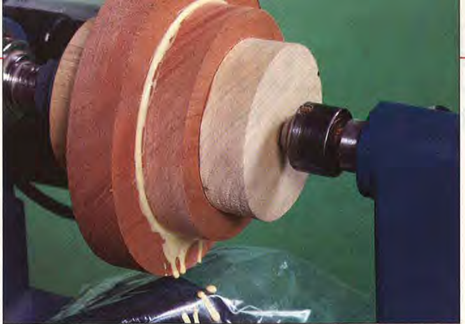
The lathe serves as a clamp when gluing the base discs together. A plastic bag protects the toolrest and lathe bed from dripping glue squeeze-out.
