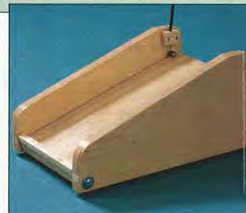
The foot pedal connects to the lever using a bicycle brake cable.
