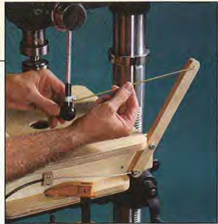
Connect the brass rod to the plastic clamp on the end of the feed lever.
