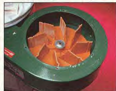
SECO's manufacturer installs plastic impellers (above) in all models except the UFO102B.
