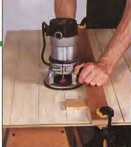
Use a straightedge as a guide to rout the decorative grooves in the plywood back. A spacer block is used to position the straightedge from the marked lines.
