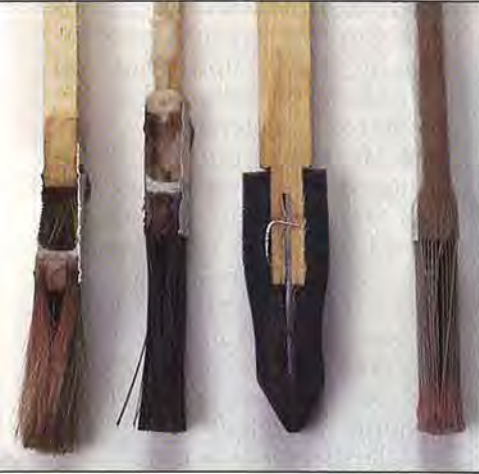
Cutaway views of disposable brushes reveal their low-cost construction. From left, natural bristle, synthetic bristle, foam, and 3M NewStroke.
