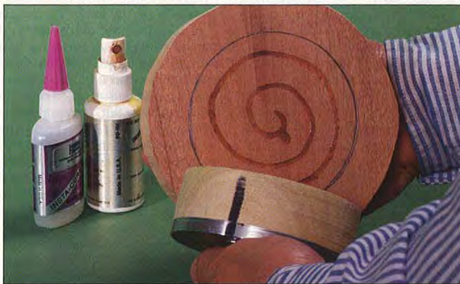
Apply cyanoacrylate adhesive inside the marked circle on the blank. Mist the face of the wasteblock with accelerator, and bring the two pieces together.
