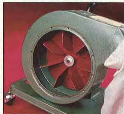
Most dust collectors in our test come equipped with steel plate impellers, as shown above.
