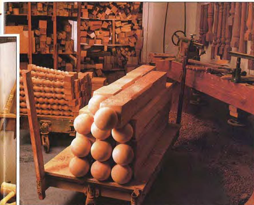
Above: The freshly turned newel posts on the cart are destined for installation on a restoration staircase in San Francisco's Pacifica district. Behind are balusters for a Victorian porch railing.
