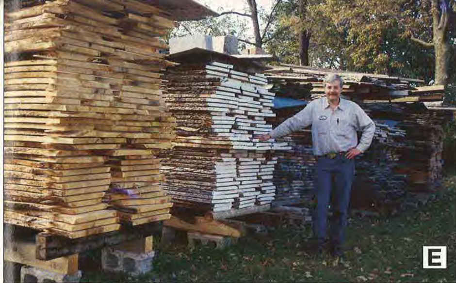
E I stack and sticker the boards in the order they came from the log. Then, I seal the ends with latex paint.
