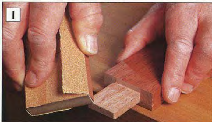
I Sand slight chamfers on the end of the tenon to make it easier to insert the tenon in the mortise. Dry-fit the mating joint pieces and sand the tenon faces or chisel the mortise as necessary.
