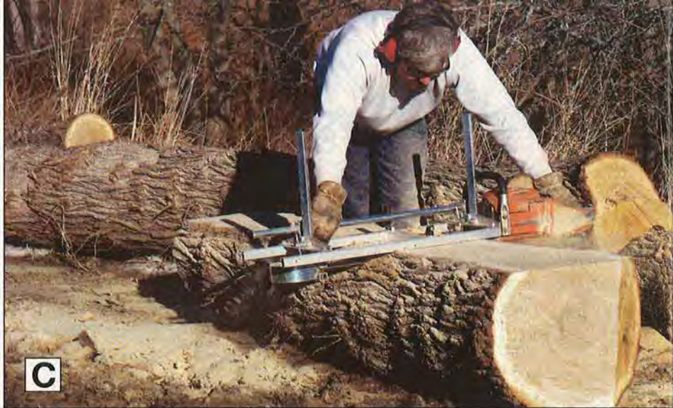
C Above: The flat plane established by the slabbing cut guides the mill through subsequent cutting passes.
