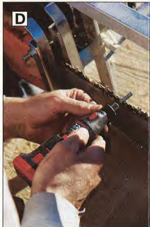
D A battery-powered rotary tool and cylindrical grinding stone help speed frequent sharpening chores.
