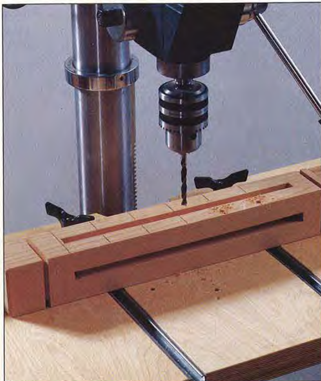
Drill \frac{1}{4} " holes where marked on each leg for the shelf pins. A fence on your drill press ensures alignment.
