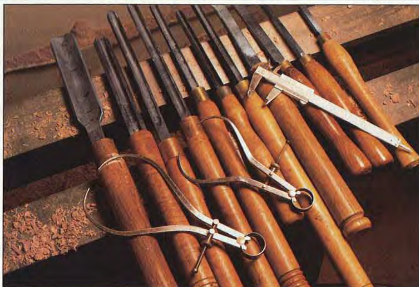
Gail has her turning tools handmade in New Zealand of high-carbon steel. She turns the plain, but hardworking, long-and-strong handles that she prefers.
