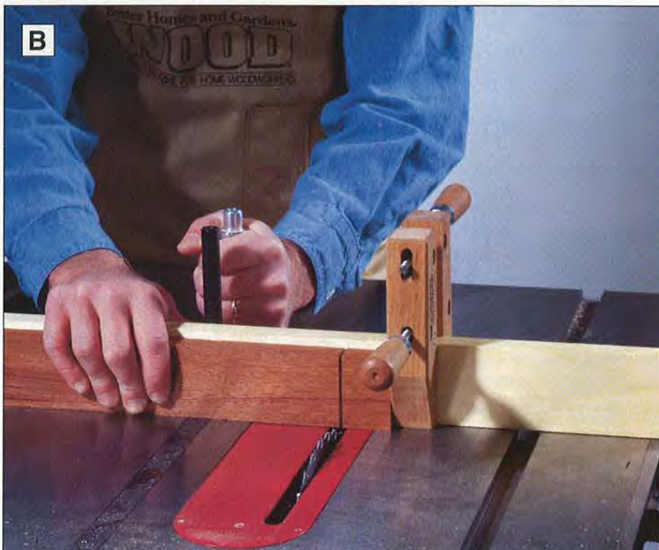
Turn the workpiece on edge, butt it against the stopblock, and cut the tenon setback shoulder. Rotate the piece 180° and cut the other setback shoulder.
