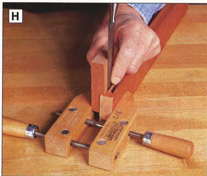
H Clamp the guide block to the workpiece. Keep the flat side of a wide chisel held firmly against the block, and shear the excess wood from the sides of the mortise.
