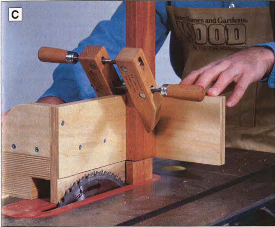
C With the jig cursor set at 1/4" (for a 1/4" cut), clamp the board against the jig fence, and cut the tenon cheeks in your workpiece and in the one side of the guide block.
