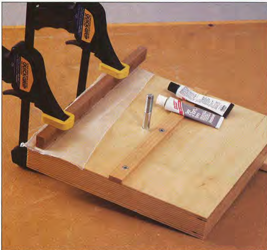
Use a strip of wood, a pair of clamps, and waxed paper to hold the magnets in place until the epoxy cures.
