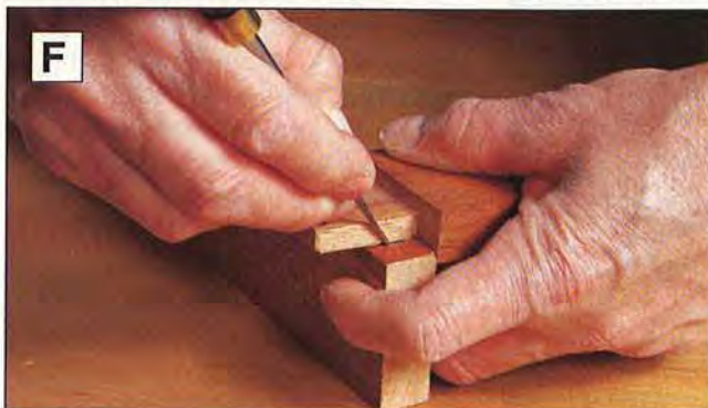
F Position the tenon atop the piece to be mortised, and mark the mortise ends. Be sure to keep the two workpieces flush and square.
