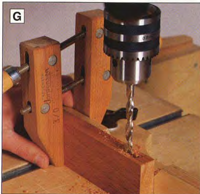
G Using a bit 1/16" smaller than the mortise width, drill a series of holes the length of the mortise. Drill the end holes first and make all holes 1/16" deeper than the length of the tenon.
