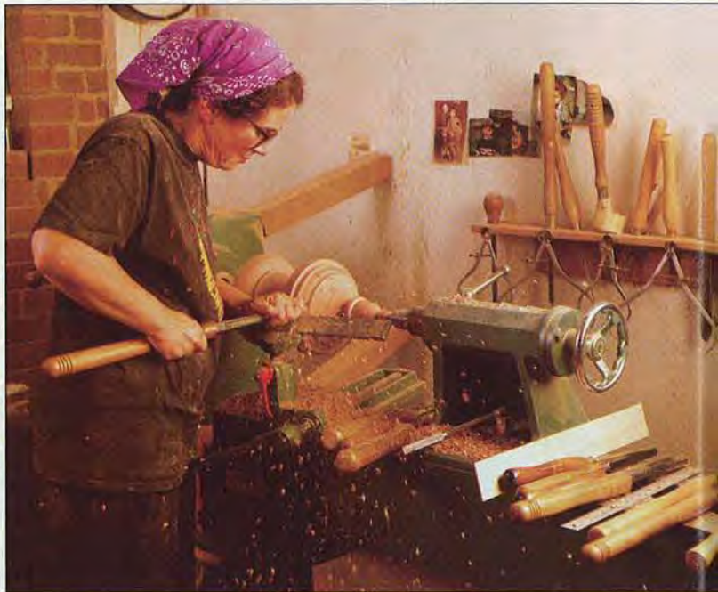
Above: After an elapsed time of 15 minutes since mounting the wood on the lathe, Gail puts the finishing touches on the cedar baluster.
