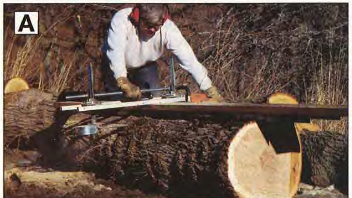
The chainsaw-mill guide controls the initial slabbing cut.
