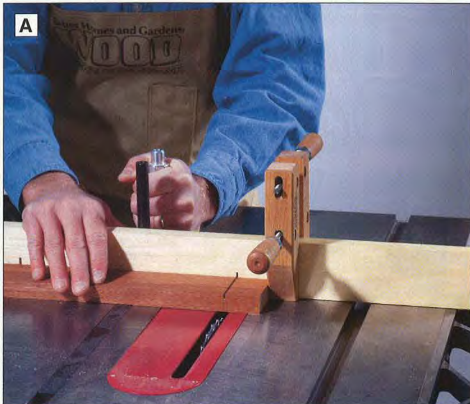
Adjust the saw blade depth, and use a miter gauge with an auxiliary fence and a stopblock to cut the tenon shoulders in the workpiece and one side of the guide block.
