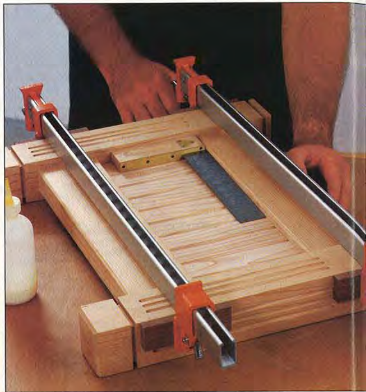
When assembling the planter end frames, be sure to square them as you tighten the clamps. The slats float in the end frame.
