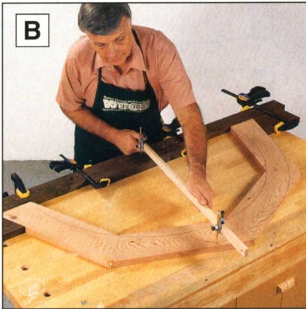
Above: After sanding the glued-together finger joints smooth, use a trammel to mark a pair of arcs on one face of each arched top.
