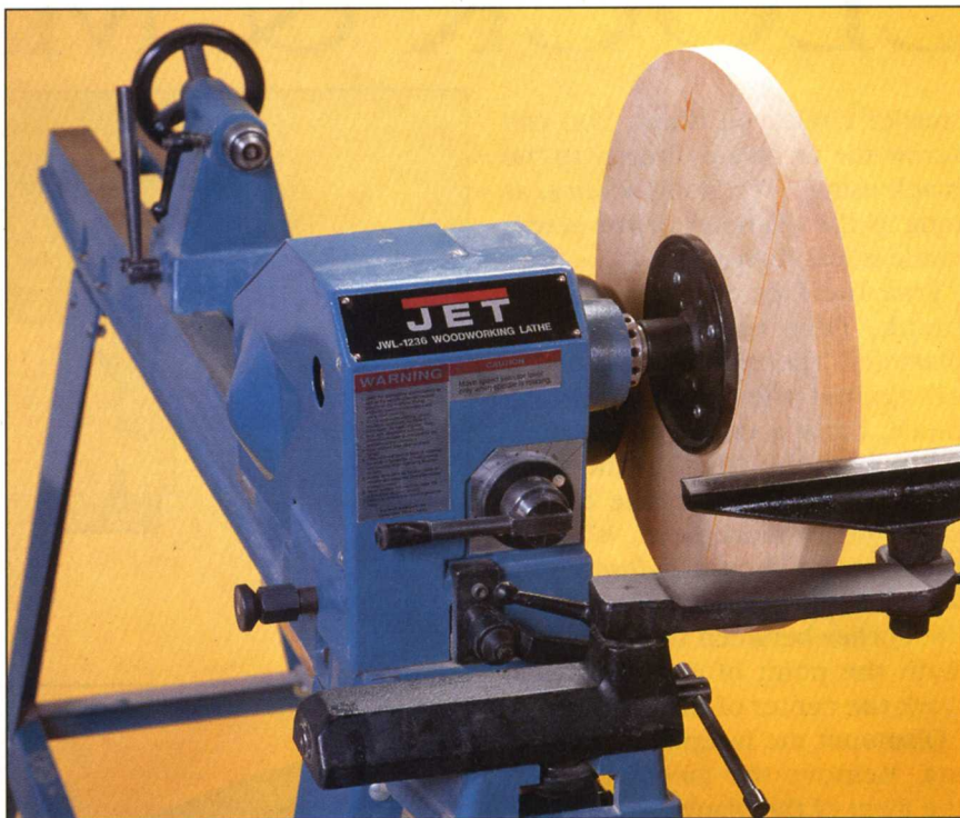
The mirror frame is too large to turn over the bed on most home-shop lathes. The job calls for one that can be set up for outboard turning.
