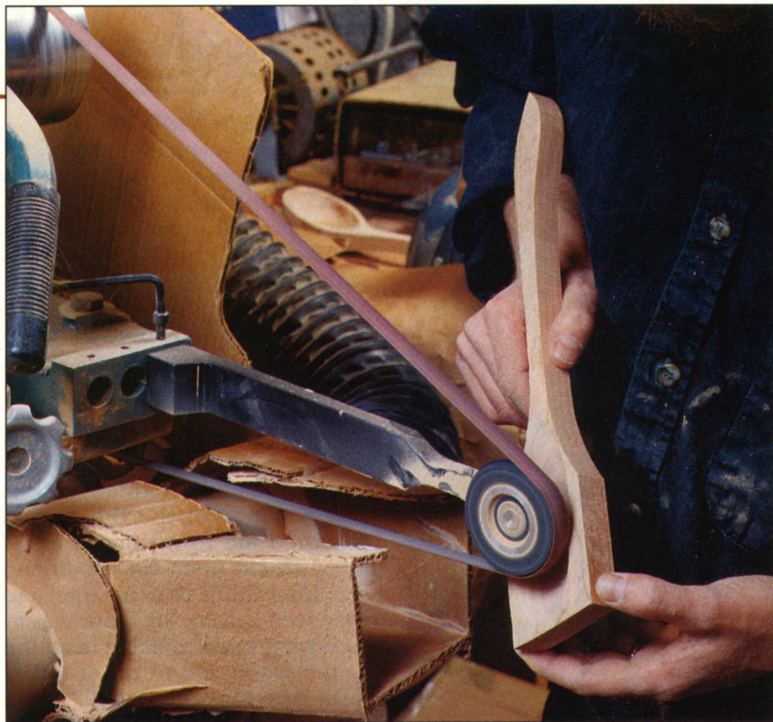
To make the depression in the bowl of a spoon, Jonathan modified a special belt sander. The abrasive of the extra-long belt doesn't clog with sanding dust as easily as a shorter belt.
