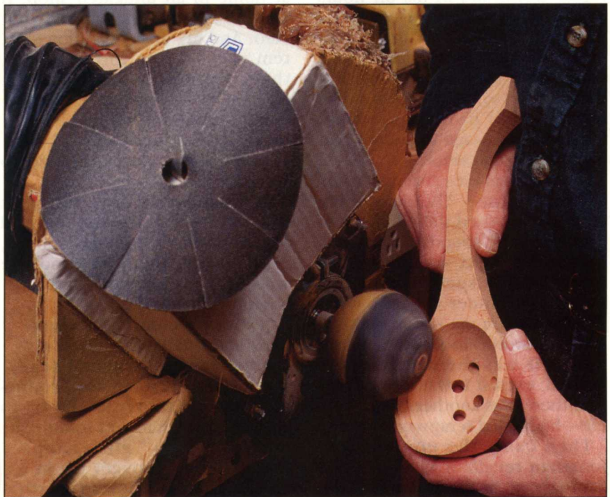
This ladle serves as a strainer, too. A rubber baseball on the sander arbor perfectly fits the ladle's bowl. Hot glue adheres the abrasive disc to the ball.
