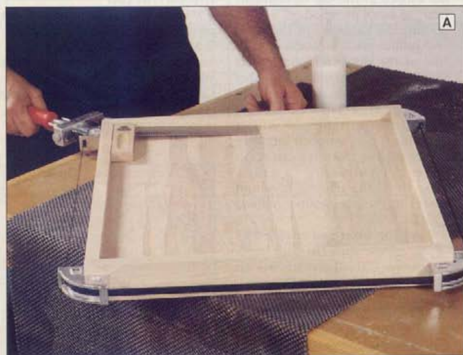
Check for tight miter joints, then glue and clamp the solid maple banding pieces around the plywood center section for the swivel top.
