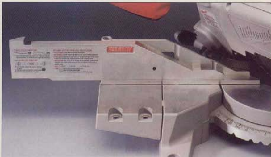
The fence on Milwaukee's 6494-6 extends to a maximum length of 31", the longest of the 10" saws. The left fence can also be reversed, placing the diagonal end by the tilted saw blade for full support when bevel-cutting.
