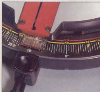
The scale on the Sears model 23514 shows three color-coded degree settings: standard degrees with detent stop locations for basic miter cuts (white), separate crown molding settings (red), and settings for cutting rafters (yellow).
