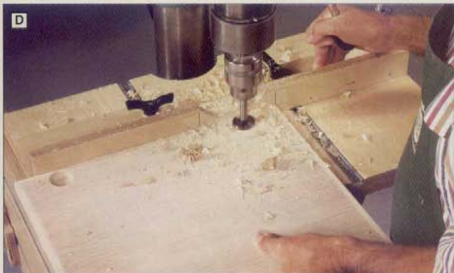
D Mark the centerpoints on the doors, and drill a pair of counterbored holes in the back side of each door for attaching the hinges later. A fence keeps the holes aligned.
