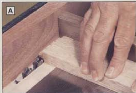
A wood extension secured to our miter gauge minimizes chipout when cutting the rabbets to form the tenons on the ends of the rails.
