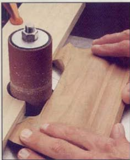
When forming the legs, use a fence with a drum or spindle sander to sand a straight edge and smooth radius.
