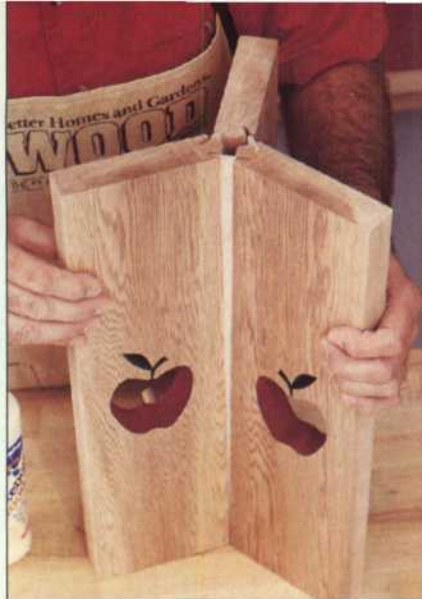
Work from the bottom upward when assembling the splined three-way joint.
