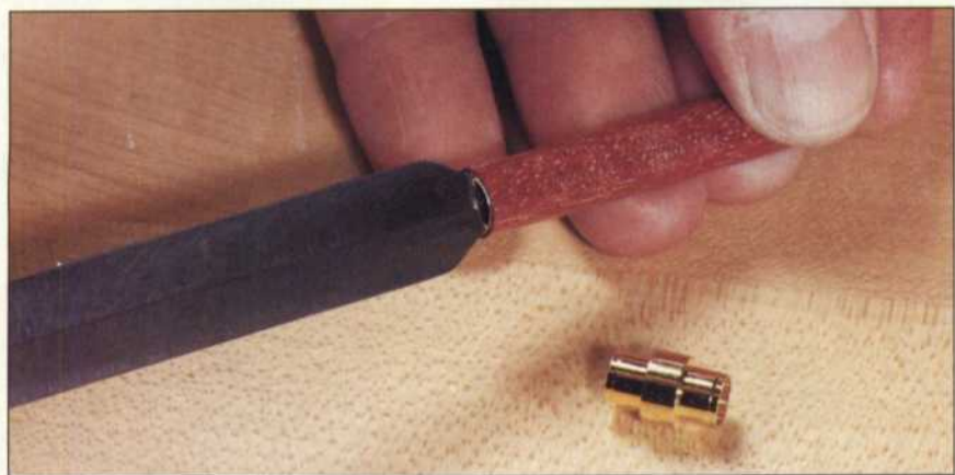
Reaming a slight chamfer on the inside of the tube ends makes assembly easier. A parting tool does the job just fine.
