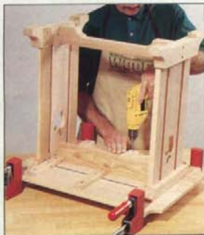
Clamp the top boards together using spacers for even gaps, then screw the base to the bottom of the top.
