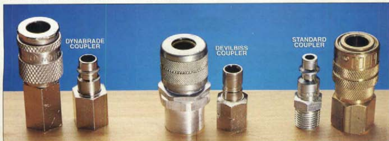
Conversion guns require high-air-flow couplers like those left (from Dynabrade) and middle (DeVilbiss). On the right is a standard coupler. Note the larger inside diameter of the male component of the high-air-flow couplers.
