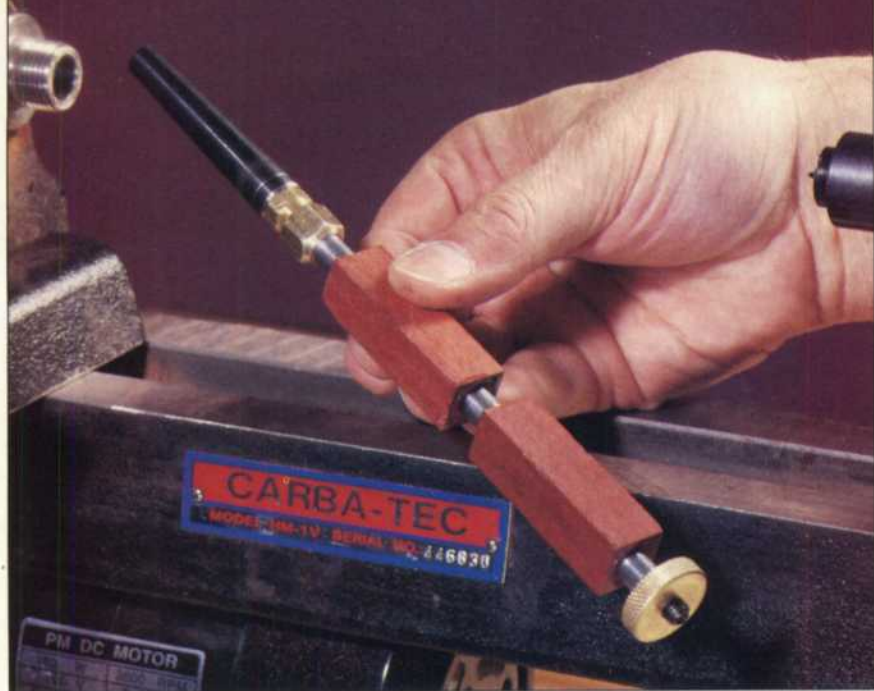
With the blanks and sizing bushings in place and the knurled nut secured, the mandrel is ready to install on the lathe. The brass fitting at the left acts as a sliding stop.
