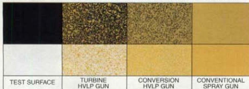
We made one spraying pass on a black and white test surface with three spraying systems to show how well each of them atomizes finishes. HVLP guns do not atomize finishes well enough for auto painting, but they're plenty good for wood surfaces.
