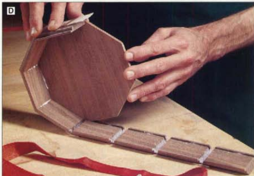
Wrap the taped-together side pieces around the base panel. Use a band clamp to pull the joints tight.
