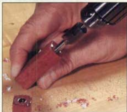
The barrel trimmer pilots in the brass tube to square the ends of the blank to the tube.
