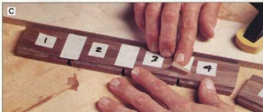
Use a straightedge to align one edge of the base pieces when taping them together at the miter joints.
