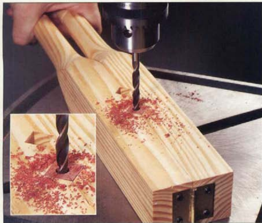
You don't need to precisely center the hole on the end of the blank, but it must run straight and true through the blank.
