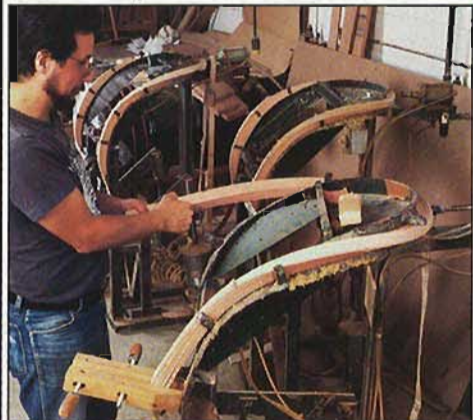
Each continuous arm for a chair is built up of 10 1/16"-thick pieces of cherry. Larry Mosqueda frees the arm lamination from one of the machines that bent it to shape under 20,000 pounds of hydraulic pressure.
