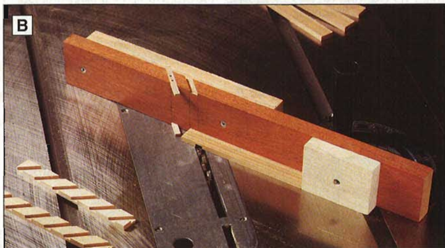
Position one end of a louver side piece against the stop, and make the first cut. Place the angled dado on the index pin, and continue making the cuts until all six dadoes are cut in half of the louver sides. Check the location of the dadoes against the drawing at right.
