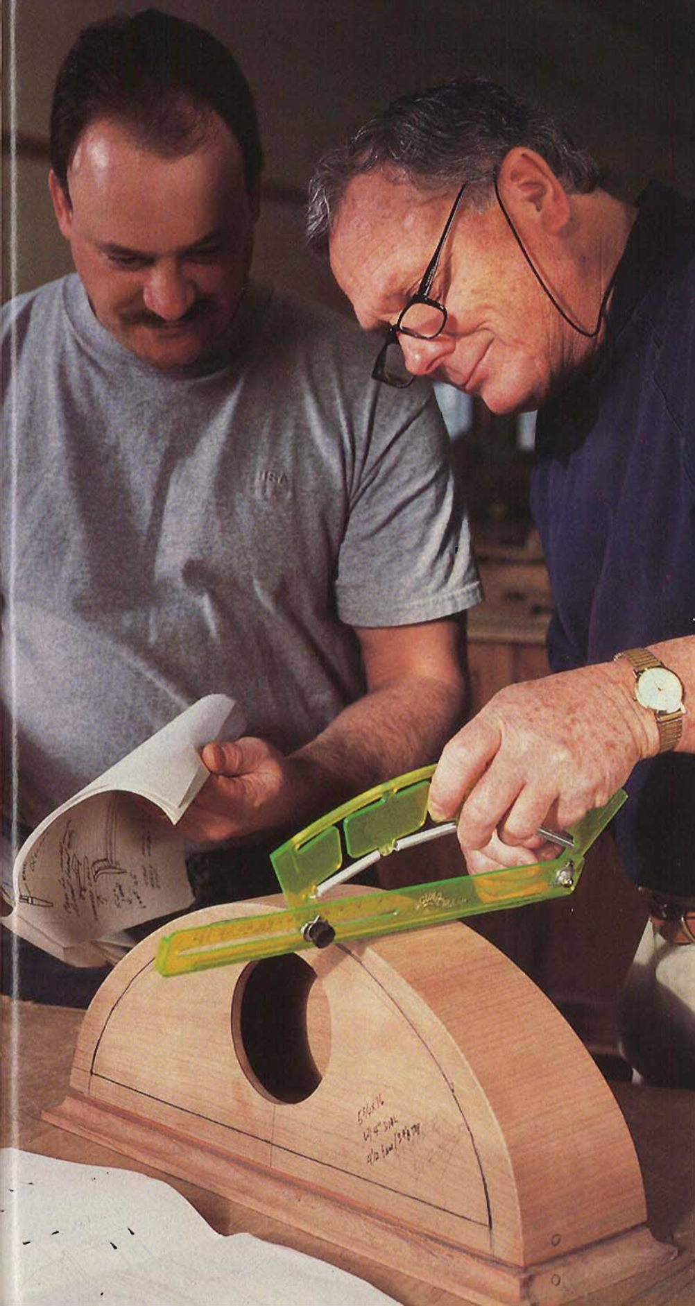
Each continuous arm for a chair is built up of 10 1/16"-thick pieces of cherry. Larry Mosqueda frees the arm lamination from one of the machines that bent it to shape under 20,000 pounds of hydraulic pressure.
