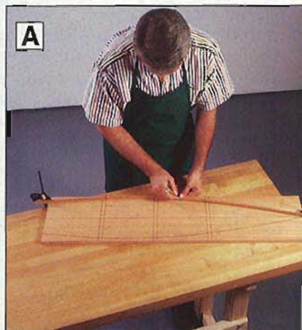
Trace along the inside edge of a flexible strip of wood to mark the curved edges to form the bottom piece.
