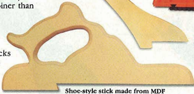
Shoe-style stick made from MDF
