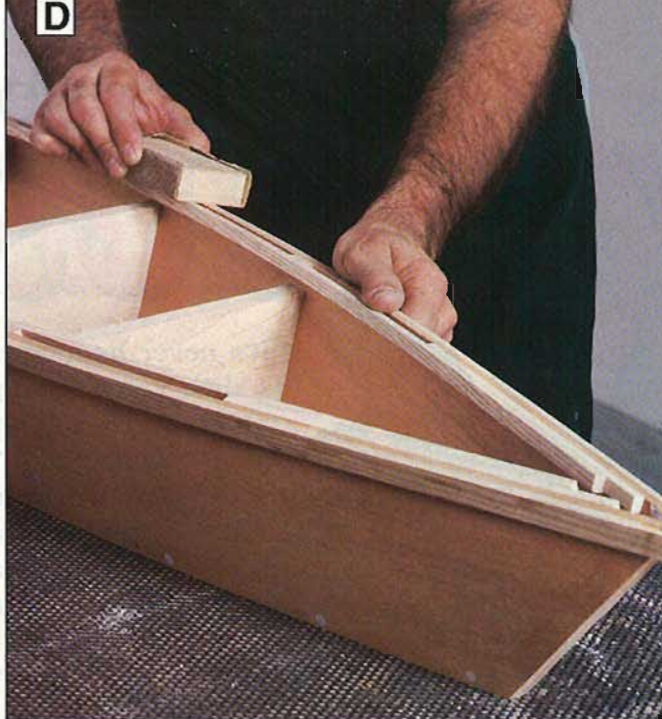
D Use a sanding block to sand the top edge of the gunwale assembly flush.
