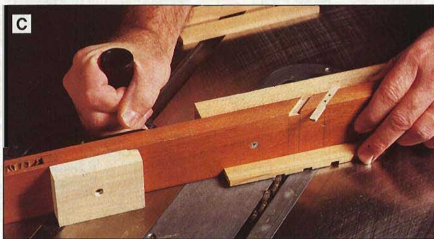
To cut the dadoes in the other half of the louver side pieces, angle the miter gauge 45° the other direction and switch the jig to the opposite side of the blade. Remove the jig from the miter gauge, and put the side that was down in photo B up as shown in photo C.
