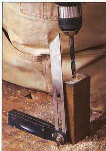
With his drill and a brad-point bit \frac{1}{16} " smaller than the dowel hole, Bob drills out the old dowel.
