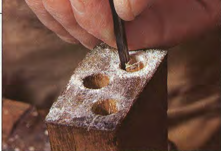
Use a small, dull chisel to remove the remaining pieces of dowel left in the holes.
