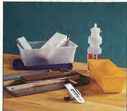
Contain the sharpening mess with a shallow tray, such as a cookie pan. Other useful items include (clockwise from top) a plastic box for stone storage, a water bottle to rewet the surface periodically, a tray for soaking the stones, and a sharpening or honing guide (shown holding a plane iron ready for sharpening).
