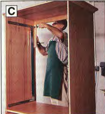
C Locate the top slide's position in the cabinet, drill the mounting holes, and screw the slide in place.
