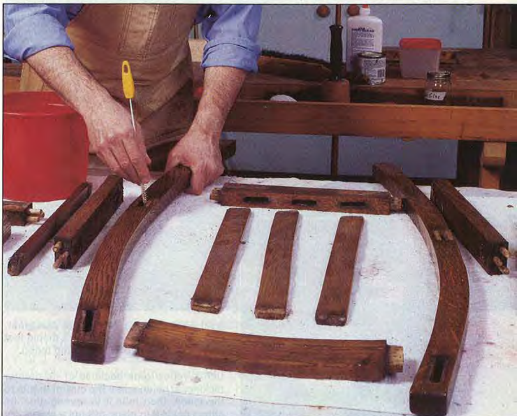
With a kitchen brush, the restorer works water into mortises and dowel holes to dissolve remaining hide glue.
