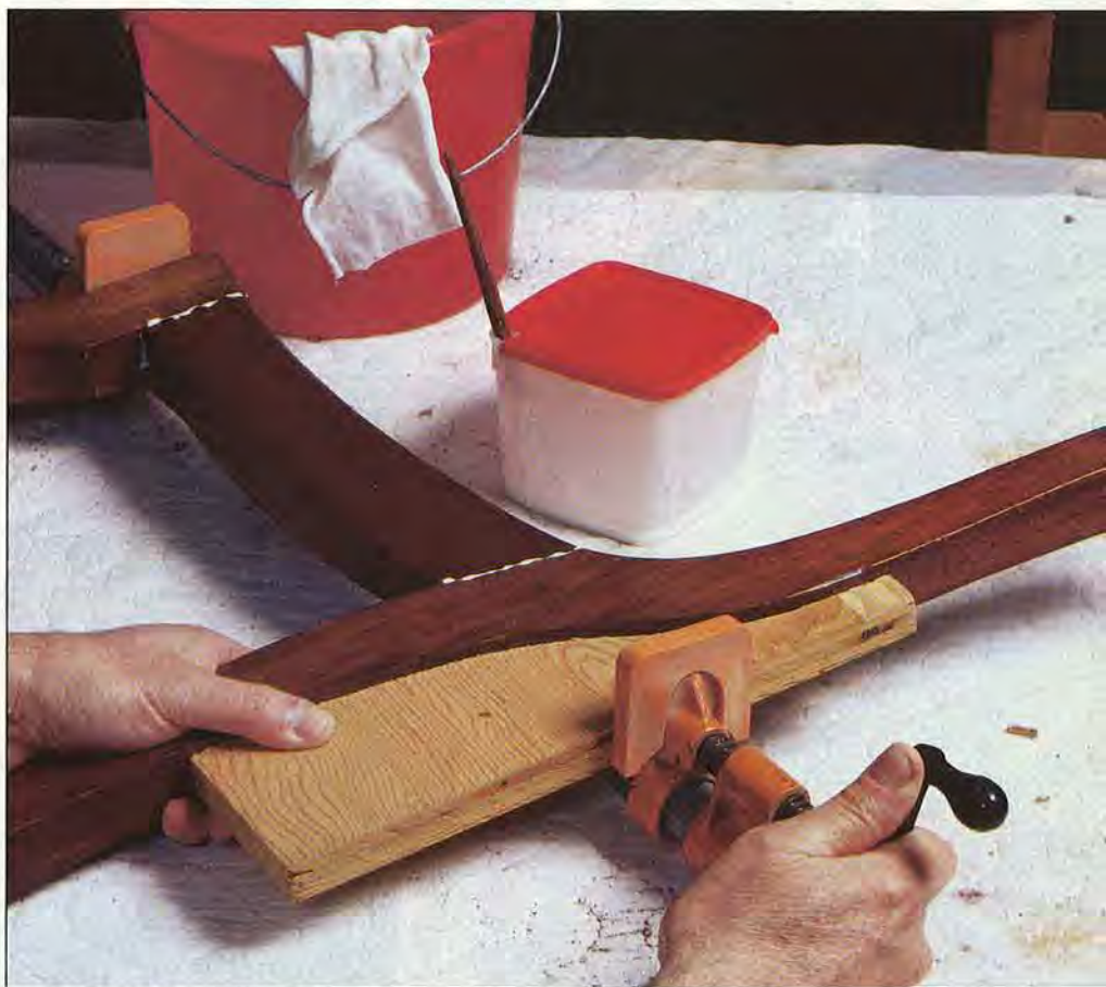
The curved backs of some chairs require a shop-made jig of scrap plywood to achieve parallel clamping when pulling the joints together in reassembly.
