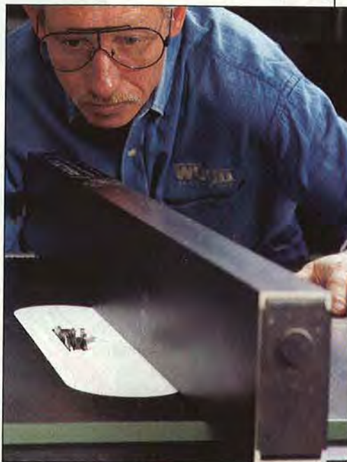
Hold the zero-clearance insert down with your tablesaw fence as you cut through the insert (but not your fence!).
