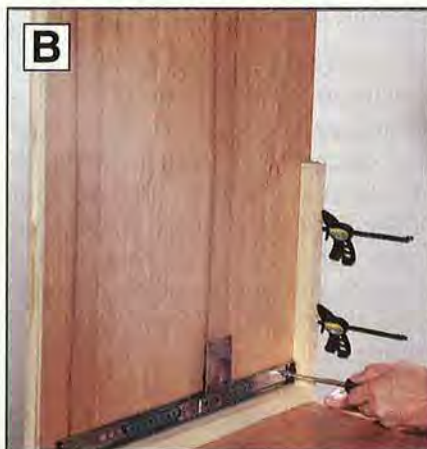
B Use spacers to position the bottom slide where dimensioned on the Section View drawing.
