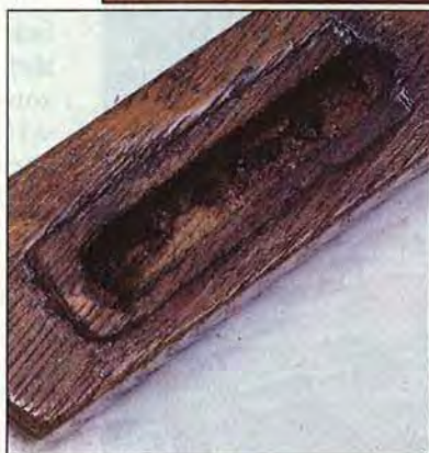
For a good bond, Bob uses a cabinet scraper to take off the aged hide glue from a square tenon.
