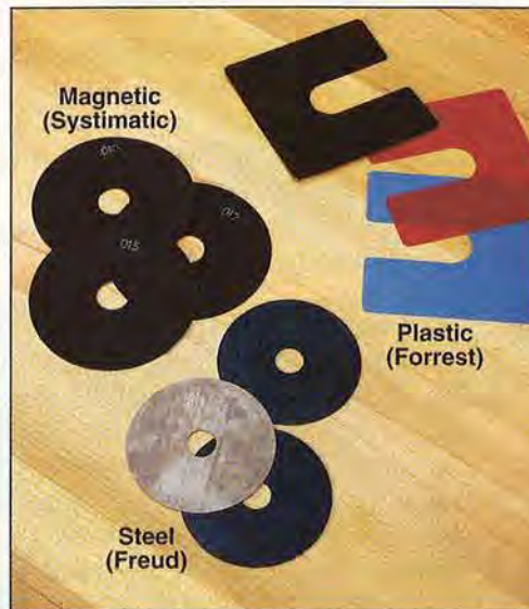
Of the various shims available we prefer magnetic ones for handling ease.
