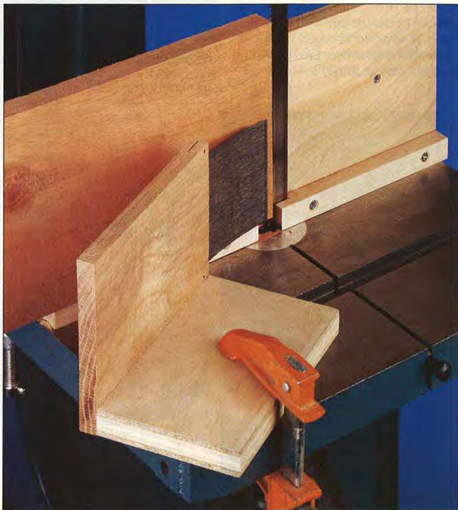
This special feather board uses a small piece of plastic laminate to hold the stock snugly against the fence.
