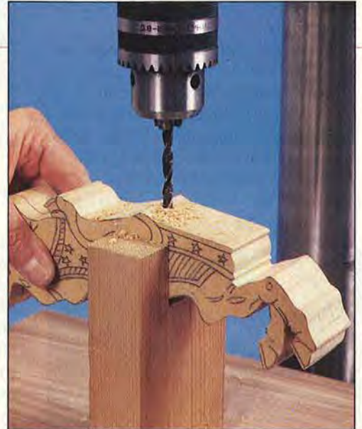
While drilling the body for the pole, steady it with a simple notched block. Keep the body nearly level.
