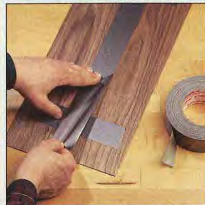
Duct tape makes a great clamp for thin stock. But, if removed before the glue is fully set, it can also pull the joint apart.
