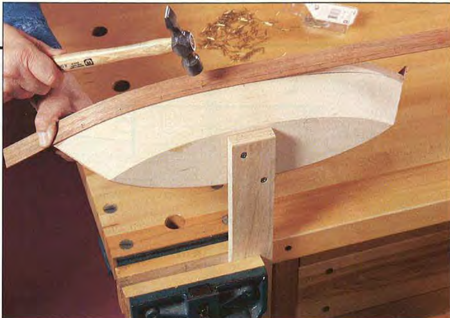
Work from the center outward when nailing and gluing the sheer plank. Align the plank's bottom with the guide line drawn earlier.
