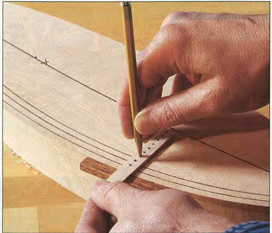
Draw lines for the deck planks all the way to the center line.
