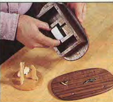
Slide the key shaft up the slot in the spacer block to install the movement.
