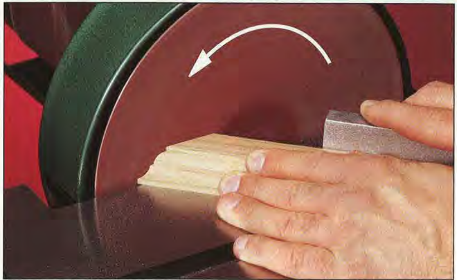
When sizing up a machine, remember that you use only the left side of the disc. So, the actual sanding capacity of a disc is just less than half its diameter.
