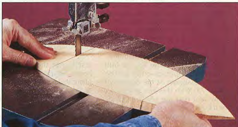
Transfer cabin end lines from the pattern on the other side to the bottom of the deck waste so you can place the flat surface on the bandsaw table.
