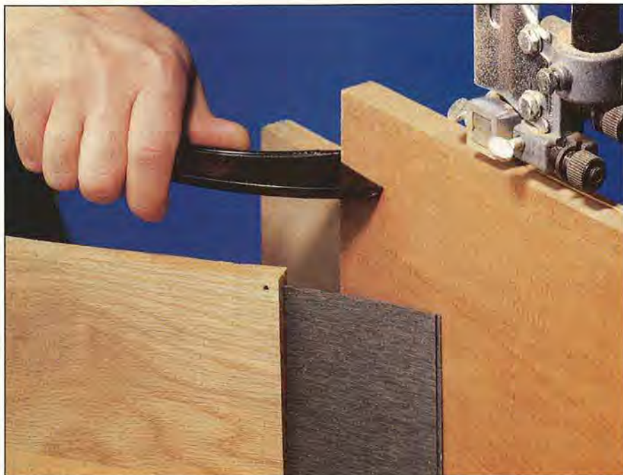
A bandsaw blade can't tell flesh and bone from wood, so use a pushstick to safely complete the cut.
