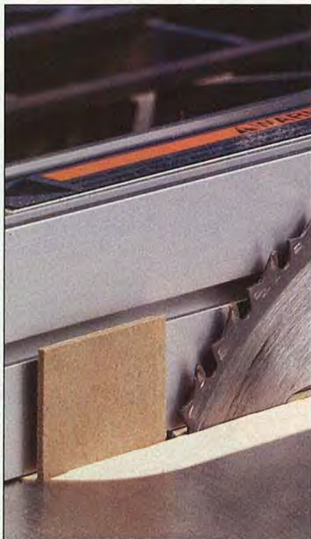
A splitter behind the blade keeps the kerf from closing up and binding while you cut.
