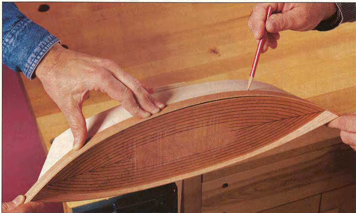
A helper comes in handy when positioning the sheer planks on the hull.
