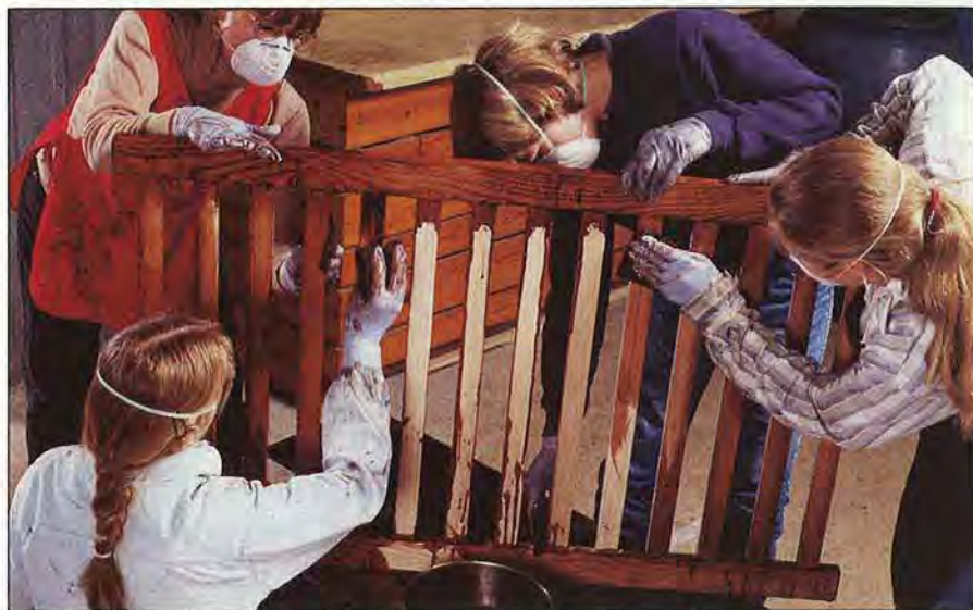
The Schmitt family teams up to apply the first toning coat of a water-soluble dye solution to an oak baby crib built in the Arts and Crafts style.
