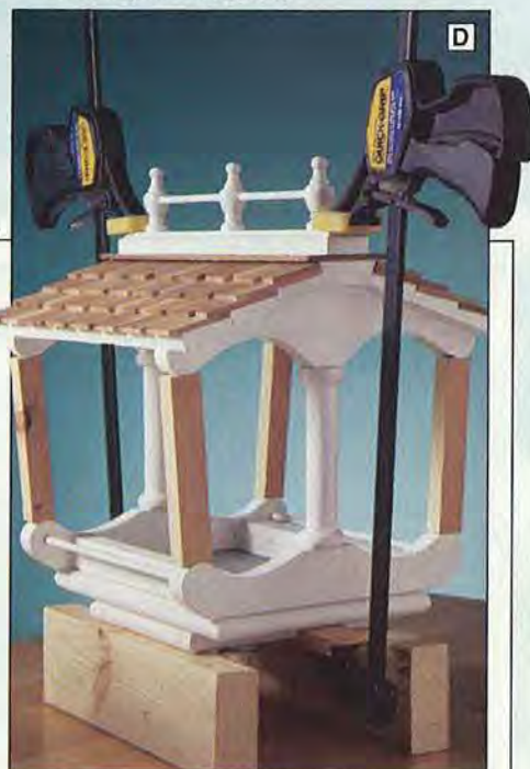
Use four spacers to support the roof when gluing it to the two columns.
