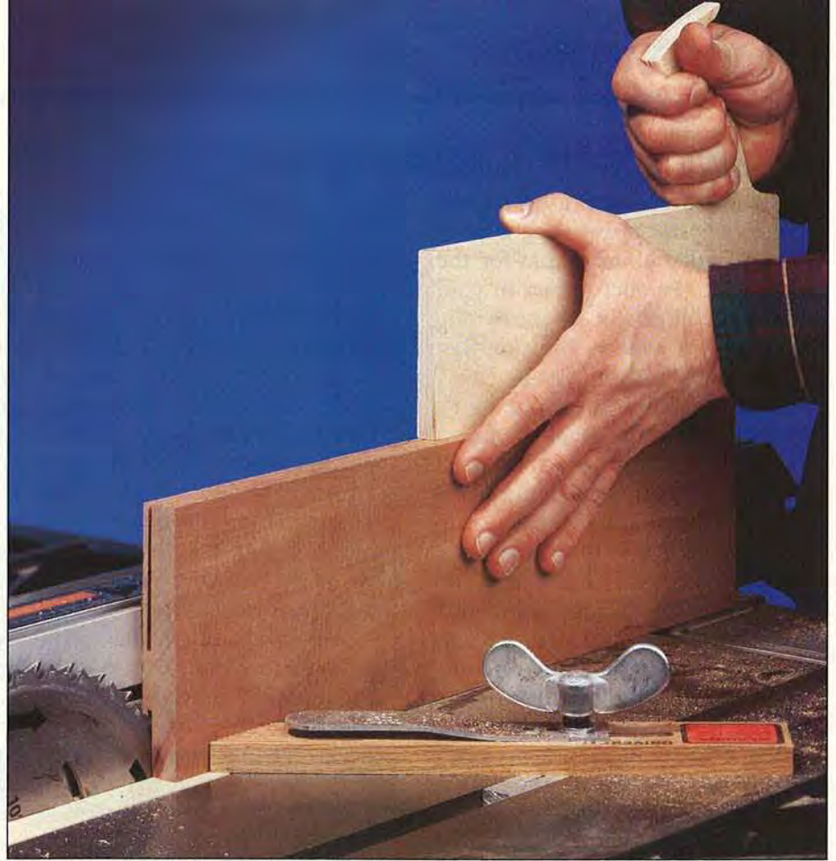
Because the fast-cutting teeth of the saw blade are hidden during the cuts, keep your fingers at a safe distance with a pushstick.
