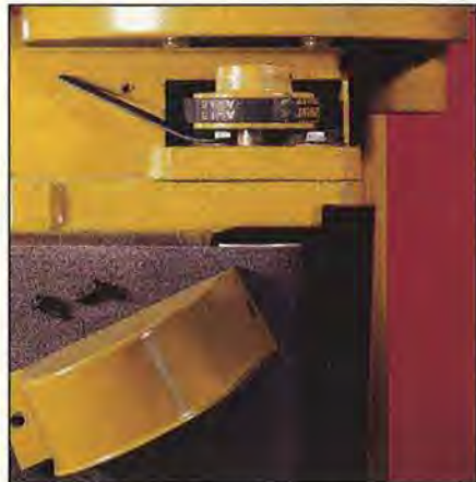
The Powermatic's stamped wrench (shown on bolt) fits poorly, making an already tricky task even more difficult.
