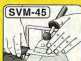
SVM-45 Knife Jig For most knives. Min. blade length 2 3/4". Portable electric hand planer blades. Carvers draw knives.
