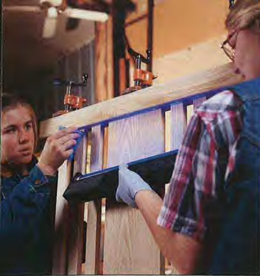
A fluorescent additive in the glue helps Alana and Jennifer spot any squeeze-out as it glows under a black light.
