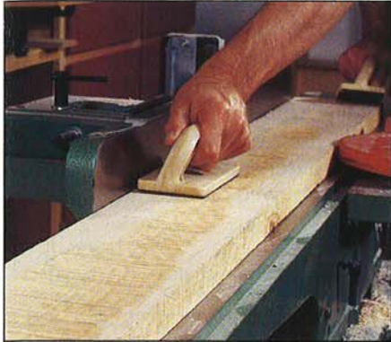
A flat table that requires little sanding begins with flat, face-jointed boards.
