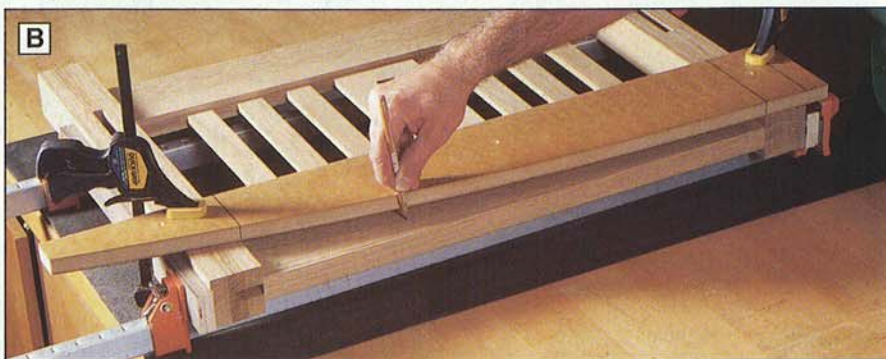
B Clamp one of the template pieces to the dry-clamped (no glue) side frame, and then trace the cutline onto the top rail and leg tops. Repeat for the other chair side.
