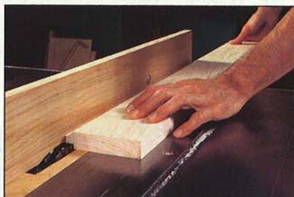
Cut the tongues on the breadboard ends with a tablesaw and dado set.
