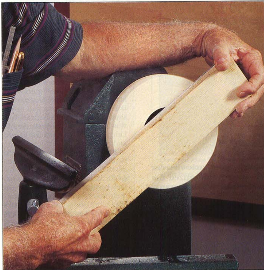
After truing the face of a ring, sand the face flat with a long sanding block.
