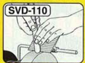
SVD-110 Tool Rest with TORLOCK For turning scrapers. Carving scrapers and inshaves. Screw drivers.
