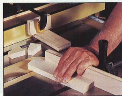
Cut the segments to approximate length and angle on your tablesaw. Install a zero-clearance insert.
