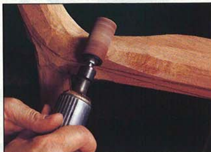
With a die grinder, Robert takes off wood to round the back leg-arm joint. Sanding will later smooth it.
