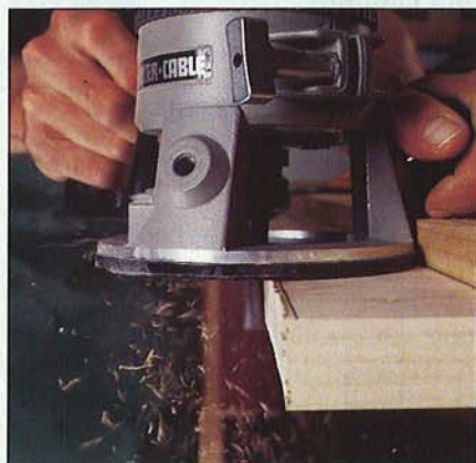
A router, spiral bit, and clamped-on straightedge make for clean ends.
