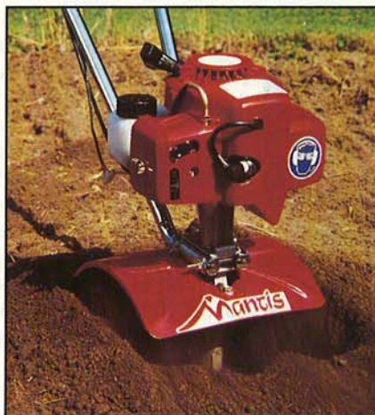
Mantis tines spin at 240 RPM
