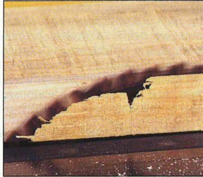
After jointing one edge of each board, rip the other edge. Then, joint the ripped edge, too.
