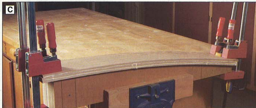
C Clamp the armrest form in a woodworker's vise, and then glue and clamp the armrest pieces against the form.
