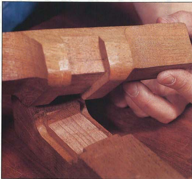
Robert demonstrates the two parts of the sculpted, locking-mortise joint he uses on the seats of his chairs.
