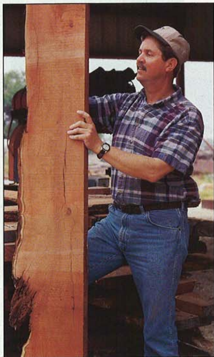
Mesquite, usually not a big, straight tree, yields only about 10 percent clear wood. The typical board Robert holds has a noticeable wind-shake crack.
