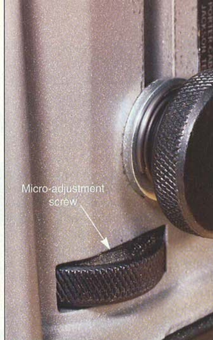
A micro-adjuster, like this one at the base of the Porter-Cable 7310, lets you precisely set the depth of cut.
