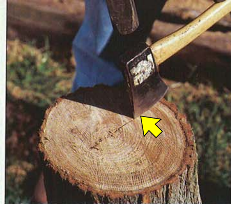
Splitting the wood along existing checks releases the tension created as the wood dries, and also minimizes future checking and splitting.
