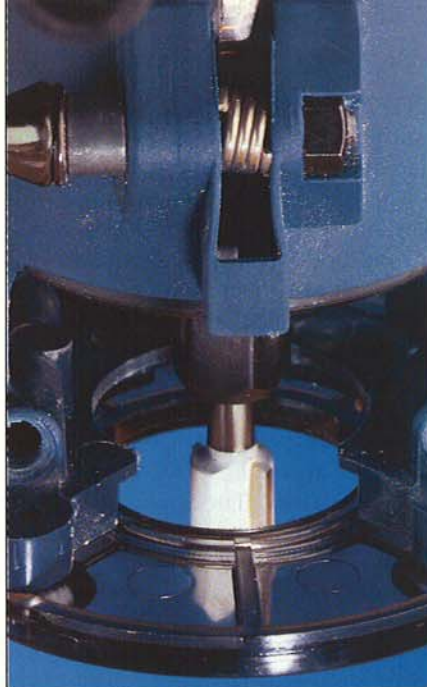
The Ryobi and Sears routers have clear plastic sub-bases that make for excellent bit visibility.
