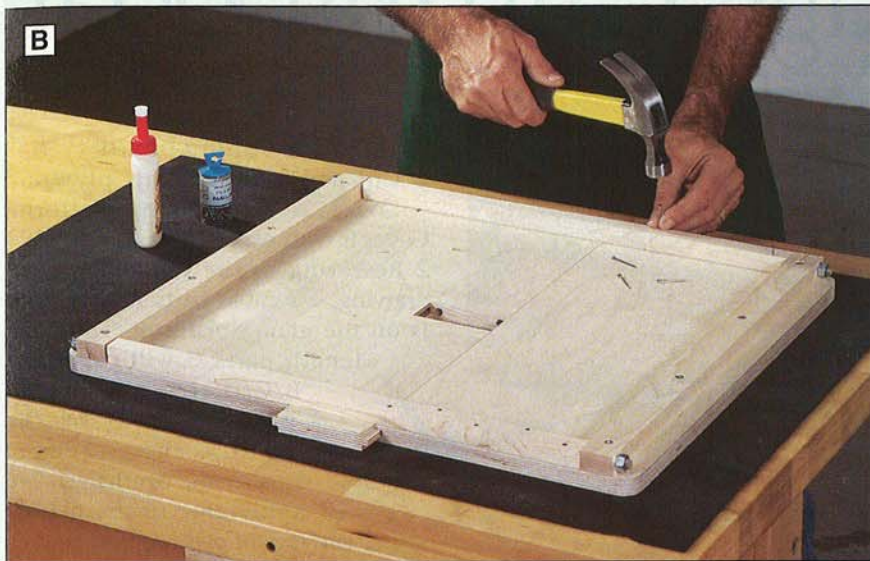
With the tables and spacers upside down, slide the all-thread rod through the clamp blocks and guides to align the pieces. Nail the guides in place.
