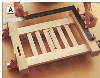
After checking the fit of all the pieces, glue and clamp the end frame, checking for square.
