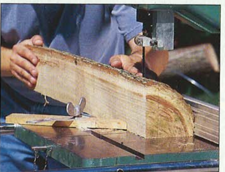
After truing three faces, cut slabs of wood about \frac{1}{4} " thicker than the final thickness you need.
