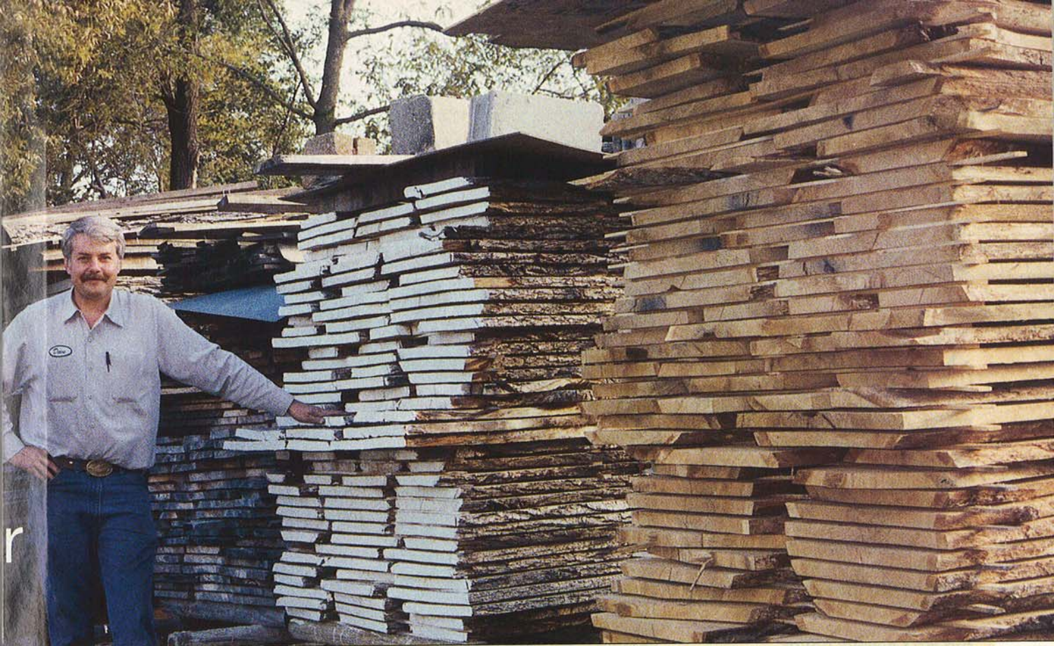
It takes green wood about one year per inch to dry to a level that's suitable for woodworking. This slower method may net you more stock, as you'll see less cracking and twisting. For more about air-drying lumber, see WOOD magazine #97 (June 1997), pages 68-71.
