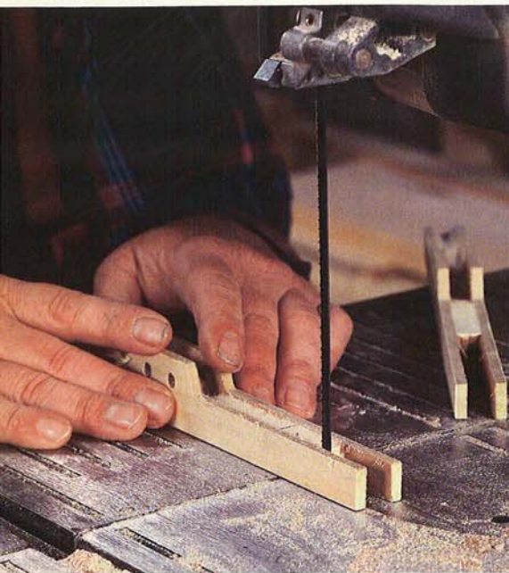
At his bandsaw, Ed cuts out part of a Prentice loader's working boom made of yellow poplar.
