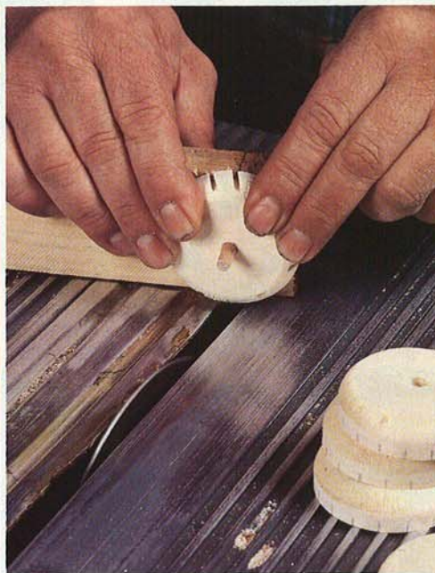
With the miter gauge set at 15°, a jig holds the tires while Ed saws evenly spaced kerfs for tread.
