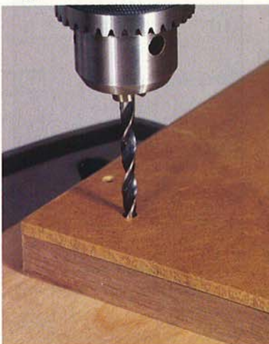
A hardboard template accurately locates the holes for the shelf-support pins in the case sides.
