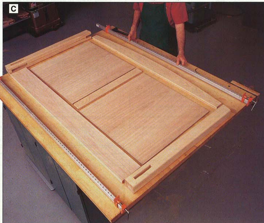
As shown in this bird's-eye view of the dry-assembled headboard, we check the fit of the pieces before gluing and clamping them together.
