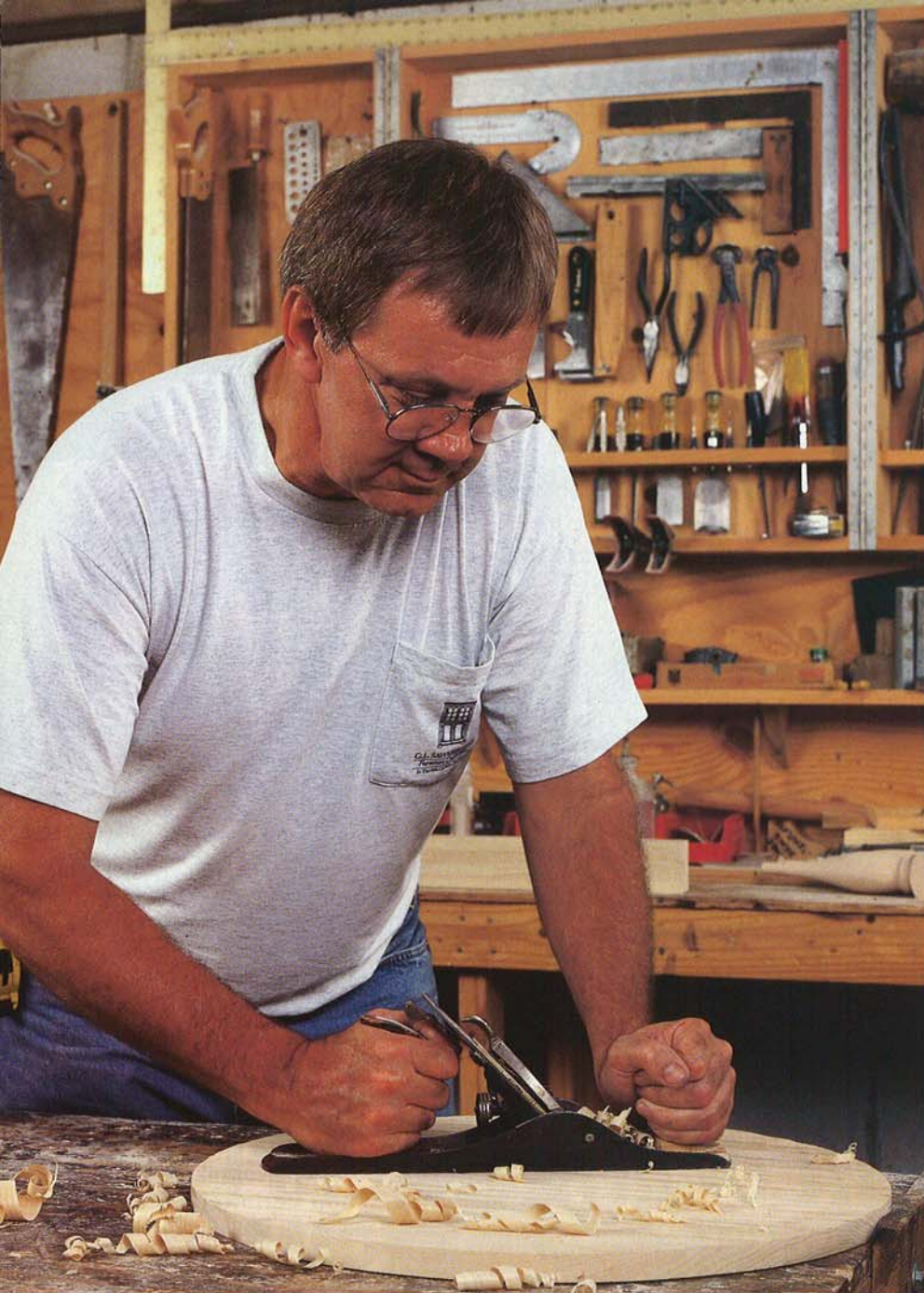
Above: Lee gives a tabletop the wavy look of warp and hard use by making passes with a hand plane fitted with a rounded iron.
