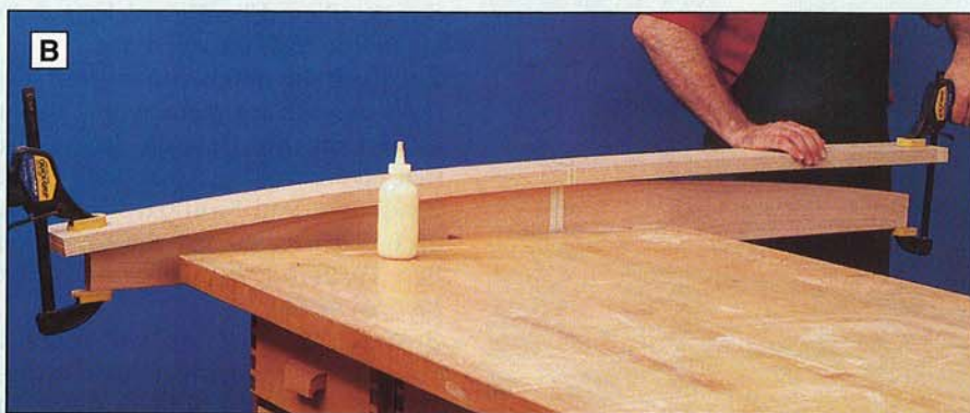
Use the arched headboard top rail as a form to laminate two 1/2" pieces of stock against it to form the curved 1"-thick headboard top cap.
