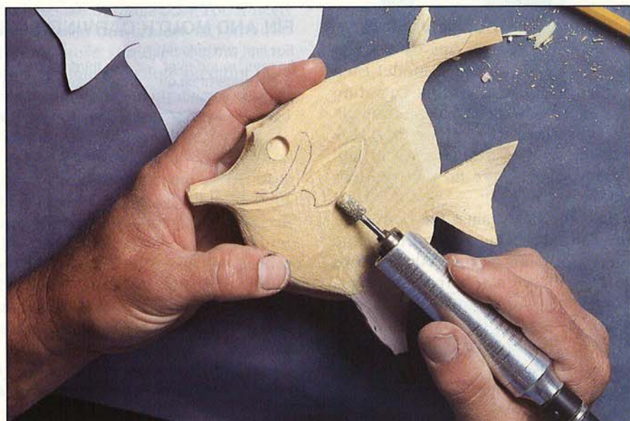
Using a rotary handpiece and carbide burr, Bob carves the detail lines.
