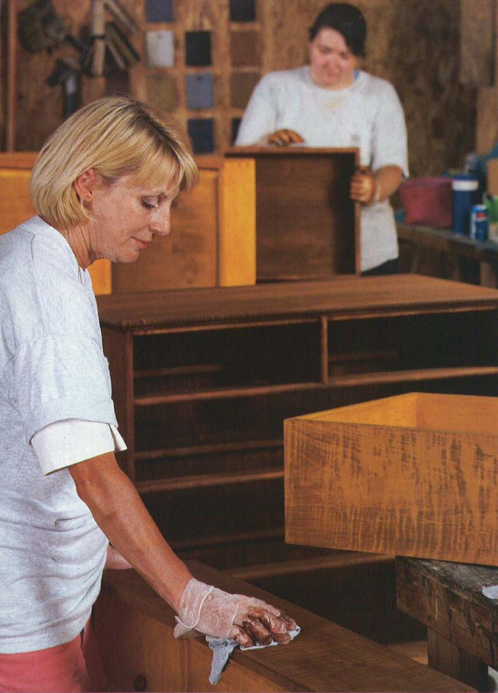
Above: Finishers Helen Borduex and Susan Dunmire add a dark stain over a yellow one to the curly maple drawers of a chest. They'll wipe most of the dark stain off with naphtha, resulting in accented figure and an aged patina.
