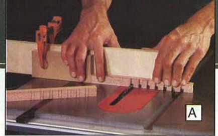
Mark all the cut locations on one post, transfer the locations, and cut the dadoes on the other posts.
