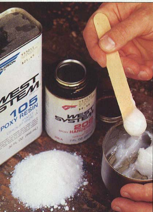
Adding a thickener, such as the mound of silica shown, turns some epoxies from a coating to a strong, paste-like adhesive.
