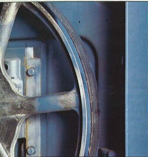
Every bandsaw has rubber tires on the upper and lower wheels that drive and track the blade. Worn rubber spells blade wander and the difficult task of tire replacement.
