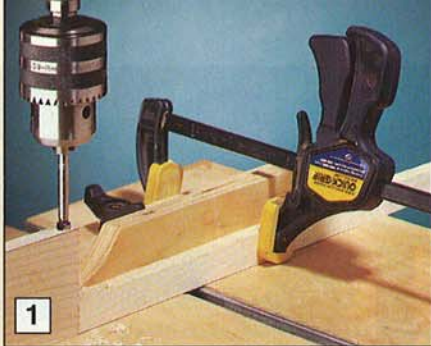
1 A fence and stopblock on your drill press will locate the counterbores and holes in the base accurately.
