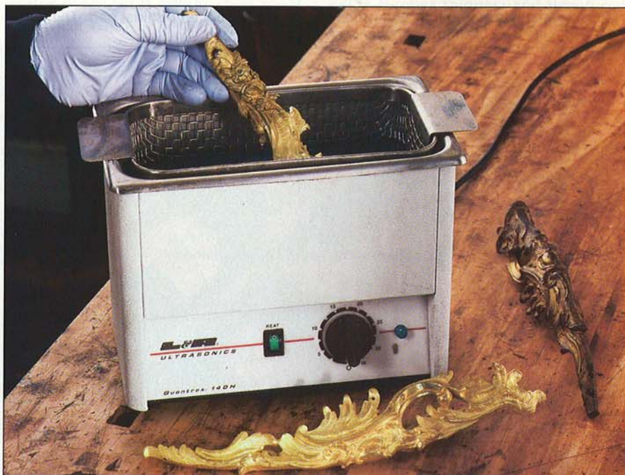
An ultrasonic cleaner provides heat and agitation to clean hardware while you work on other things. Convenience has its price: Dominick paid about $600 for this toaster-size unit (available from McMaster-Carr, 630/833-0300, or online at www.mcmaster.com ).
