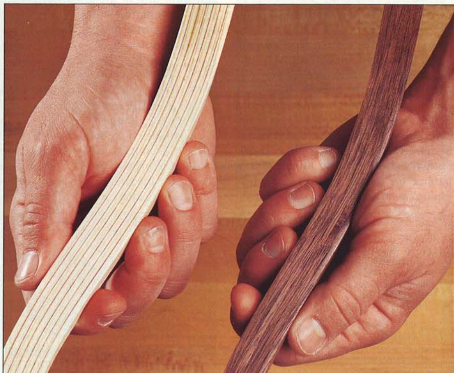
Resorcinol glue lines are virtually invisible in the walnut lamination on the right. However, the dark purple lines can be a distraction, or a stunning design feature, in lighter-colored woods.
