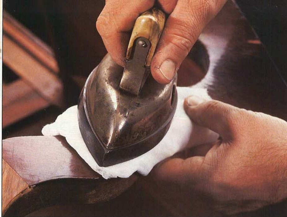
Dominick reactivates the hide glue under loose veneer with a damp cloth and an old iron. Note the newly replaced veneer on the left.
