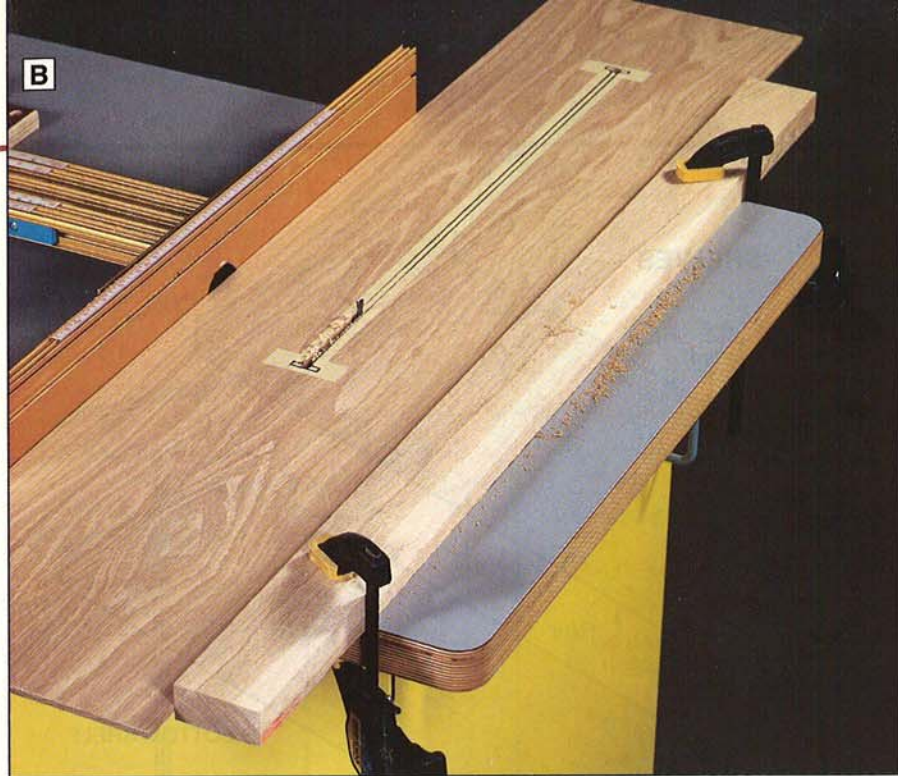
B Position the side-frame panel on your table-mounted router so the \frac{1}{4} " straight bit fits into one of the \frac{3}{16} " holes in the panel. Start the router, and rout to the opposite hole. The double fence secures the workpiece to ensure a straight groove.
