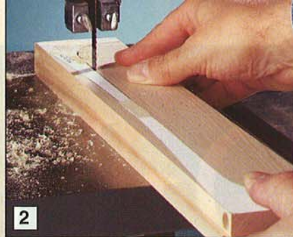
2 Bandsaw both bases at once by laminating the blanks with double-faced tape.
