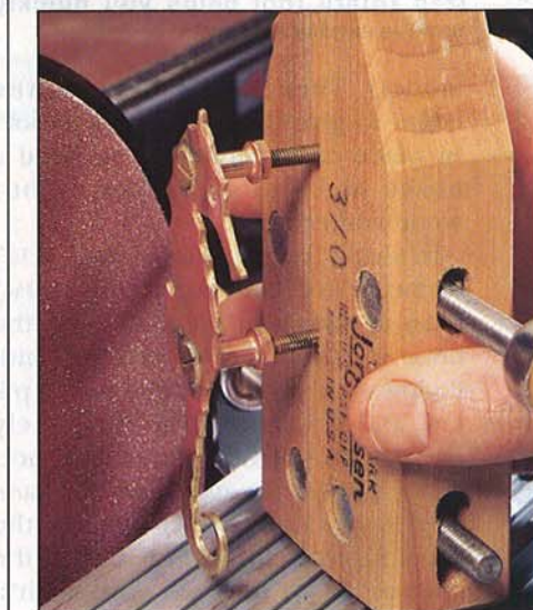
After filing the screw heads nearly flush, you can sand them flush with a disc sander. Use a gentle touch!
