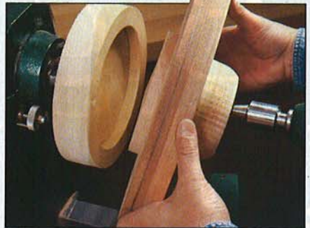
Fit the tenon on the lid into a jam chuck to turn the top surface.
