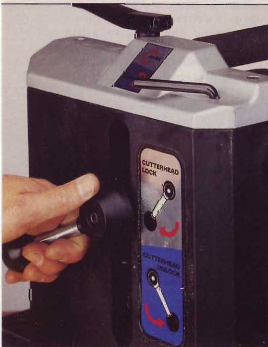
A quick twist of a side-mounted handle locks the cutterhead of the Delta 22-560.
