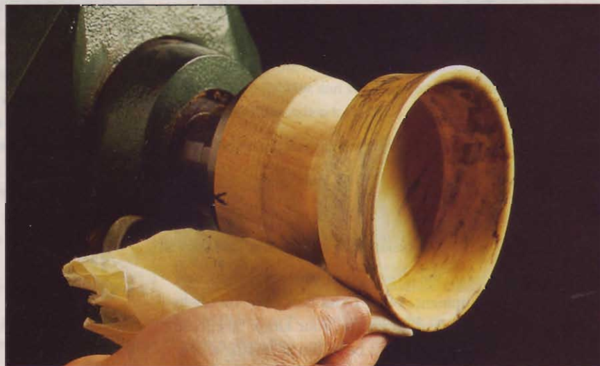
Apply liquid polish with the lathe running, but keep your fingers pointed in the direction of rotation, and don't wrap the cloth around your hand.
