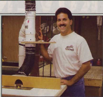
Bob DiTucci's dust collector turns on automatically when he opens a blast gate, thanks to his Top Shop Tip.
