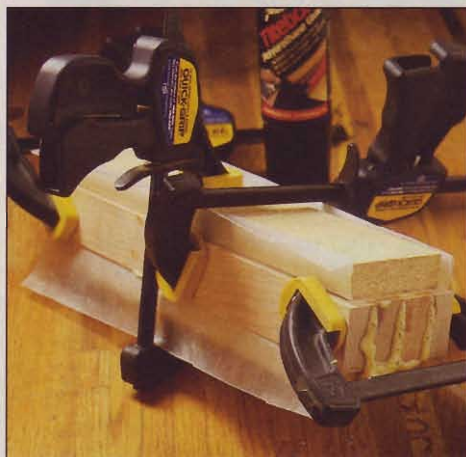
Sandwich the lamination between scrapwood platens to keep the surfaces flush.
