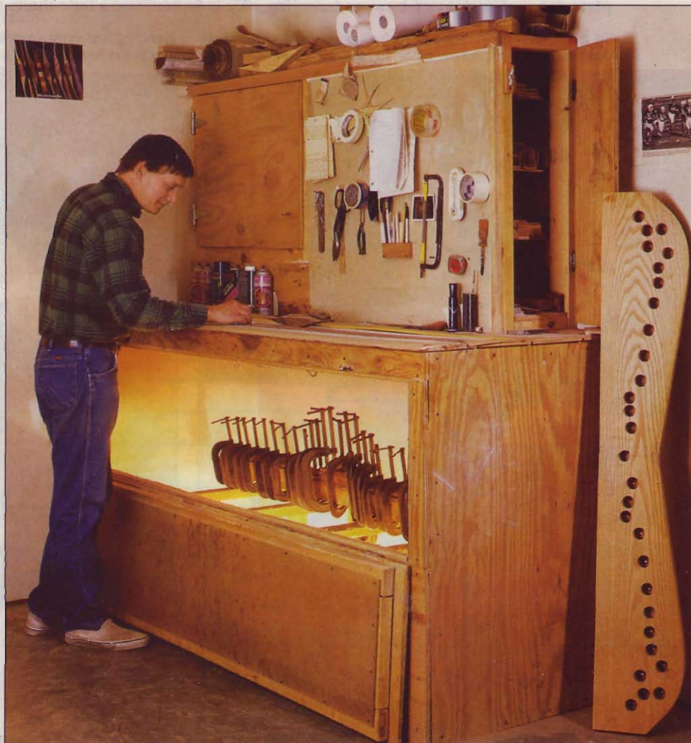
At his workbench, Kent cleans laminations with denatured alcohol before gluing them up. In the heatbox below, a glued-up bow clamped to its form awaits removal.
