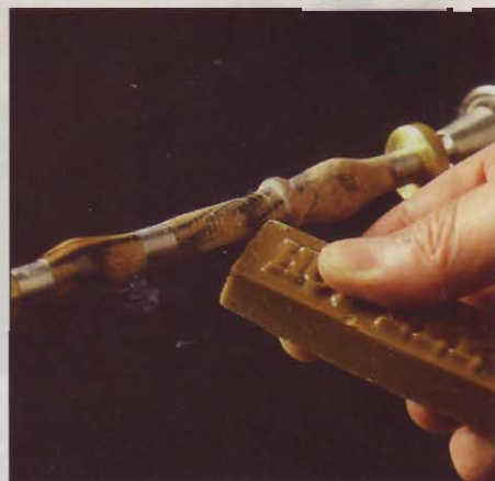
HUT finish polishes out sanding scratches, making it a particularly effective finish for acrylic-stabilized burl like these turnings. Compare the polished and buffed part at far left with the unfinished end at far right.
