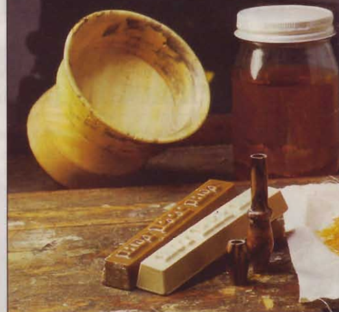
Shellac, denatured alcohol, and boiled linseed oil make an easy-to-apply finish for bowls and other small turnings. HUT Wood Finish sticks, left front, are ideal for small spindle turnings and pens.
