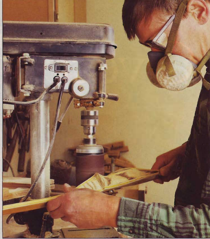
At his drill press, the bowyer further refines the shape of the bow's risers and limbs with a drum sander.
