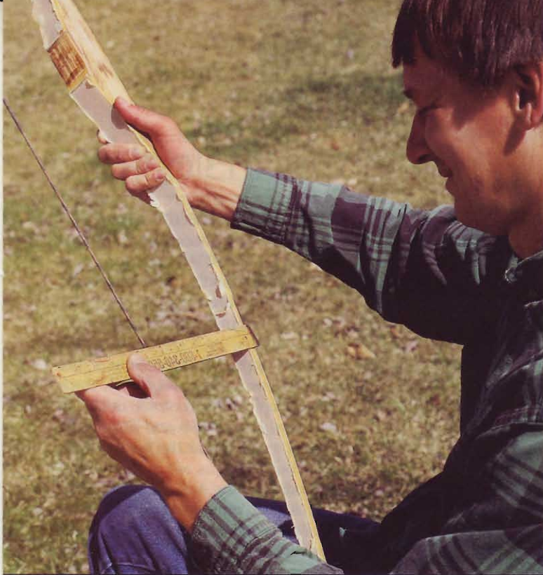
During sanding, constant measurements between the strung bow's limbs and string tell Kent how close he's coming to the draw weight.
