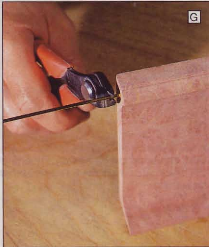
Brass or bronze brazing rod makes for sturdy hinge pins. Nip the pins so they stick out \frac{1}{8} " from the lid.
