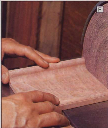
Lightly touch one end of the lid to a disc sander to reduce its width by about \frac{1}{64} " uniformly along the end.
