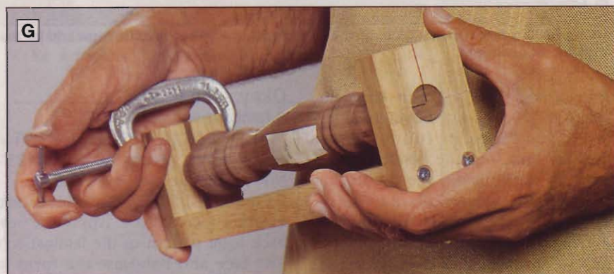
G Align the appropriate mark on the leg's bottom end with the jig's vertical line, and clamp the opposite end in place.
