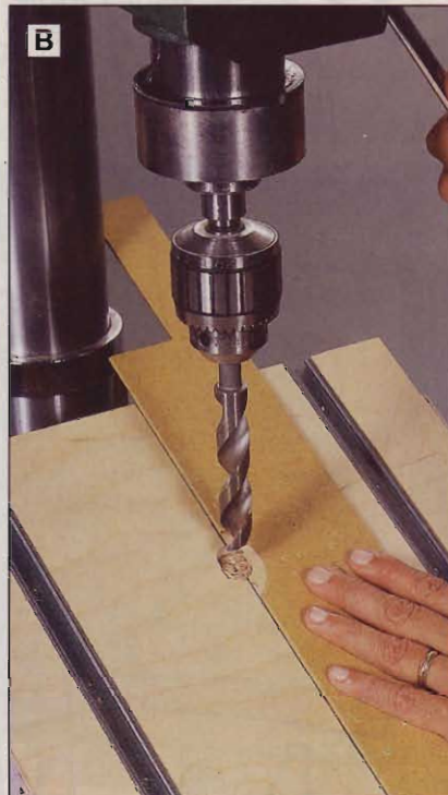
Use the column alignment gauge to locate the drill-angle jig prior to clamping it in place.
