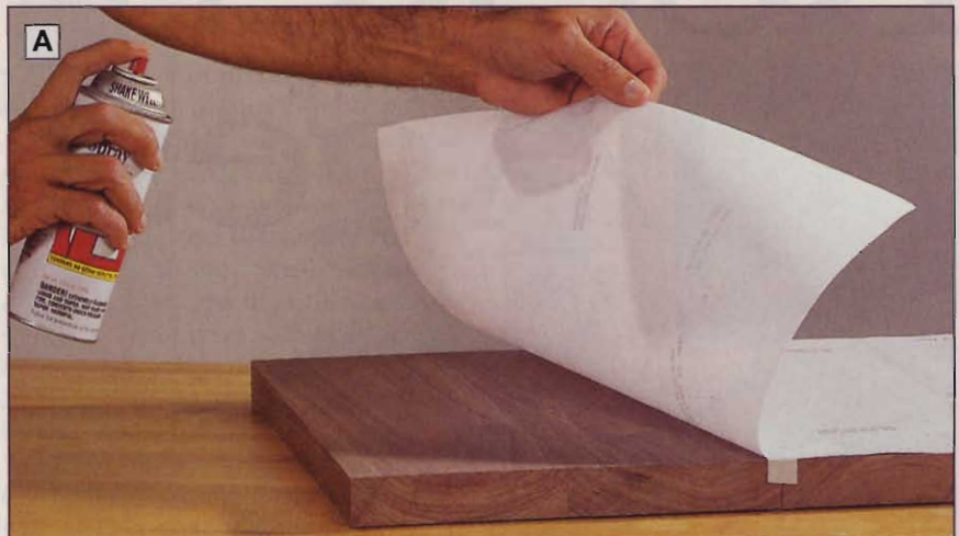
Center and align the top and bottom patterns along the front edge of the seat blank. Tape them in place at the centerline edges; then spray-adhere them to the seat as shown, smoothing out any wrinkles.
