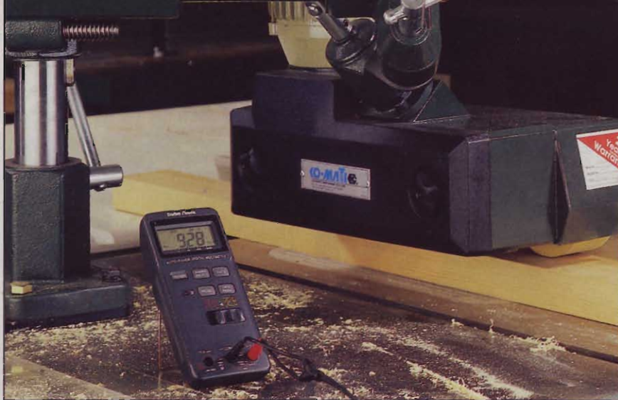
To evaluate how easily each blade cut, we used a Comatic power feeder (Sunhill Machinery, 800/929-4321) to rip thick pine boards at a constant rate, and measured the saw strain with a multimeter.
