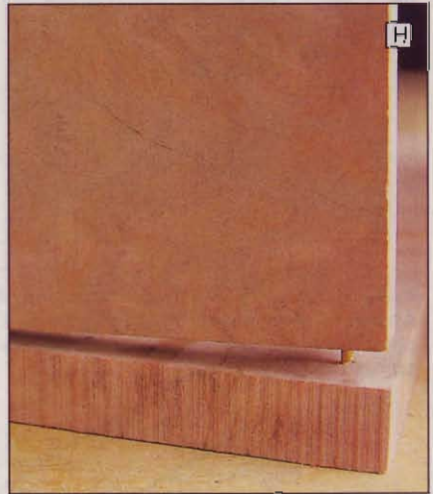
Use the hinge pin already placed in the lid to mark its matching location on the side pieces.
