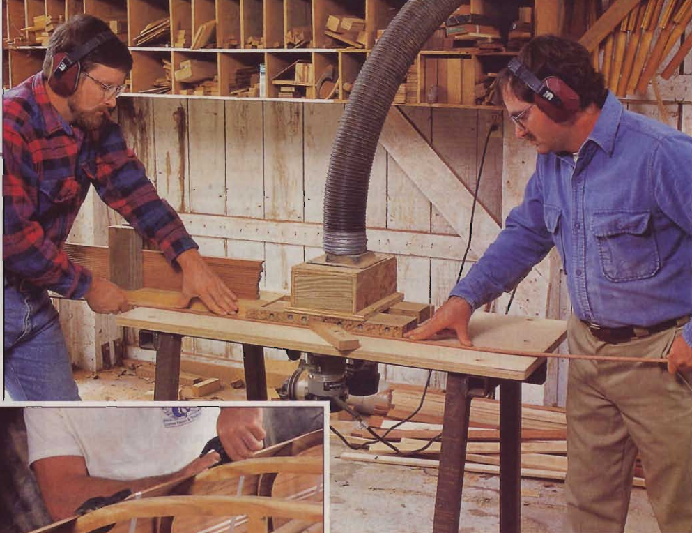
Above: At the shop's double router table, Phil, left, and brother Tim shape bead-and-cove strips for a canoe hull.
