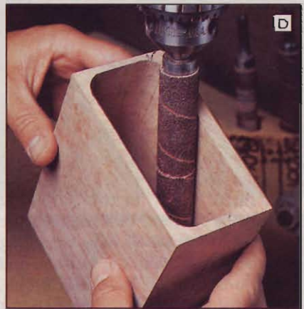
A sanding spindle with an aggressive abrasive, such as 50-grit, quickly smooths out the bandsaw blade marks.
