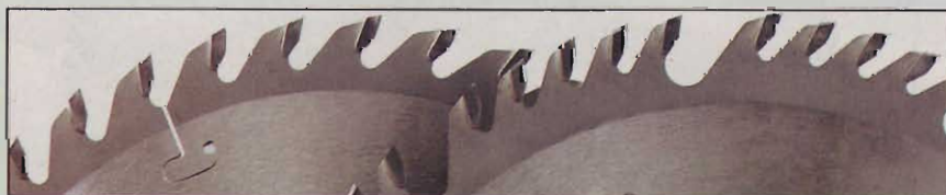
Deep gullets, each followed by a raker tooth and four ATB teeth, distinguish a combination blade (foreground) from a general purpose blade (background), with its evenly spaced ATB teeth and consistently deep gullets.
