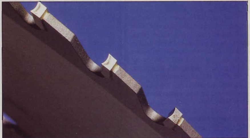
Craftsman's "Razortooth" (on the Professional C300 blade) sports a curved face so each tooth does twice the work of one ATB tooth.
