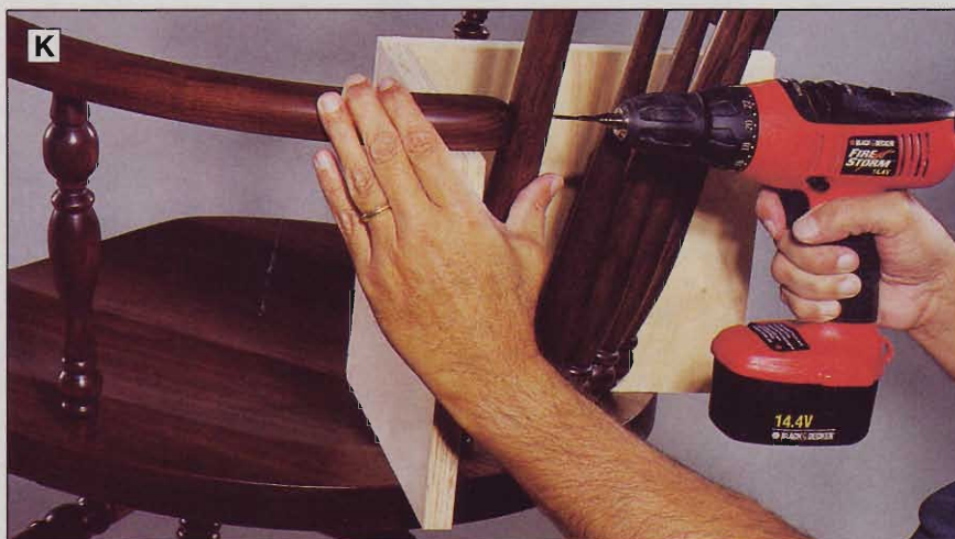
Rest the armrests on a right-angle spacer, and drill the countersink/counterbore holes with a portable drill.
