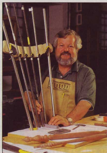
Jim Downing verifies the hole angles for the seat-back spindles and back splats. With this project, angles are everything.
