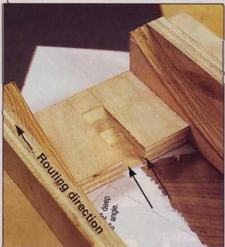
As you move the jig around the seat, align both corners of the exit ramp along the pattern line, as indicated by the arrows. Place the jig so you cut with about two-thirds of the bit's width.
