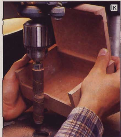
Use a spindle sander to make a 1"-long finger recess along the bottom front edge of the box.
