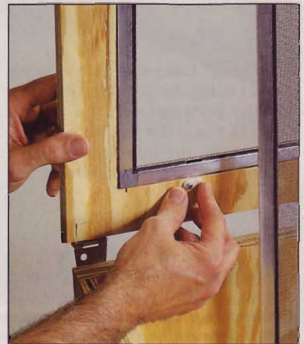
Nylon turn buttons hold the interchangeable inserts in the lid. You can also glaze the lid directly with a piece of clear acrylic sheet.
