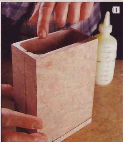
Prevent squeezeout on the inside of the box by wiping the glue bead away from the inside edges of the lid and bottom.
