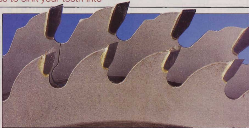
You'll get more sharpenings out of the background blade because the teeth have more carbide to grind.
