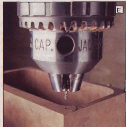
Use a #53 bit to drill the hinge-pivot holes into both ends of the box blank. Stabilize the bit with stop collars.
