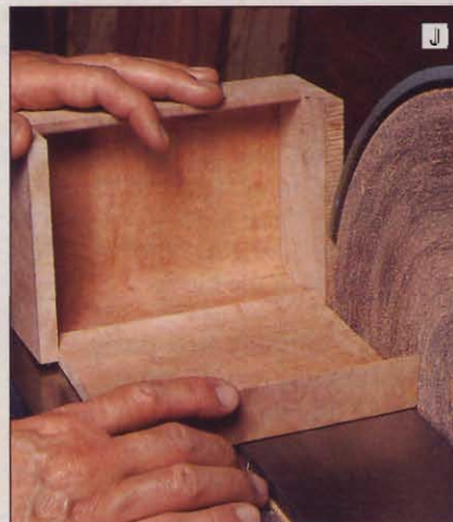
Use a gentle touch with a disc sander to equalize the gaps between the box lid and sides.
