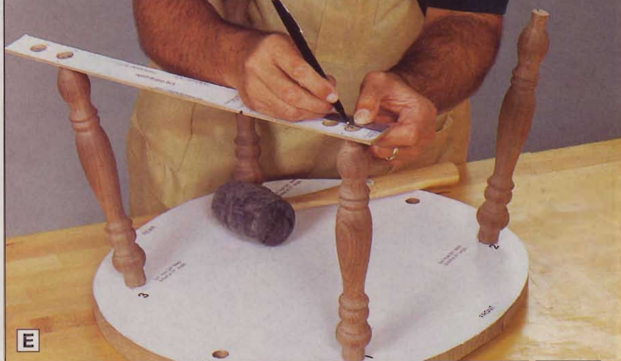
E Place the guide over the bottom ends of the legs and make alignment marks for the drilling operation.
