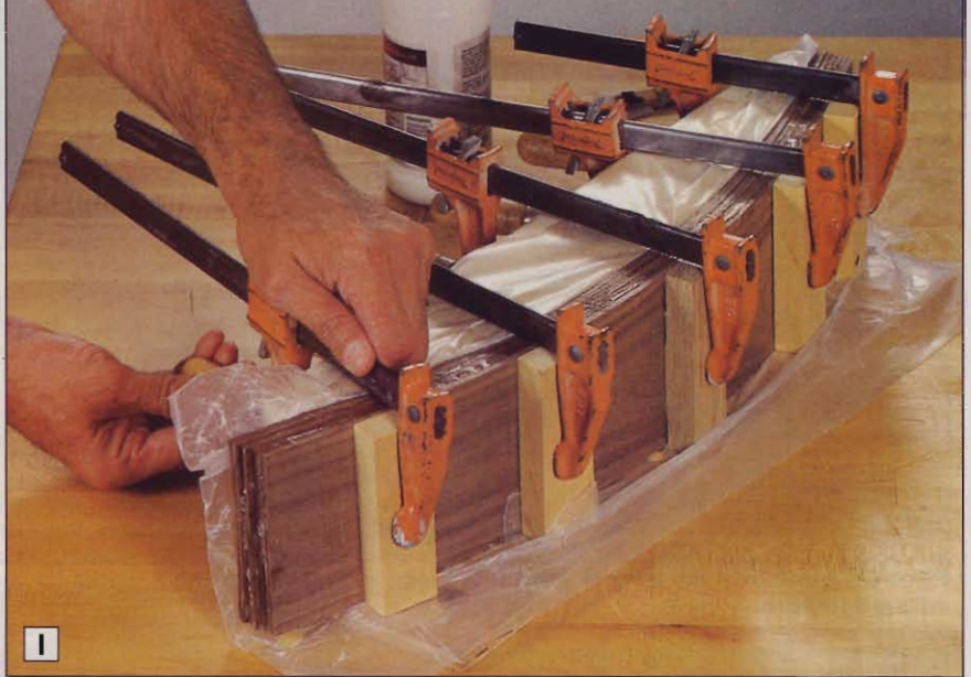
I Using white woodworker's glue, glue and clamp the \frac{1}{8} " pieces to the form and let the glue-up sit overnight.
