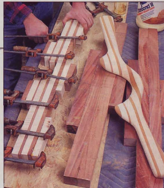
A canoe's carrying yoke begins as a lamination of mahogany and bird's-eye maple. It's then cut out at a bandsaw and shaped with a grinder.
