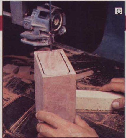
Hold the block firmly on the table with one hand and use a pushstick to guide the portion of the block near the blade.
