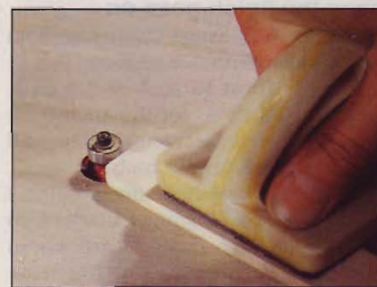
A secured zero-clearance table overlay and pad-style pushblock facilitate routing round-overs on the side panels.
