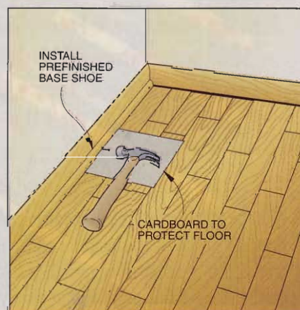
FIGURE 6 Finally, nail on matching shoe moldings to cover the gaps around the edges.
