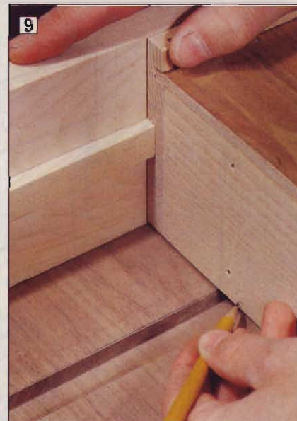
9 During assembly, turn the tabletop and base upside down and mark the stop locations on the back of the drawer.
