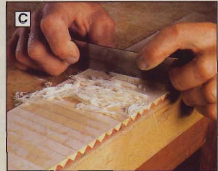
C After unclamping the log of banding, remove masking tape residue and glue squeeze-out with a hand plane, sanding block, or cabinet scraper (shown).
