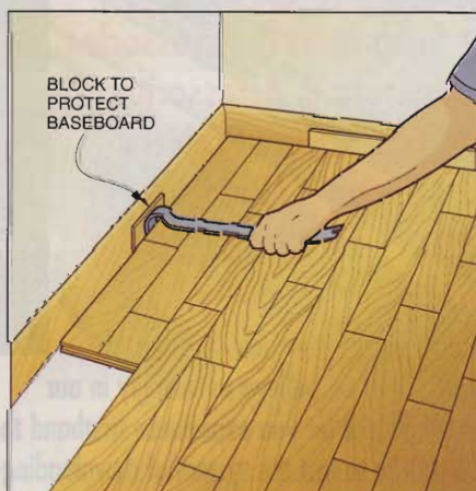
FIGURE 5 Apply glue and use a pry bar to snug up the first and last planks, as shown.
