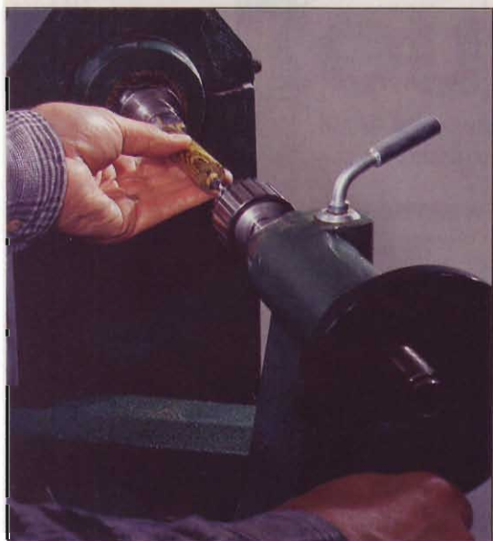
Turn the tailstock handle slowly and steadily to advance the drill into the wood. Run the lathe at a slow speed.
