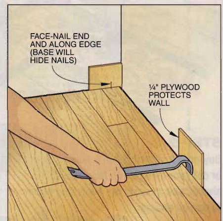
FIGURE 6 Push the last course tight with a pry bar, face-nail it, and cover the nails with putty.
