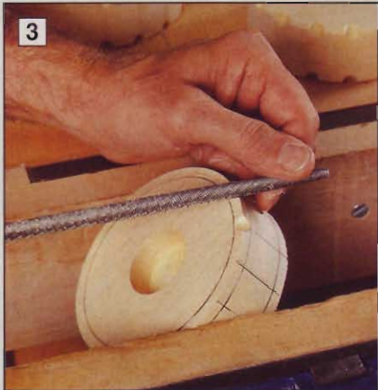
3 Guidelines show how deep to file with the round rasp when notching the tires.
