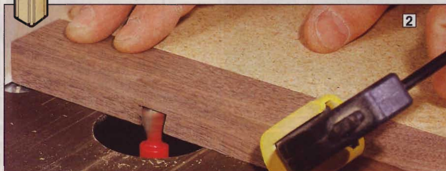
2 Clamp a follower block to the base rails to guide the dovetail cut and to prevent tearout when the bit exits.
