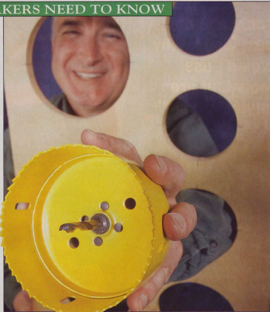
A large holesaw is one way to make holes big enough to reach through.
