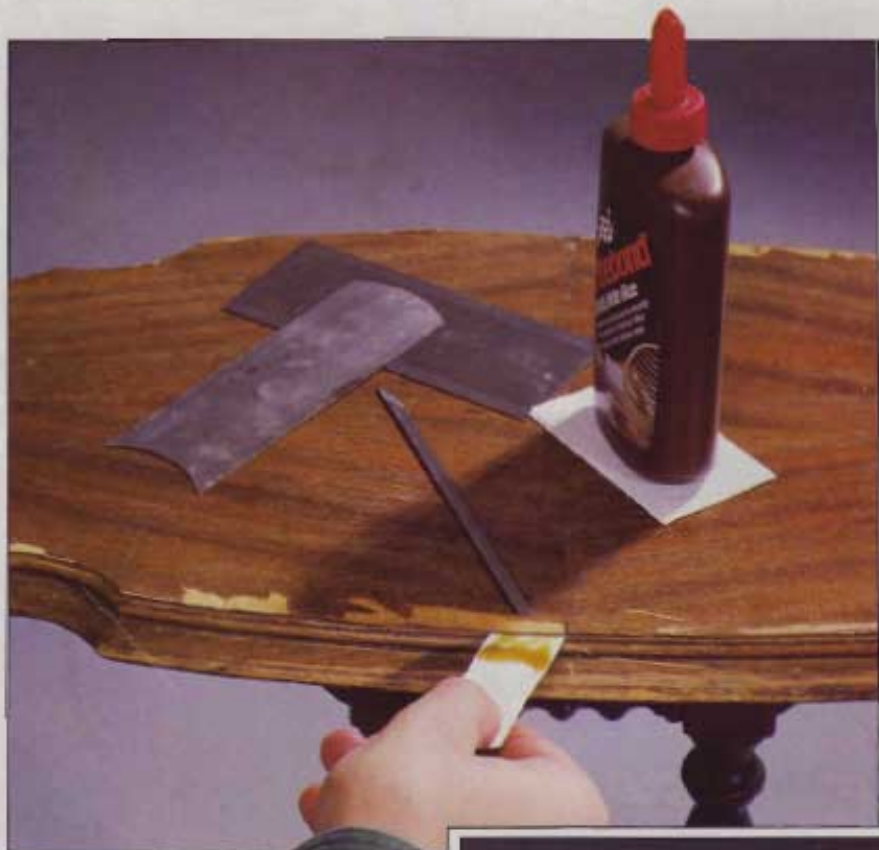
Chipped veneer is only part of the damage to this table edge. The layer between the tabletop and the finish veneer has come unglued, too.
