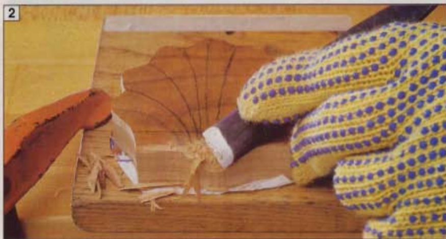
2 After roughing out the curvature with a gouge, you can smooth the contour by carving with the inside of a gouge, such as the 20 mm no. 3 shown. (The wing end of the shell is shown here.)
