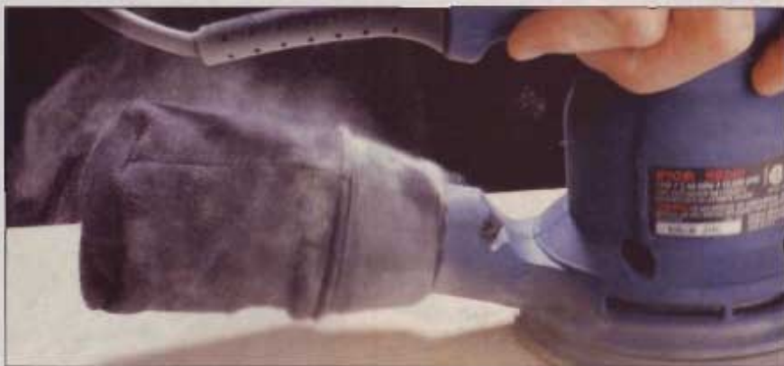
The Ryobi RS240 was one of two random-orbit sanders that blew clouds of dust through their bags.
