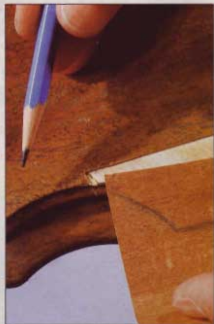
Fit the replacement veneer to the routed area. Trim it to rough width before gluing it in place.
