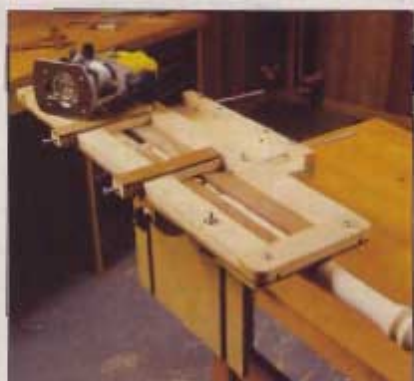
Creating mortises in workpieces goes quickly and precisely with this jig setup.
