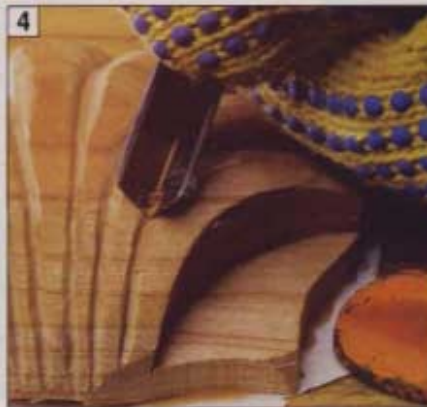
4 Carve the lobe lines with a V-tool, then round over the sides of the lobes to separate them. The wings have been cut to about ¼" thick.
