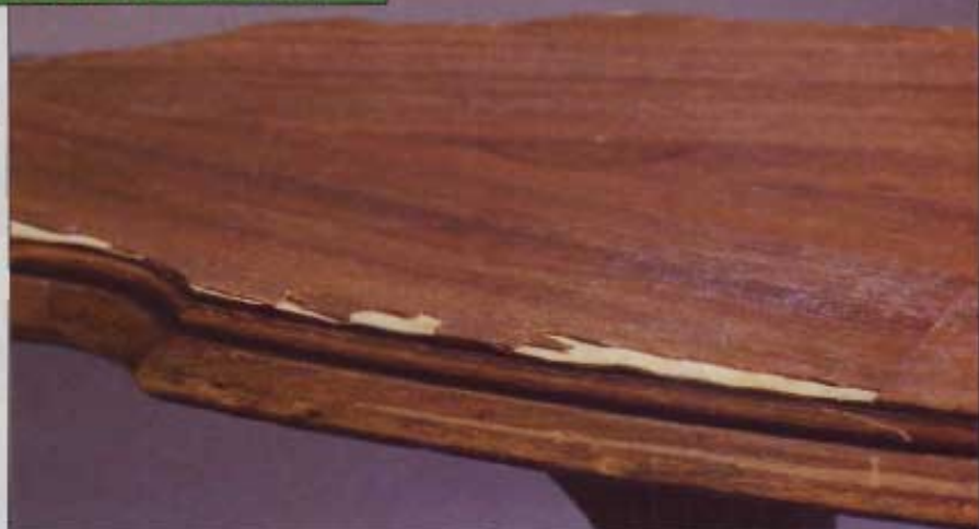
Chipped veneer is only part of the damage to this table edge. The layer between the tabletop and the finish veneer has come unglued, too.
