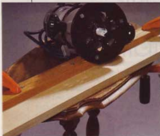
A simple guide and a router fitted with a straight bit make it easy to cut the old veneer back to a clean, straight edge.
