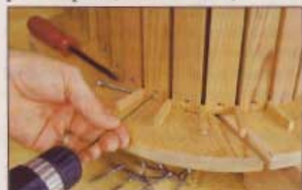
A length of coat-hanger wire, or other stiff wire, serves as a drill bit to reach past the panel edge.
