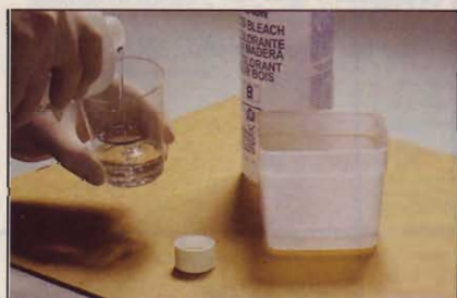
Work fast after mixing the two chemicals. The solution begins to neutralize—and lose bleaching power—just as soon as you start to pour the liquids together.
