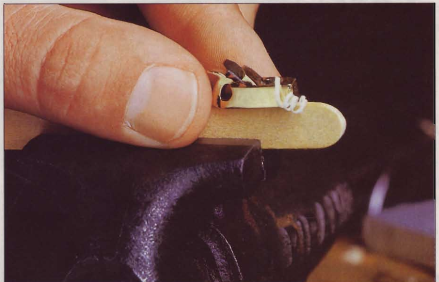
To make the blade of his tiny Sandusky coffin plane, shown here on a Popsicle stick, Hamler cut and honed a small section of a hobby-knife blade.
