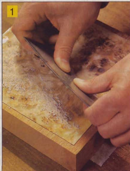
1 Scrape the veneer smooth after allowing the glue to dry. That's olive ash burl veneer on this Honduras mahogany blank.
