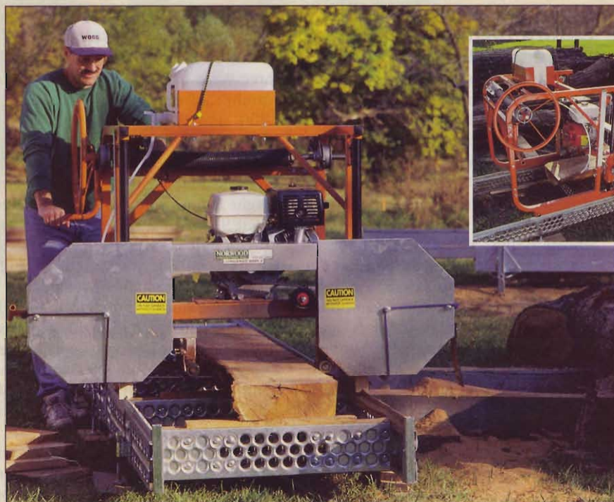
The Norwood Lumbermate must be pushed and pulled manually through the log during the sawing operation. The sawmill ships unassembled.
