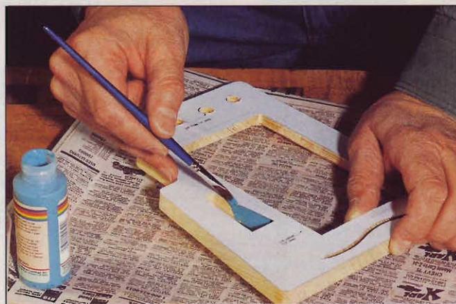
The paper pattern masks each frame front while you are painting the design cutouts.
