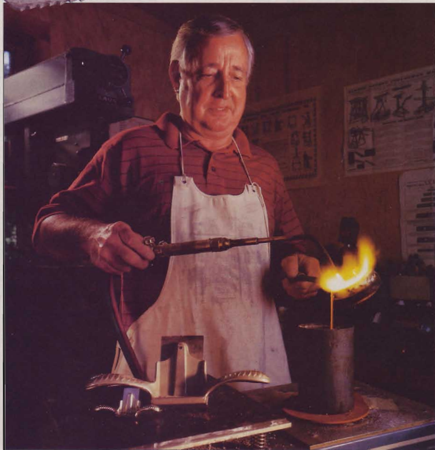
Toolmaker Paul Hamler casts brass for another miniature in his Snellville, Georgia, shop. Shown in the foreground are his full-size and 1/3-scale reproductions of a Stanley #81 scraper.
