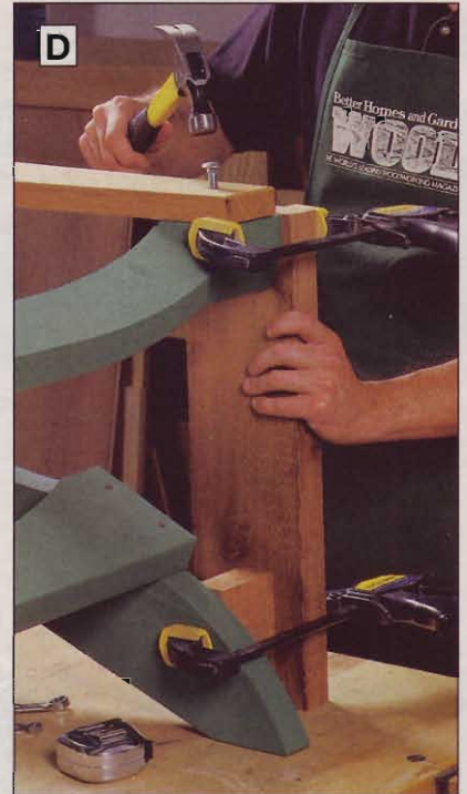
Clamp temporary support legs at each end of the frame to position the seat back support and connecting chair parts.
