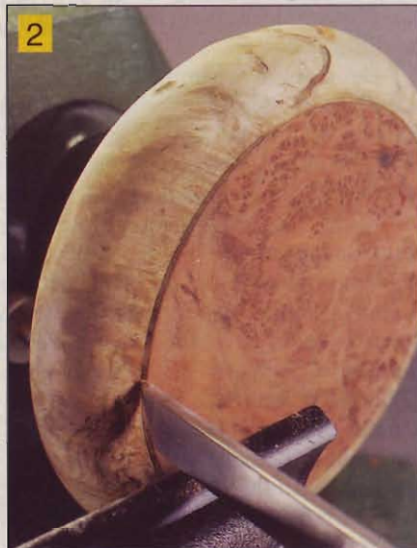
2 Define the veneer panel on front as you shape the edge. This turning features beautiful redwood burl veneer on a big leaf maple burl blank.
