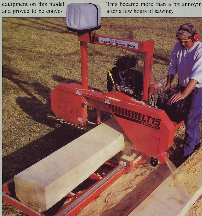
With the Wood-Mizer LT15, as with all bandsaw mills, you must first square the log into a cant before you can saw boards.
