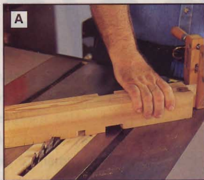
A Align the marked dados with your dado blade. Use a clamp as a stop on the miter-gauge extension for consistently placed cuts.
