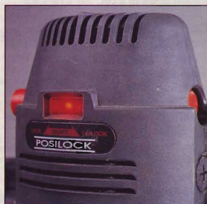
On the Craftsman 27511, snapping the red actuator to the left locks the spindle. The indicator light shows that the spindle is locked, and an internal switch cuts power to the motor until you disengage the lock.
