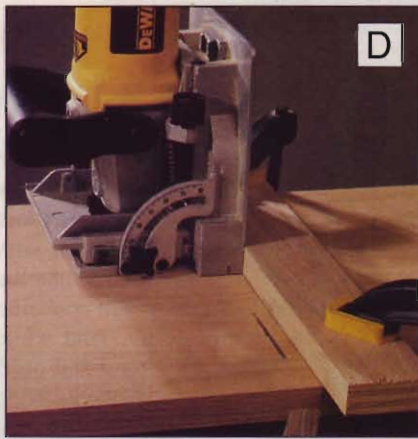
A straightedge clamped to the cabinet's sides accurately aligns slots for the biscuits that will attach the waist trim.
