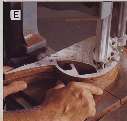
E Make the final cut to free the lid as a smooth continuation of the curve that comes down the top of the tail.
