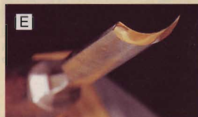
Polishing smooths the bevel for easier cutting and to leave a burnished surface, free of scratches, in the cut.
