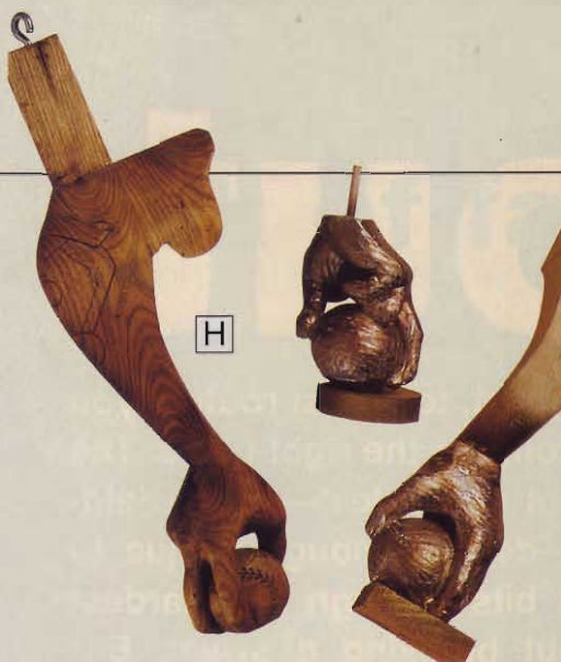
Keith used a life-casting of a hand holding a baseball (center) to mock up a table leg (right) prior to carving a prototype leg (left).
