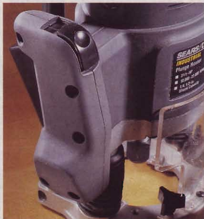
Lock the Craftsman 27511's plunge depth by pulling the handle-mounted trigger. To release the mechanism, simply push the button on top of the handle.
