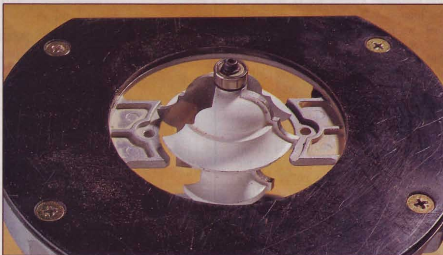
The guide-bushing mounting tabs on the Hitachi M12V effectively narrowed the base opening enough that we couldn't fit the widest part of a multiple-profile bit through.
