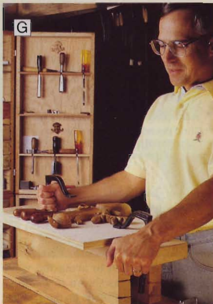
G Scrapwood risers bring the working surface of an ordinary woodworking bench up to elbow height, a better level for carving.
