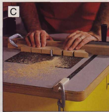
Stopblocks—one on the auxiliary fence and the other in the miter-gauge slot—let you control the location and depth of the waist trim notches.
