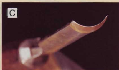
Grind the edge until the reflection is about the width of a pencil line before beginning to hone the edge.
