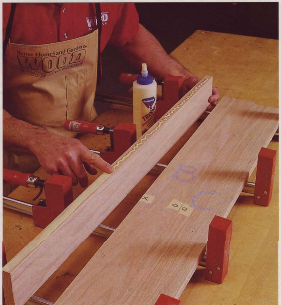
Apply a bead of yellow glue on just one board per joint, and spread it evenly with your finger. All it takes is enough to coat the surface. Anything more gets squeezed out.
