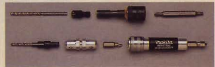
Jack Rabbit (top) parts, left to right: drill bit, countersink/collet, sleeve, driver bit. Flipper parts, left to right: drill bit/countersink, insert, driver bit, holder.
