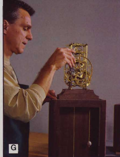
G The removable upper case makes mounting and adjusting the movement easy.
