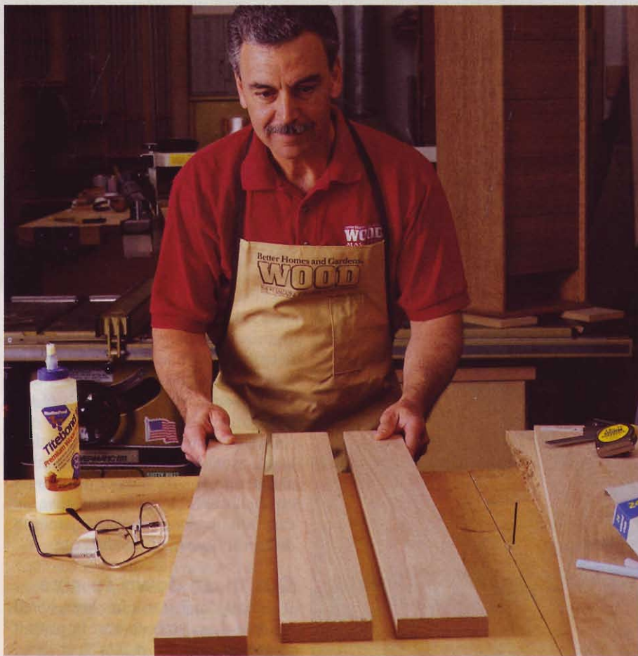
After cutting your stock to size, lay the boards on your workbench and begin looking for the perfect match, as WOOD magazine's contributing craftsman Jim Heavey does here.
