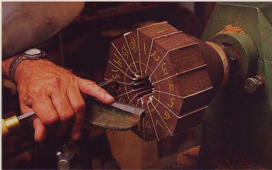
Chucked onto his 5-speed Woodfast lathe, the segmented ring presents solid end grain to Galen's turning tool.
