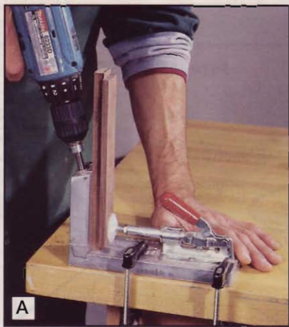
A Use a pocket-hole jig to drill the inside faces of the rabbeted rails.
