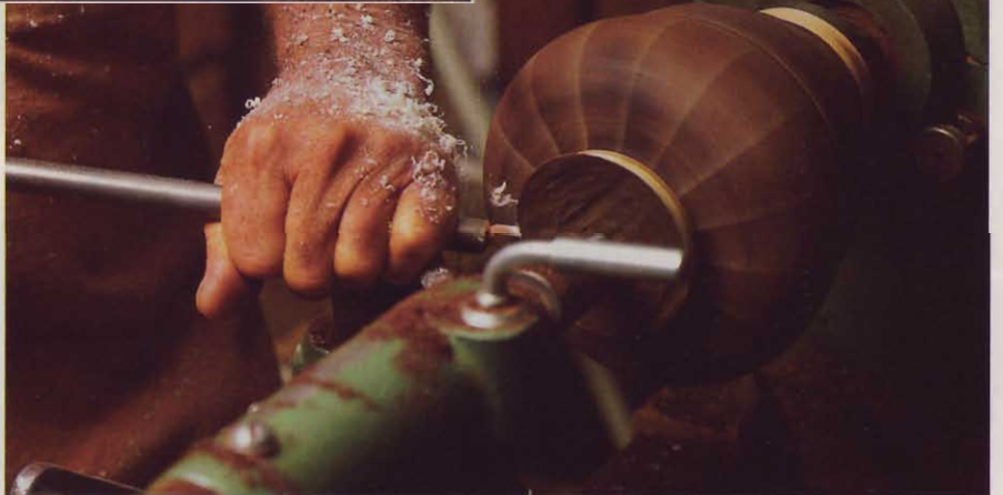
"The high-speed steel cutting tip actually shears the end grain, although it looks as if I'm scraping because there are no long curls," says Galen.
