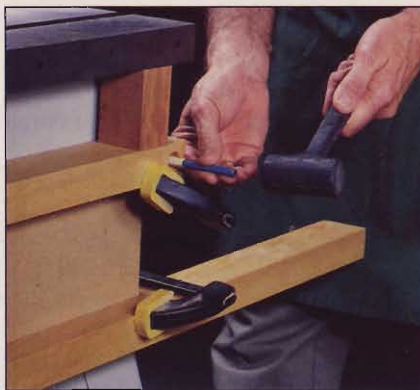
Position the rails with spacers, clamp the rails to the table, and transfer the 3/8" hole locations using a center punch.
