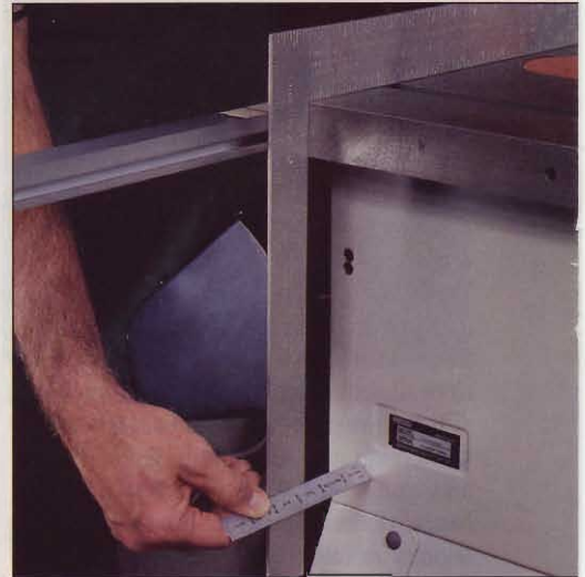
Use a framing square held tight against the table edge, along with a rule, to determine the width of the rails (E, F).
