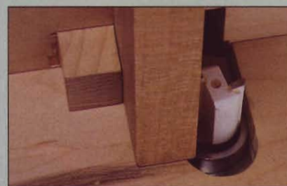
The bit-to-guide-pin distance should exactly match a \frac{3}{4} "-thick piece of scrap.
