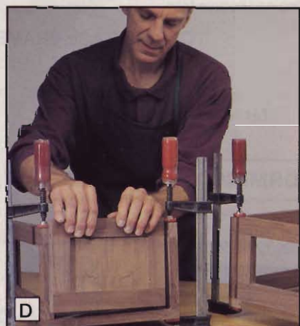
D Check the fit of the upper case top frame in the upper case and the fit of the lower case top frame in the lower case.
