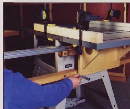
Clamp the sliding table flush with the saw top, and measure for the thickness of the wear blocks and their spacers.
