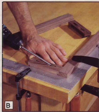
B A square keeps the edge of the rail flush with the end of the stile during assembly.
