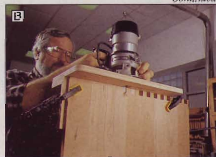
Use the jig to rout the notches in the ends of the back panel.
