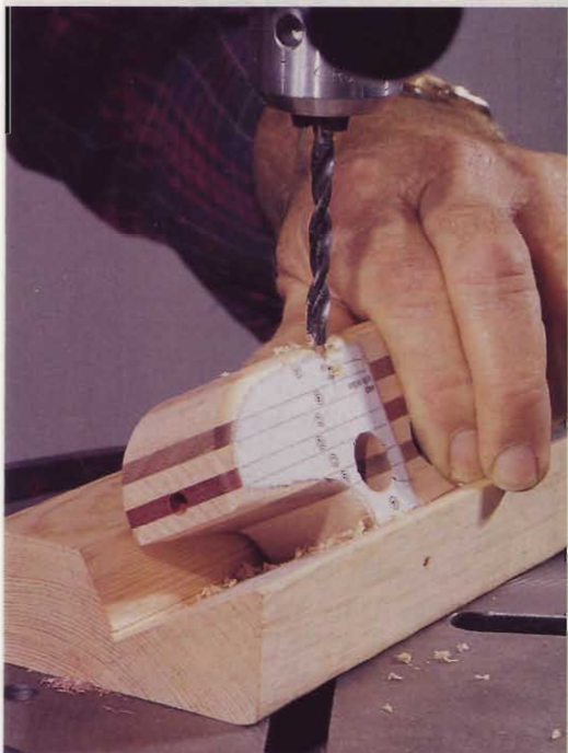
Use the drilling jig to bore the angled pontoon-strut holes (shown here) and wing-strut holes.
