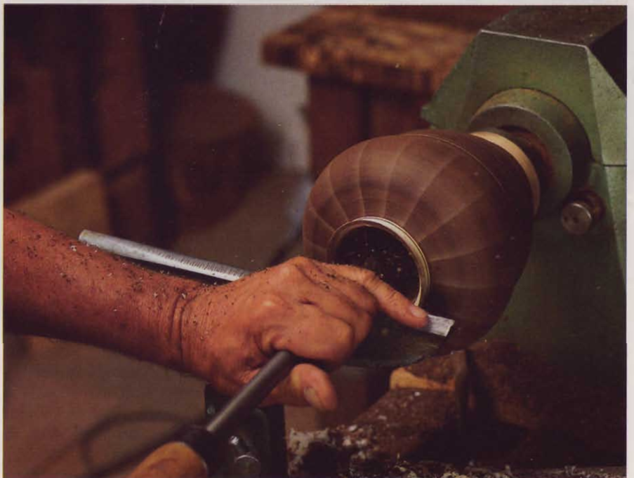
With the outside of the bowl turned to shape, Galen turns his attention to the inside with a Thompson hollowing tool. After the bowl has been finely sanded, he'll finish it with three or four coats of Waterlox, a tung-oil based clear finish.
