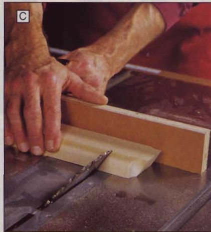
Form the pilot bumper (G) from a long blank, then cut it to length.
