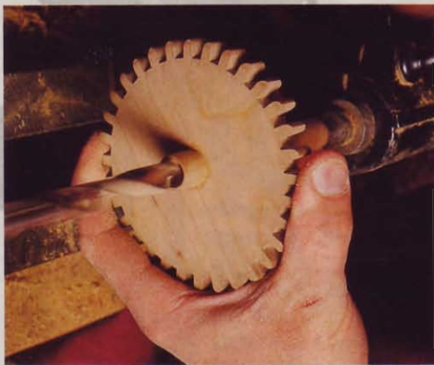
At the lathe, Jim drills out a dowel that the hand shaft will pass through. He prefers iron-wood for those parts.
