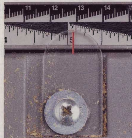
Some of the tapered increment markings on the Ridgid TS2424's rip scale don't reach the cursor.
