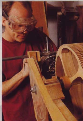
A router mounted on a sliding track cuts the teeth for gear wheels. The fixture will take a wheel up to 8' in diameter.
