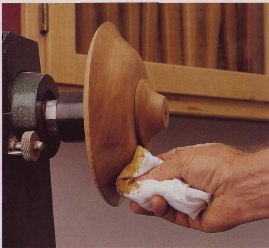
Finish the outside of the bowl on the lathe before reversing it on the chuck to turn the inside.
