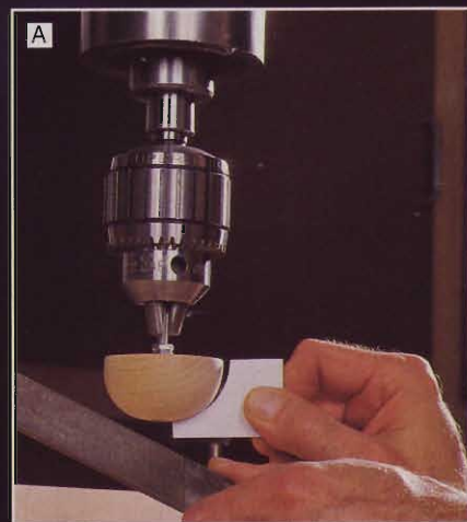
As you form the nose (C), check your progress with the template.
