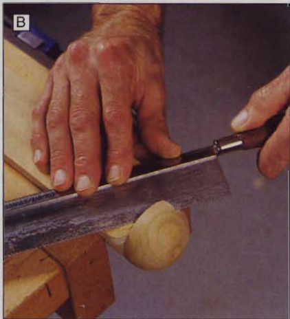
Use a handsaw to trim the nose (C) flush with the bottom of the running board.
