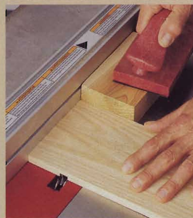
To prevent tearout when making a dado cut, back your workpiece with a scrap softwood follower block.
