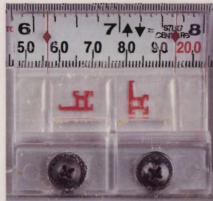
Dual cursors keep Delta's scale accurate regardless of the fence orientation. But from some viewing angles, we couldn't tell one increment marking from another.
