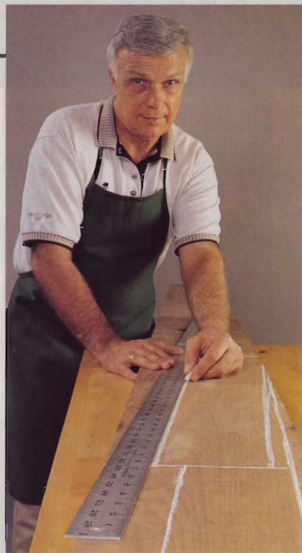
For the best grain match, Chuck Hedlund often cuts workpieces at a skewed angle to the board edge.
