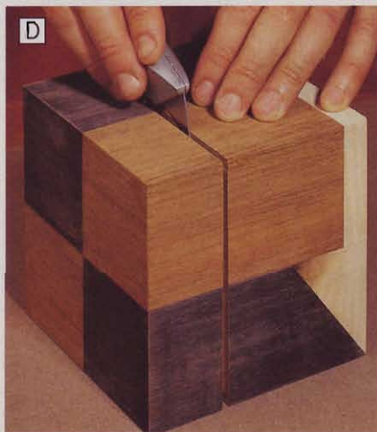
Carefully slice through the last \frac{1}{2} " by cutting down the center of the saw kerf with a utility knife.
