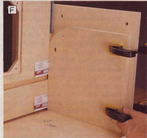
F Clamp the guides to the sides, inserting business cards for working clearance.
