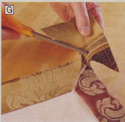
G Miter-cut the fabric at the back-panel corners, and leave enough material to fold over the point of the corner.
