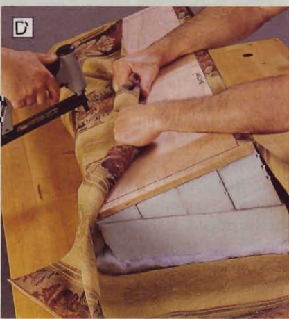
D Enlist the help of a friend to pull the fabric uniformly taut along the length of the cushion as you staple the fabric.
