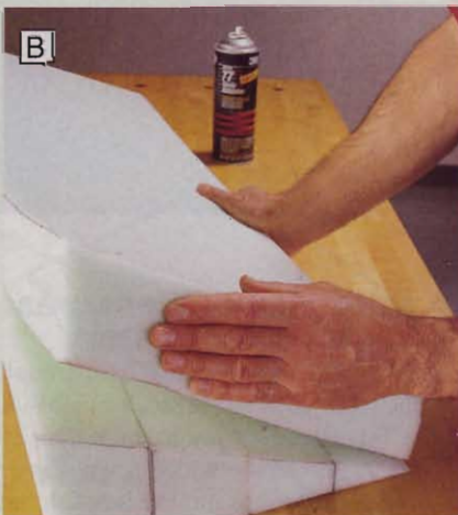
B Align and adhere the front piece of the seat back to the glued-up rear pieces.
