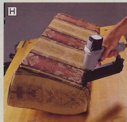
H Brads hold the upholstered back panel to the upholstered cushion panel. The brad heads disappear below the fabric.
