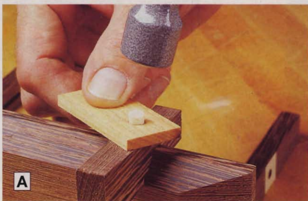
A Use a \frac{3}{16} "-thick strip of wood with a \frac{5}{16} " hole to gauge the projection of the dowels.
