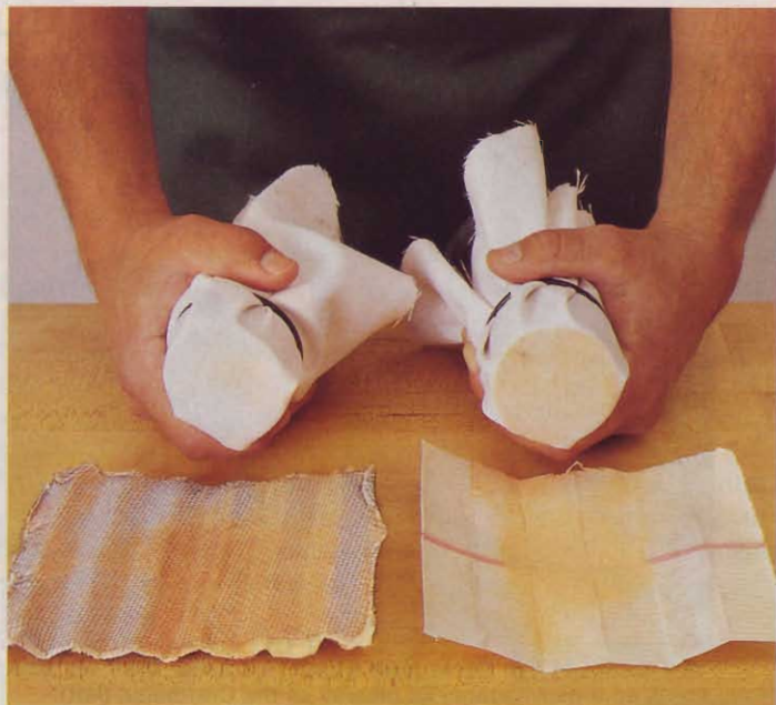
Fewer chalk-dust particles escaped Genie's HEPA filter (left) than Craftsman's pleated-paper filter (right).
