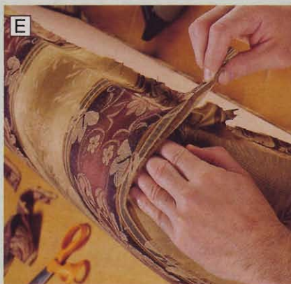
E Use one hand to tuck the excess side fabric under the top or bottom fabric. Staple down and trim the extra material.
