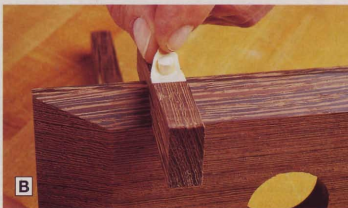
B When you remove the tape, the glue that squeezed out when you inserted the dowels comes off with it.
