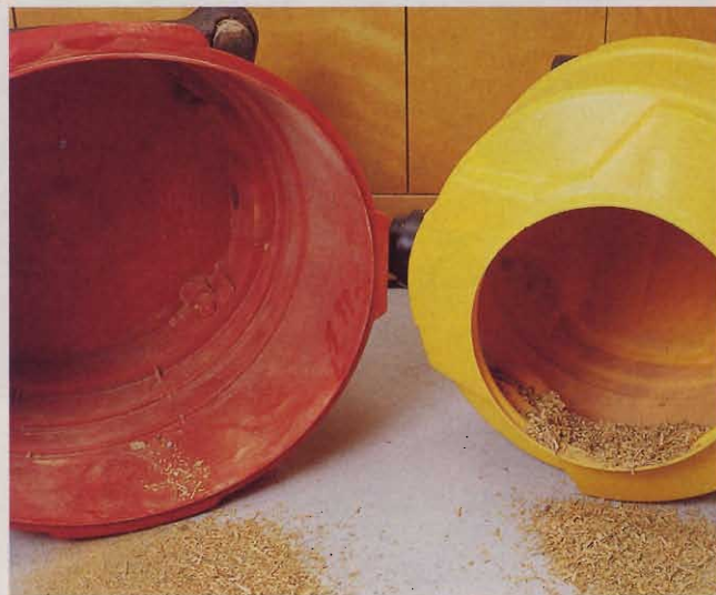
The mouth of the Genie tank (right) is smaller than the tank itself, so it didn't empty as cleanly as the Craftsman (left).
